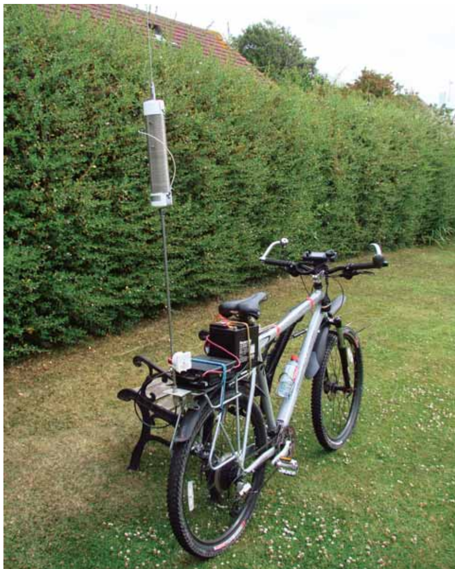
PHOTO 1: The G3LDO bike mobile with the IC-707 Mk2, which provided 10W of RF for the tests. The antenna shown is a cut-down version of the Texas BugCatcher antenna, which was used as a reference. The RF current meter can be seen at the base of the antenna.
