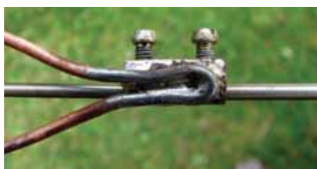
PHOTO 4: Method of adding 14SWG copper wire top loading to an existing stainless steel stinger.
