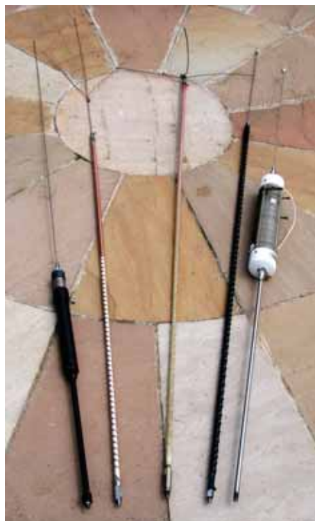
PHOTO 2: (r-l) a cut down Texas BugCatcher; helically wound commercial mobile of unknown pedigree; a modified CB FireStik, another unknown commercial helical; and an MP-1 portable manual 'screwdriver' antenna.
