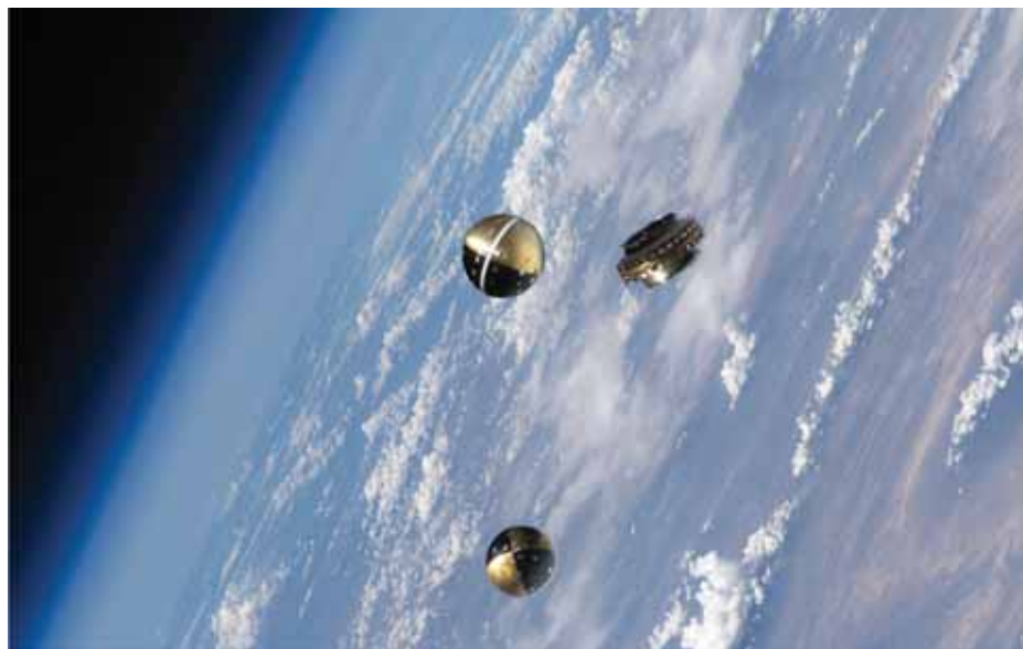
PHOTO 1: Castor and Pollux shortly after deployment, photographed from the Space Shuttle and seen with a discarded coupling ring. Photo: NASA.
