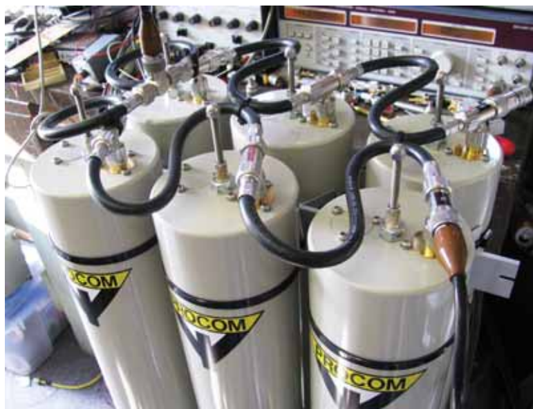
PHOTO 1: DPF2/33 2m band 6 cavity duplexer.
