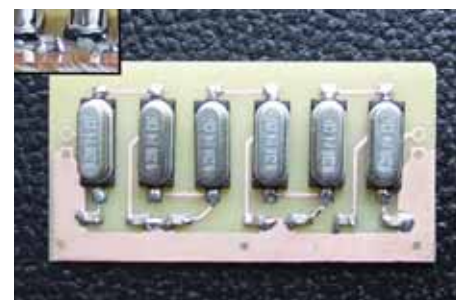
PHOTO 3: The completed SMT filter.
