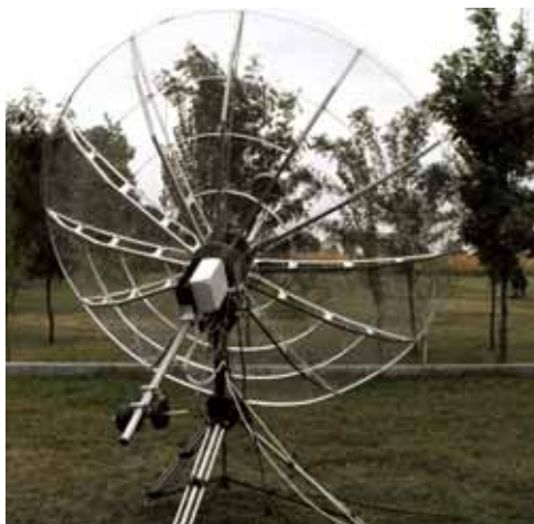
PHOTO 3: OK1DFC's 3.2m commercially available dish set up for an EME expedition. (Photo: OK1DFC).
