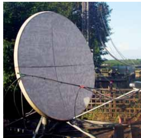
PHOTO 2: Prodelin 2.4m VSAT antenna belonging to GW4DGU. This is used on 10GHz. (Photo: GW4DGU).
