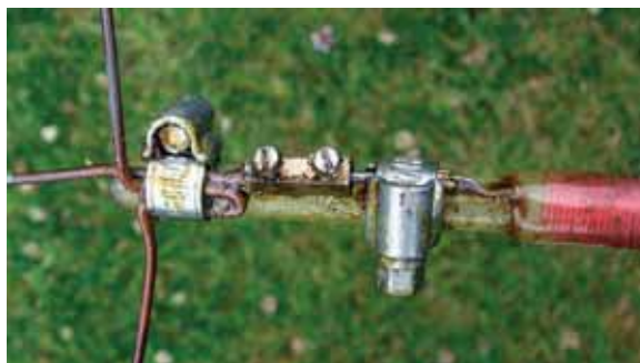
PHOTO 3: The top portion of the CB FireStik antenna, showing the method of fixing 14SWG copper wire top loading.
