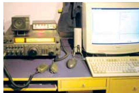
PHOTO 2: The shack at G4HPE. The Gateway interface sits on top of the HF transceiver with the VoIP computer to the right.
