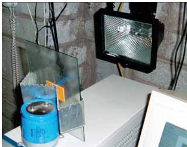
PHOTO 2: My not-so-high-tech PCB exposure system.
