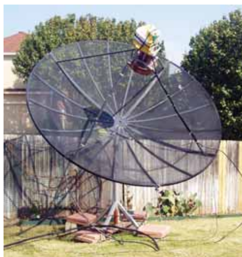
PHOTO 1: 3.1m TVRO dish used by WW2R (Dallas) on 902MHz to 3400MHz EME. (Photo: WW2R).
