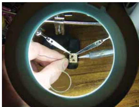
PHOTO 5: Soldering surface mount devices is often more easily accomplished with the aid of a strong magnifying glass.
