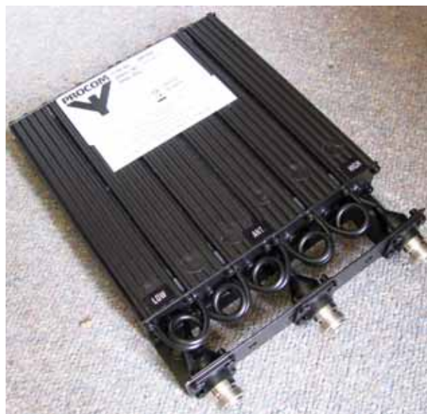
PHOTO 2: DPF70/6 70cm band 6 cavity duplexer.
