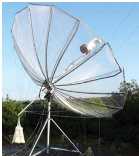
PHOTO 4: Home built 3.2m stressed construction dish belonging to DL1YMK and used on 432 – 3400MHz EME. (Photo: DL1YMK).
