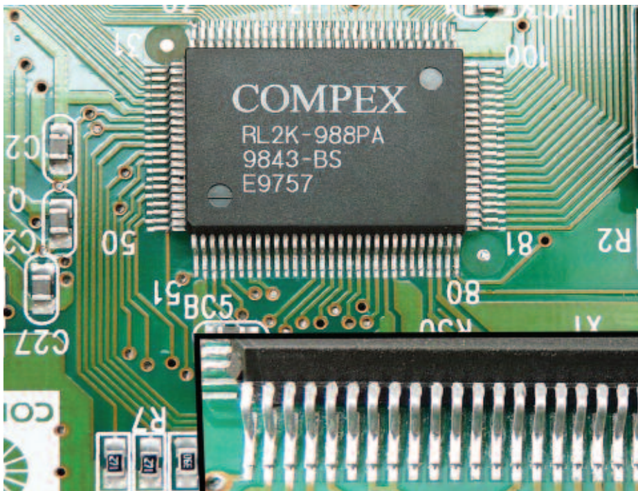
PHOTO 3: You'd never know it, but this 100 pin IC has been removed & replaced in an amateur workshop. Excess flux was cleaned off after the operation.
