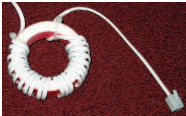
PHOTO 2: Many turns on a 58mm ferrite toroid are needed to keep top band out of the ADSL router.
