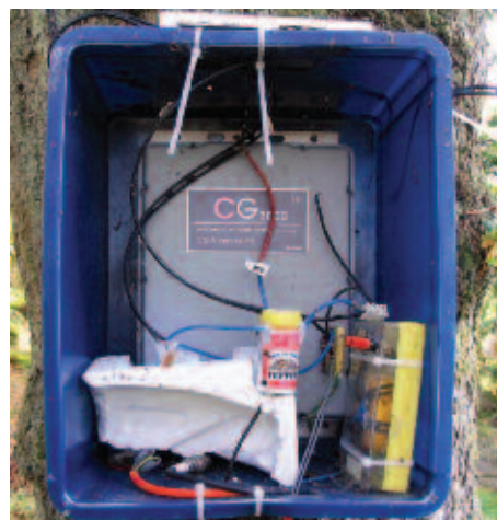
PHOTO 5: The ATU in its tree-mounted box with the lid removed. The aerial relay is inside the pepper carton.
