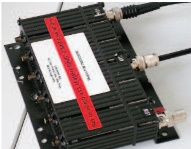
PHOTO 1: A typical duplexer filter: Thales MPX2/6H-6/16 six cavity device.
