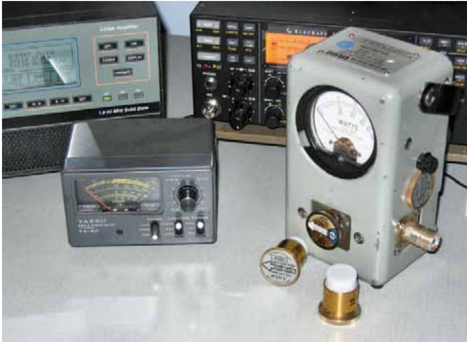
Two free-standing VSWR meters, with two more built into the equipment behind.
