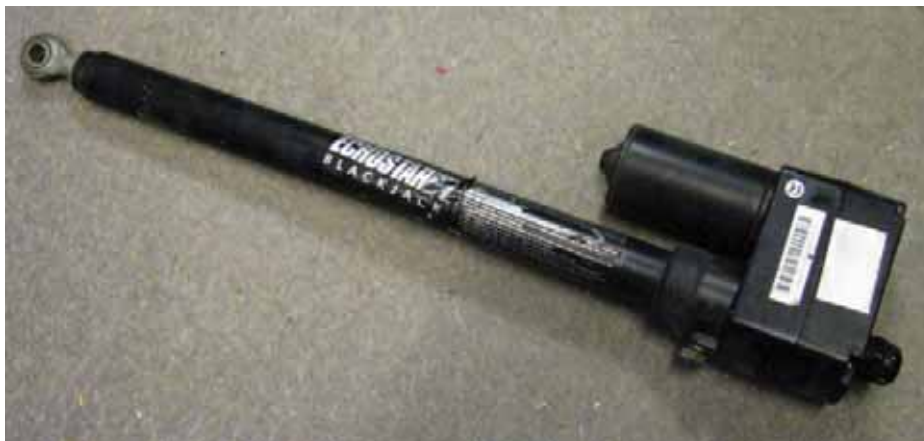
PHOTO 2: A typical linear jack as used for satellite TV positioning systems.
