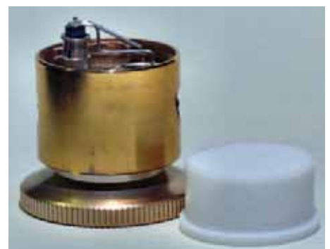
PHOTO 1: The pickup loop inside a Bird wattmeter element (like Figure 1d).
