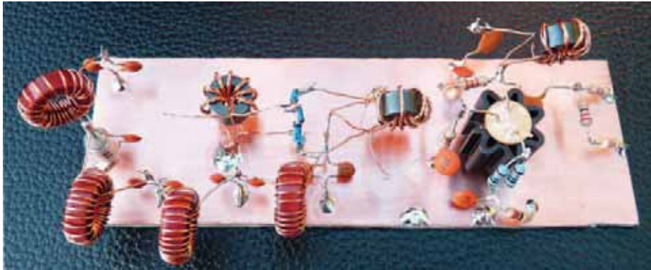
PHOTO 1: The front end of the LF receiver is a conventional low pass filter, mixer and buffer amp – see Figure 3.
