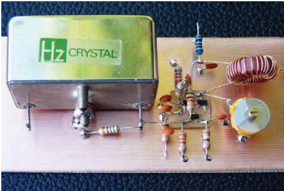
PHOTO 2: One IF amplifier, with the crystal filter on the left.
