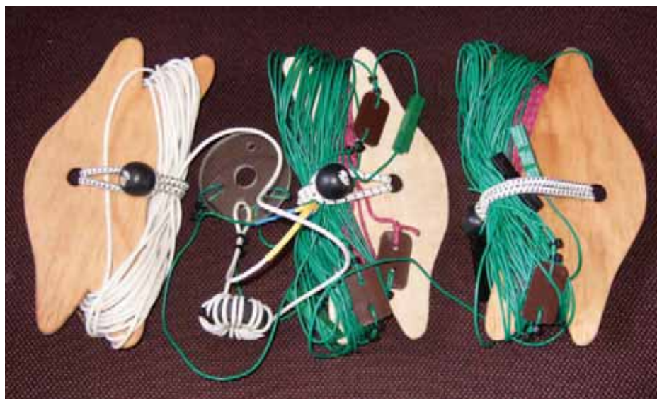
Linked dipoles. GW4BVE started using single pole PowerPole connectors in the links but has now moved on to using 2mm gold connectors as used by radio control modellers. The whole antenna including feeder and carry bag weighs 580g. Photo courtesy GW4BVE.
