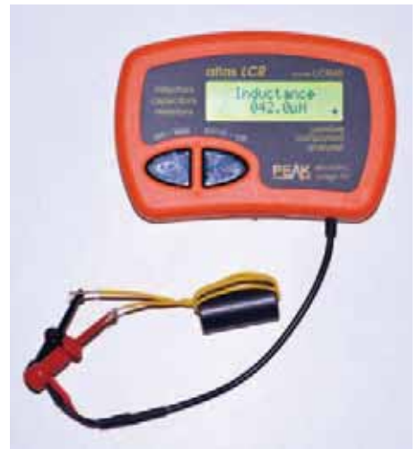
PHOTO 2: Measuring the inductance of a coil wound on ferrite.
