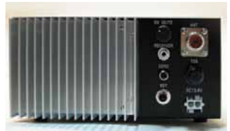
Simplicity is the keyword on the rear panel, dominated by a large heatsink.
