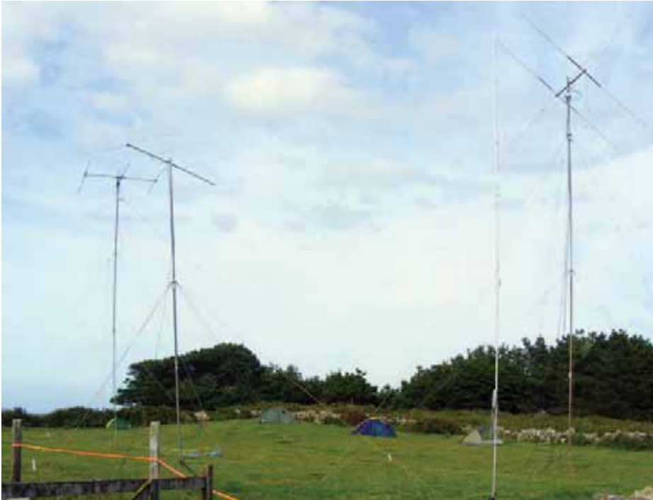
M8C antennas, with the sea-path to the east just beyond. Several team members camped in the field. L to R: TET tribander up 50ft, 6m Yagi, Butternut spotting antenna, 10/15m quad up 40ft.
