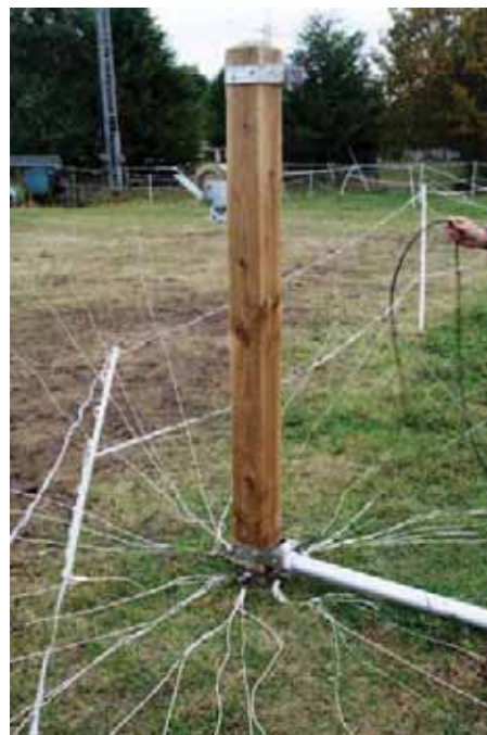
One of the 80m 4 square elements showing the radial system and lowered element.
