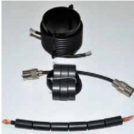
PHOTO 1: Balun types. Top: 8 turns of RG58 on a section of 70mm plastic pipe. Middle: 8 turns of RG58 through 6 ferrite rings. Bottom: 6 ferrite beads threaded on a length of Mini8 coax.
