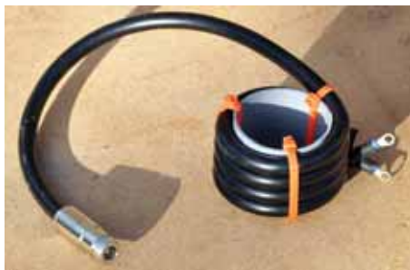
PHOTO 2: Coiled coax choke balun as supplied by Vine antennas.
