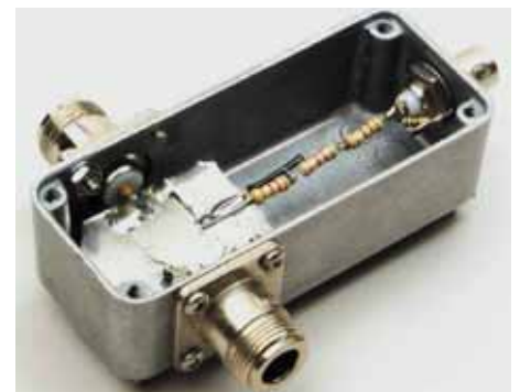
PHOTO 1: Practical construction of W7ZOL's 100W inline sampler (ARRL).
