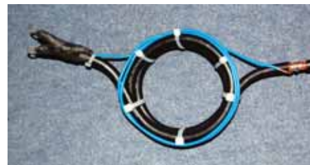
PHOTO 3: The GOKSC-recommended balun, described as a Grounded Pawsey Stub, from [3].
