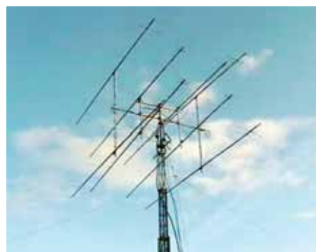
The 2m (4 x 12 ele M2) and 70cm (4 x 28 ele M2) arrays put up for EME.
