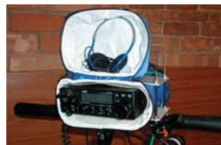
The Alinco DX-70 mounted in a weatherproof covering on the bike handlebars.
