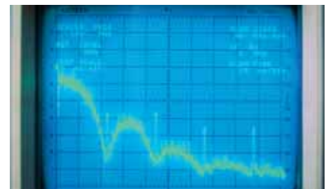
FIGURE 1: Truly random digital noise gives a SIN(X)/X shaped spectrum (ignore the spikes, which are from clock breakthrough).
