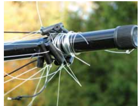
PHOTO 4: The fixing of the antenna elements.
