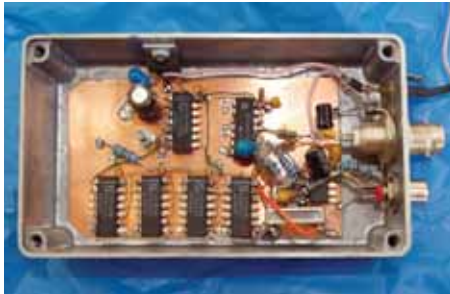
PHOTO 1: A pseudo noise generator like this can provide very good results at low frequencies.
