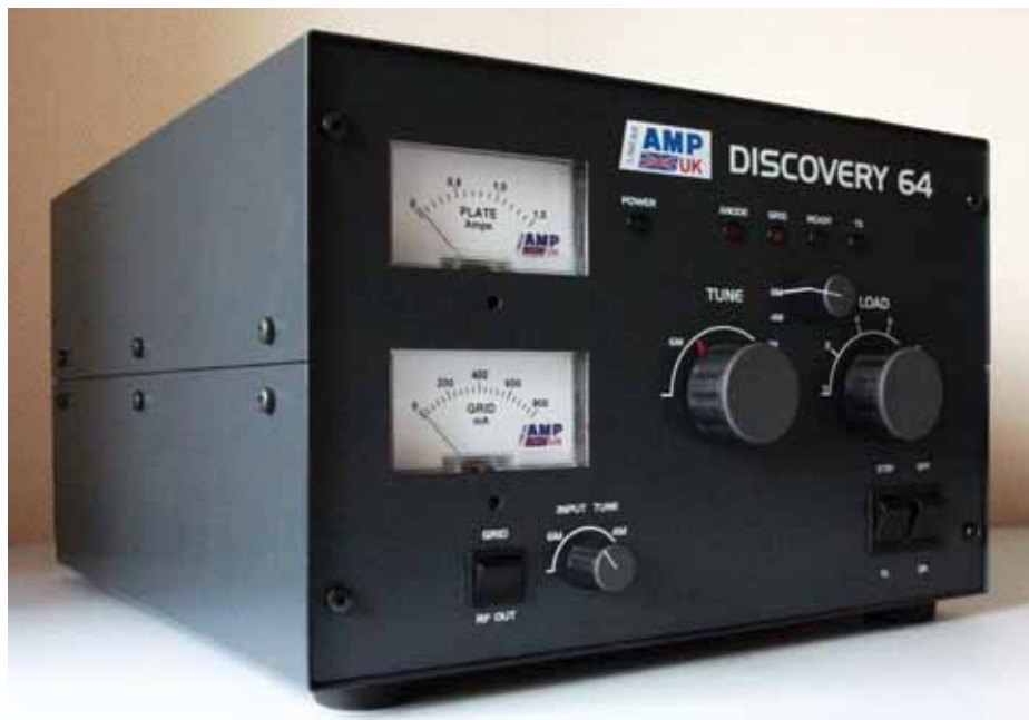
PHOTO 1: The Discovery 64 is a high power linear amplifier for 50 and 70MHz.
