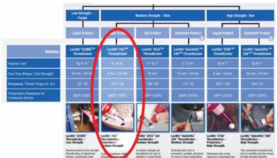
FIGURE 2: Selection chart identifies Loctite 243 for rotators and antennas. © Henkel Corporation (Loctite)
