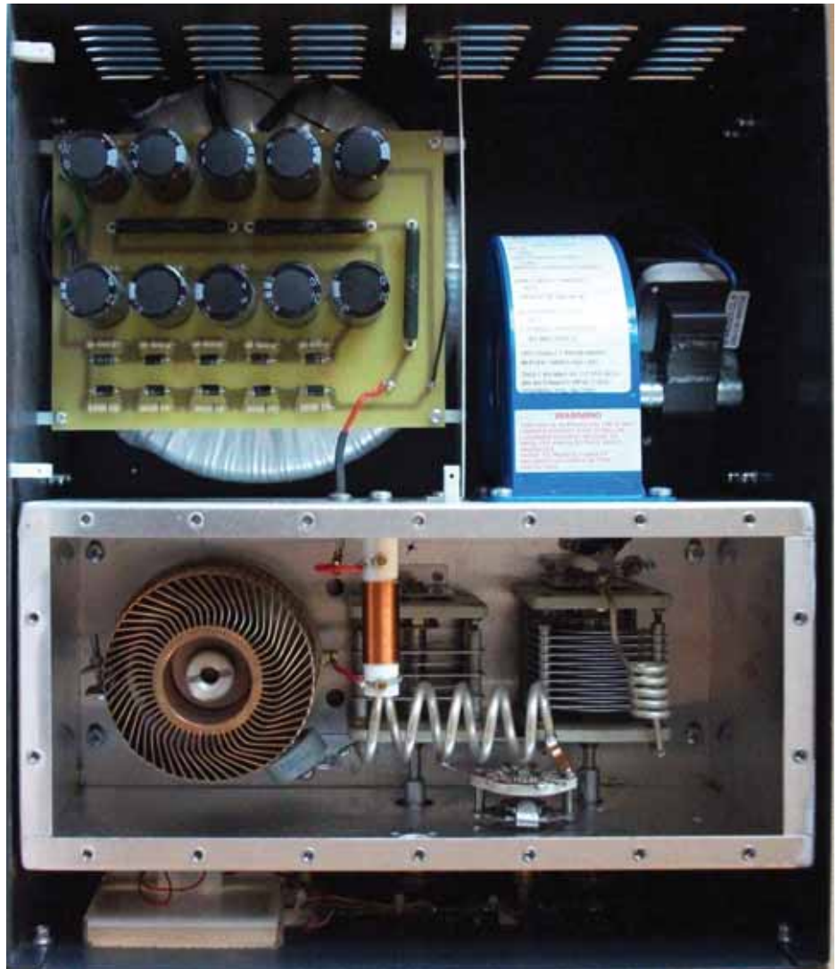
PHOTO 2: Taking the covers off revealed the PA circuitry.
