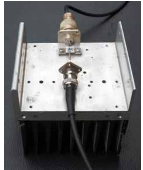
PHOTO 3: A home made 40dB high power attenuator.
