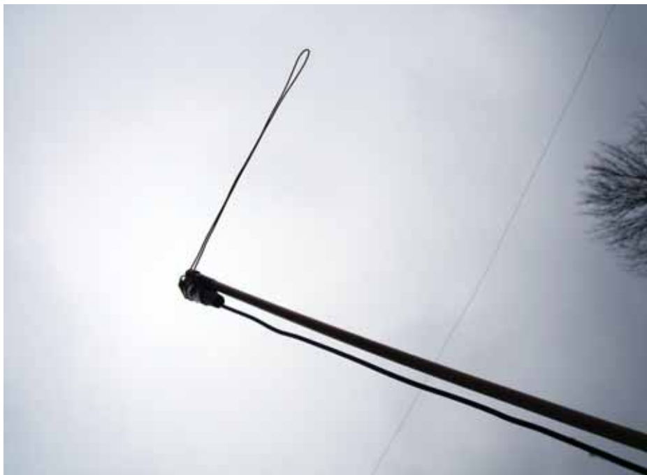
PHOTO 2: The G8MM loop mounted on a partially extended 10m fishing pole to get close to the telephone drop-wires. WARNING - Members should exercise caution when near to any overhead wires, first checking that they are insulated telephone drop wires and not overhead electric power wires.
