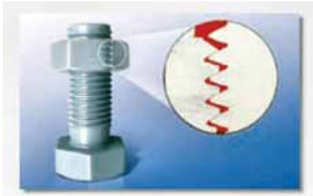
FIGURE 1: Gaps between threads are essential for assembly, but allow movement afterwards. © Henkel Corporation (Loctite).
