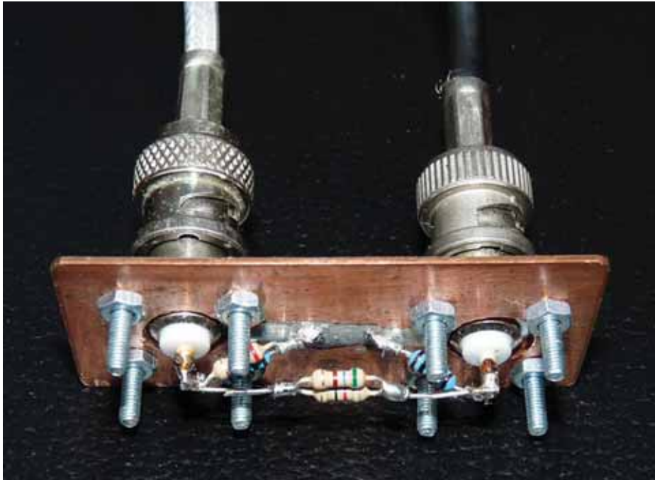
PHOTO 1: A home made 10dB attenuator.
