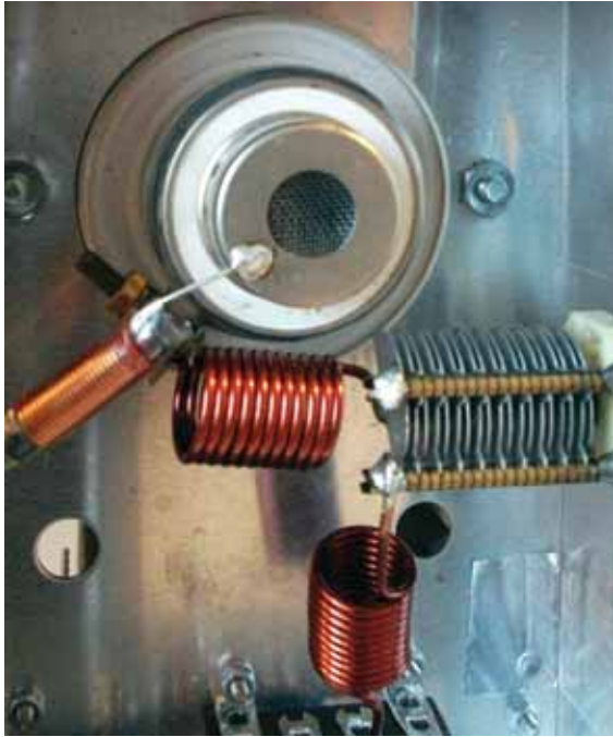
PHOTO 3: The cathode circuitry under the covers of the Discovery 64.
