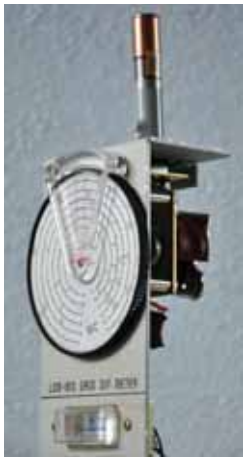
PHOTO 2: A FET GDO using the chassis, case, calibrated tuning mechanism and coils of a defunct LDM-810 nuvistor GDO.
