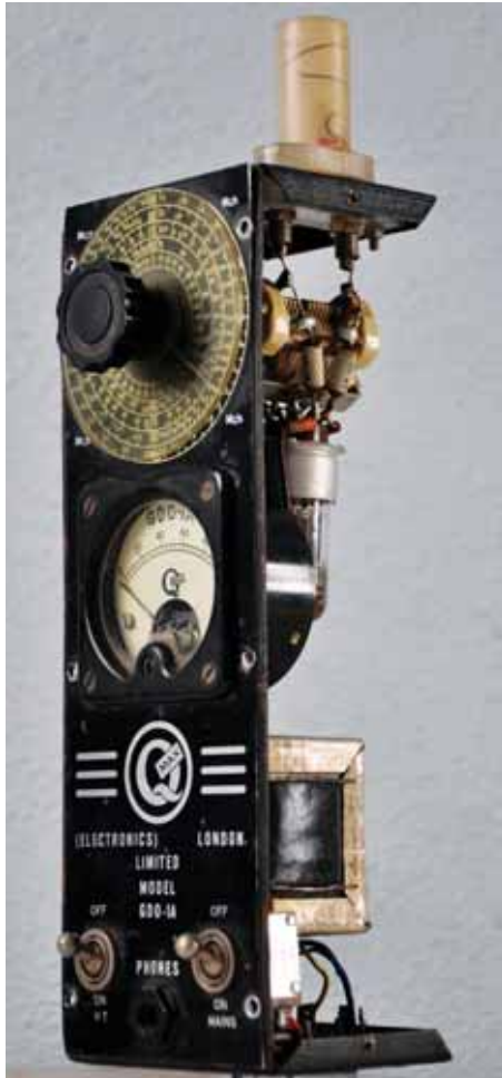
PHOTO 1: Q-Max GDO-1A uses a 12AT7 double triode, one half used as an oscillator and the other half as a half-wave rectifier.
