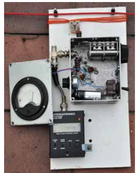
PHOTO 4: The antenna element resonance measuring kit. Note the method of maintaining a constant coupling to the antenna element (red wire) and the GDO coil.
