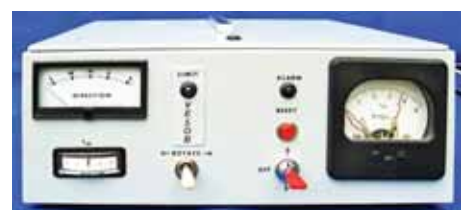
PHOTO 6: The control box. Rotator controls are on the left side.
