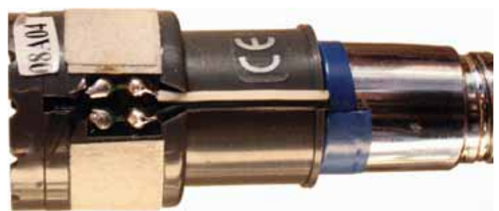
PHOTO 3: Detailed view of how the mic insert is mounted.
