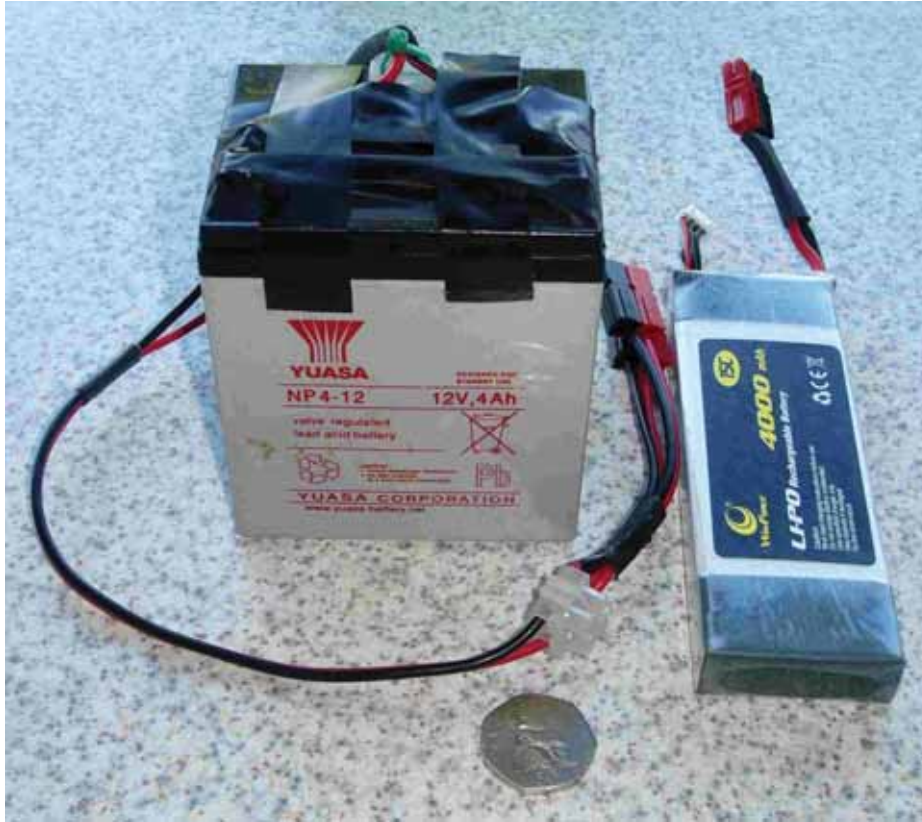
Lead-acid gel cell on left and equivalent LiPO battery on right.
