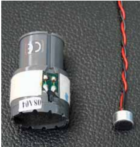
PHOTO 1: Typical dynamic microphone (left) and electret condenser mic (right). The electret mic is 9.8mm diameter.
