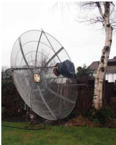
PHOTO 1: G4DZU 3m diameter EME dish with 23cm feed.
