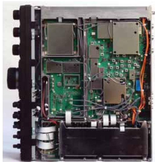
FTDX5000 underneath view with covers removed showing the main RF boards and synthesisers.
