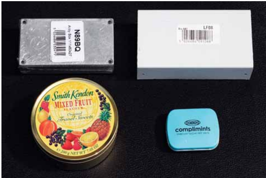
PHOTO 2: Small RF projects can be accommodated in and screened by commercial project boxes or re-purposed sweet tins.
