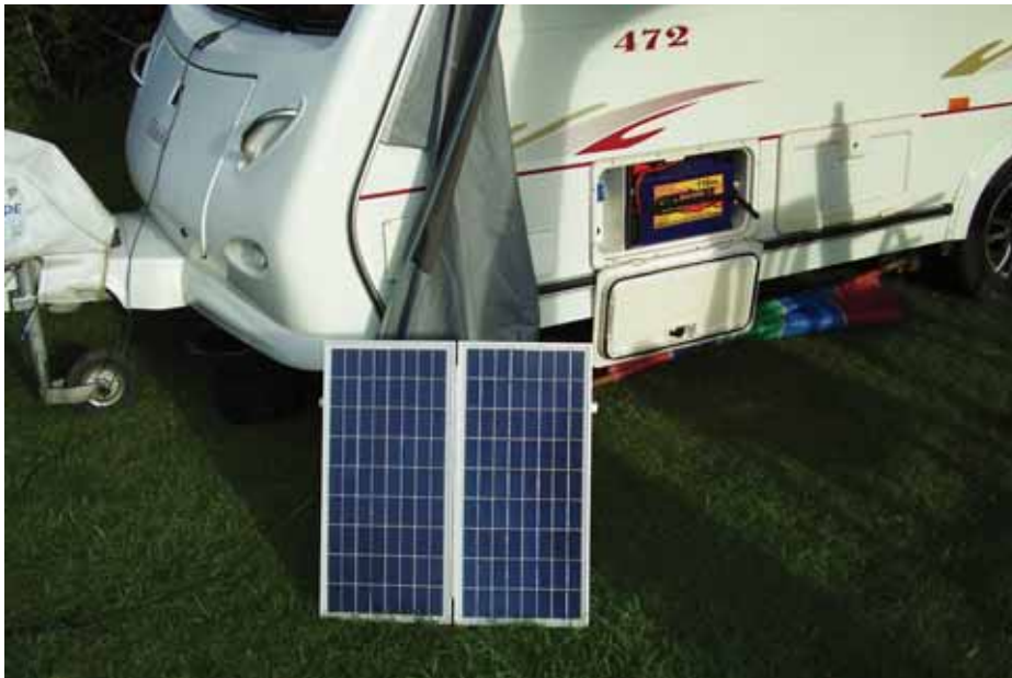
PHOTO 3: Roy, Goprk used twin 20W panels to charge a pair of 110AH batteries in his caravan.
