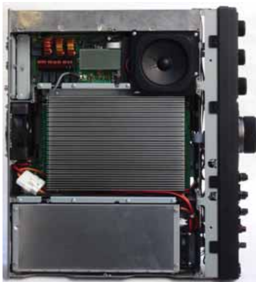
Top view with covers removed showing filters, TX PA and power supply.
