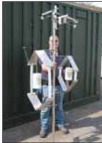
Mark, G8AWO showing off the assembled 10/15/20 & 40/80m Combo Isotron's before mounting on the roof at ML&S HQ.
