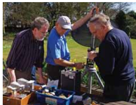
PHOTO 2: Testing the gain of a dual band 10/24GHz feed mounted on a Sky minidish at the recent RAL Microwave Round Table antenna measurement session. Left to right, Christian, F1DLT; John, G4BAO and Brian, G4NNS. A full report on RAL will appear in the next column. Photo: G4ALY.
