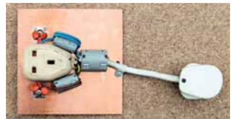
PHOTO 2: A VHF LISN for EMC conducted emission testing up to 300MHz.
