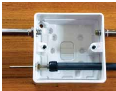
PHOTO 2: Mounting arrangements for the ferrite rod and dipole elements.
