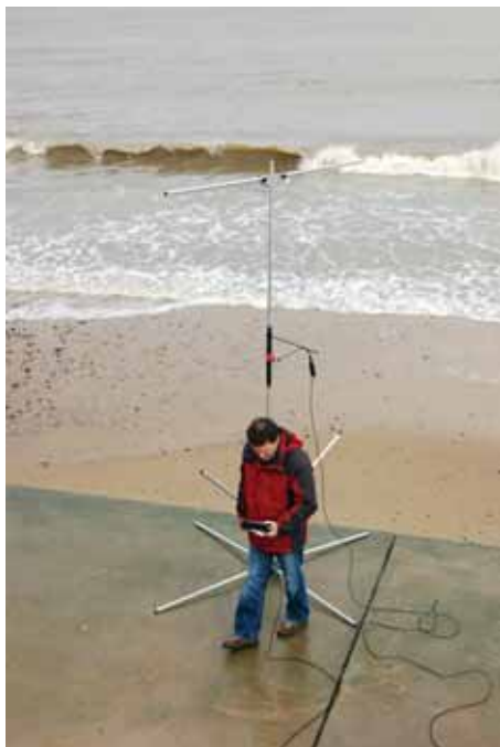
Set up on a very windy Norfolk beach took just a few minutes - This is Chris GODWV checking the SWR.
