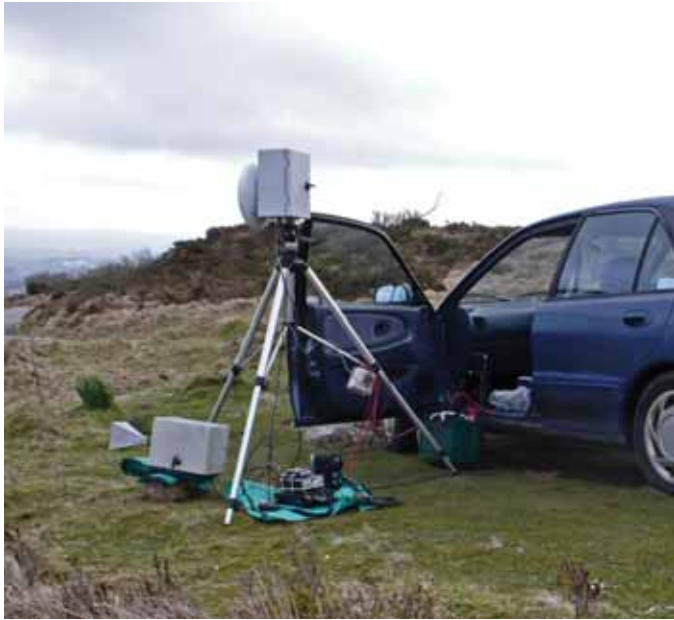
PHOTO 1: G4ALY/P operating portable on 10 and 24GHz from Kithill in Cornwall. The 10GHz portable system (with 19dB gain horn) is on the ground and the 24GHz system is on the tripod.
