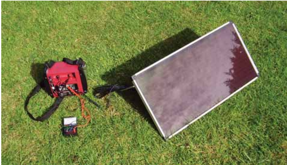
PHOTO 1: My 8W solar panel with cased 17AH SLA battery and multimeter to monitor charge.
