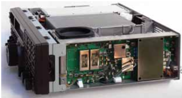
Removing the internal side shield reveals receiver A, mounted on the right side of the radio. The roofing filters (space for fitting 300Hz left) are readily accessible via a small hatch in the side shield.
