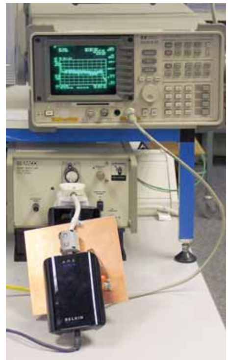
PHOTO 3: Laboratory testing of Gigabit Powerline Adaptors at VHF.
