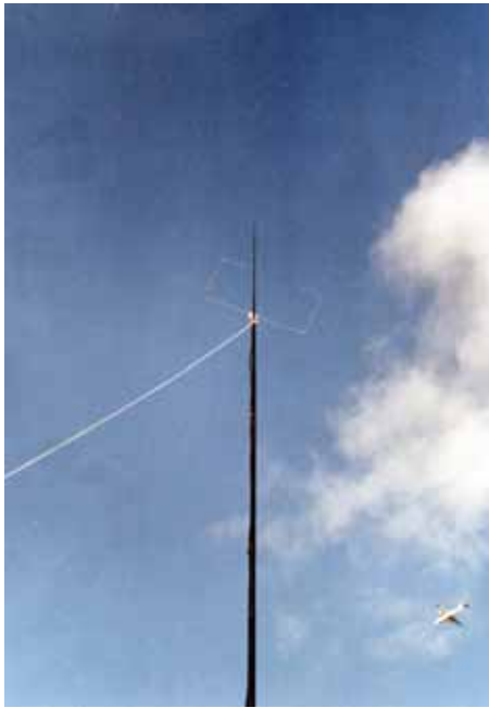
PHOTO 1: M5AEO's coat hanger omni antenna for 2m.
