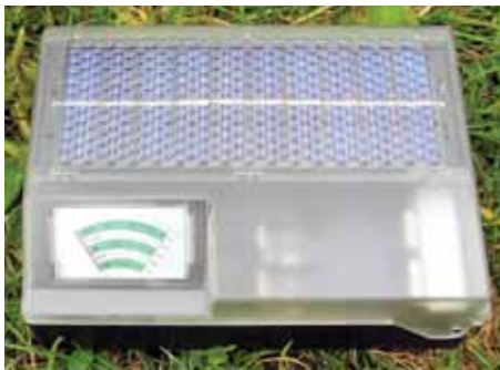
PHOTO 5: This neat solar-powered charger reckons to charge a pair of 500mAh AA batteries in 3-6 hours. 2500mAh NiMH cells would take 15-30 hours of sunlight to recharge from flat.
