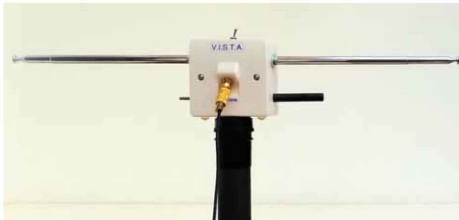
PHOTO 1: The complete VISTA antenna, shown with the two 1.3m long 10 section telescopic dipole elements retracted. Extended, the antenna is just over 2.6m wide.
