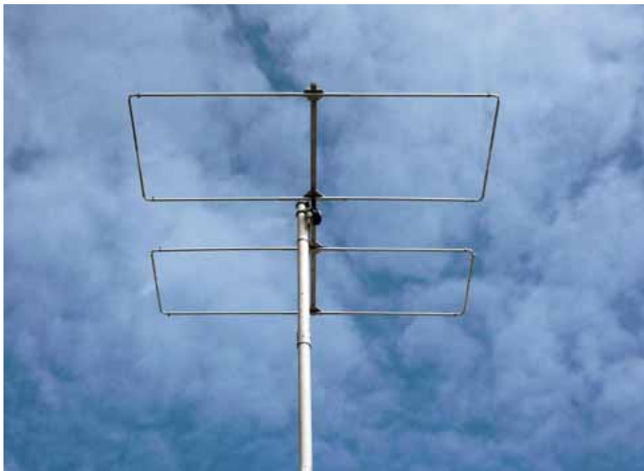
PHOTO 1: Completed 4m GW3YDX Super Moxon.
