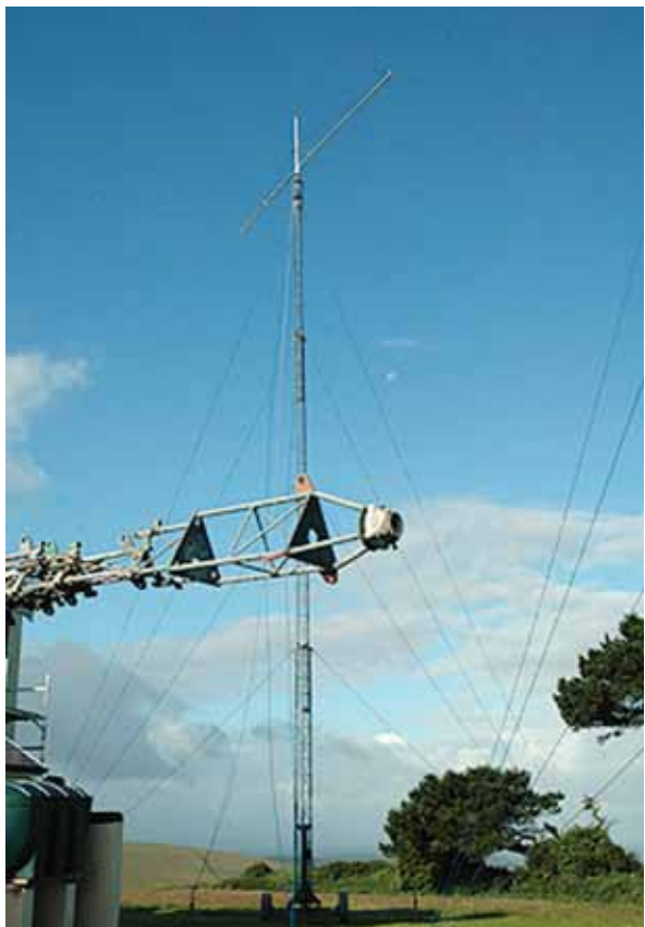
One of the two 80ft mobile Versatowers used to support 4-element 20m Yagis for GB7HQ in 2009. Photo G3TXF.
