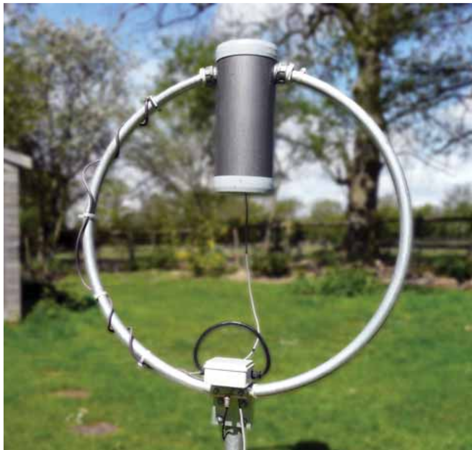
PHOTO 2: G3LHZ's AMA3 transmitting loop antenna with the 'twisted gamma' match. The original coupling loop shown is disconnected.
