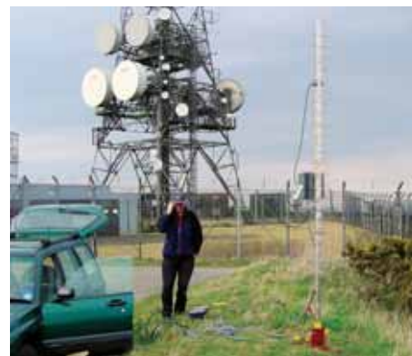
PHOTO 4: GM3SBC Ed's planar array for 1.3GHz. He uses two of these to provide a very wide beam width pattern. No rotator is necessary. Photo: GM3SBC.
