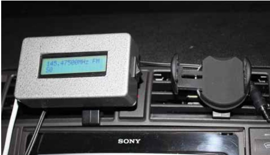
PHOTO 1: Remote display installed on car air vent. The mount was created from a mobile phone holder like the one on the right (see text).
