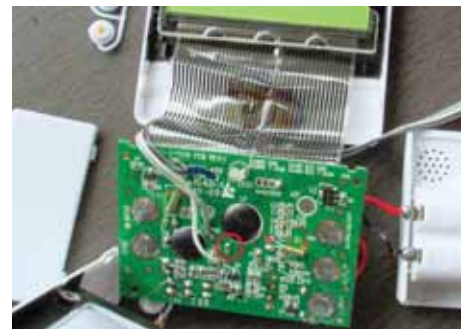
PHOTO 2: Flying leads connect the MSF receiver in this clock to the outside world. One of the added protection resistors is circled (see text).
