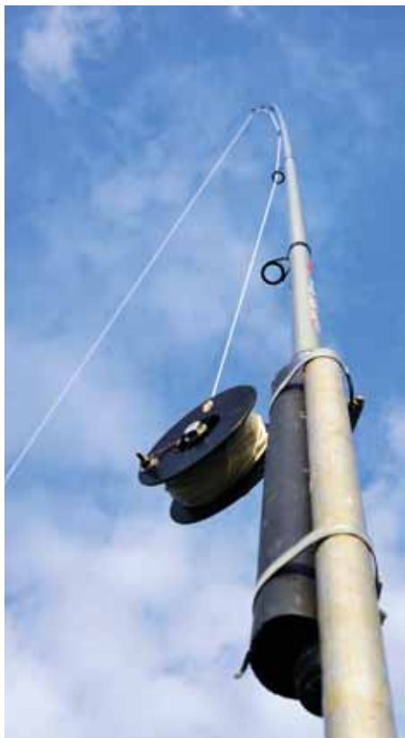
PHOTO 1: General view up the fishing pole showing the support pole, sleeve, reel and rod.
