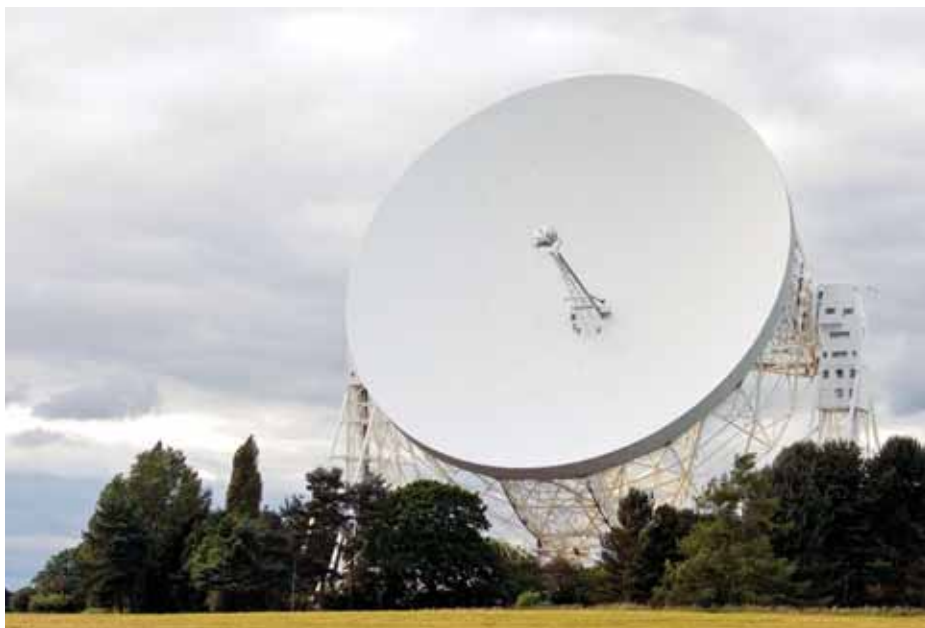
PHOTO 1: The Lovell Telescope at Jodrell Bank is 76.2m (250') in diameter – that's 4560 square metres, or well over an acre. At microwave frequencies, its beamwidth is very narrow – and therefore its gain is huge. But would an amateur signal from it reach Alpha Centauri? (Photo courtesy Mike Peel, www.mikepeel.net ).
