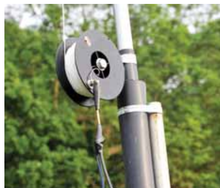
PHOTO 5: Attaching the feed (the antenna was not deployed at this point, which is why the antenna wire is not visible).
