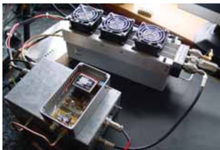
PHOTO 2: 2.3GHz band transverter and Spectrian 60W amplifier used by G3VKV to work GM4BYF/P at 360km on SSB during the May contest. Antenna used was a 16dBd Wimo Yagi fed with Ecoflex 15. Photo: G3VKV.
