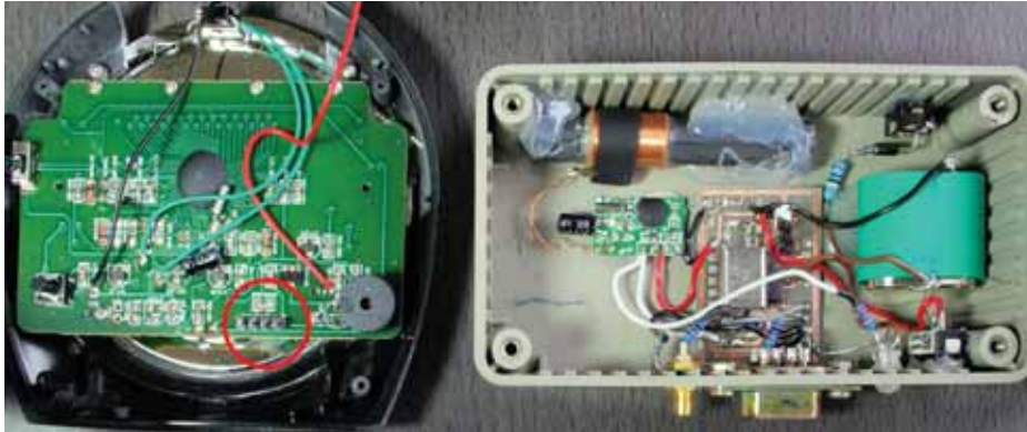
PHOTO 1: Circle shows original location of the MSF receiver module in the Acctim Radio Controlled Clock. The module (green PCB & ferrite aerial) has been transplanted into my time code generator project (right).
