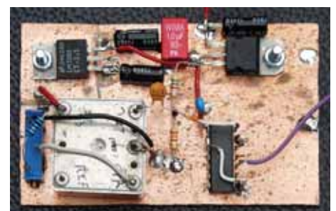
PHOTO 1: Completed reference oscillator.
