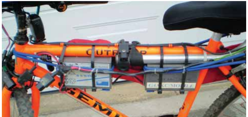
PHOTO 4: The primary pair of 7AH batteries that provide power to the radio.
