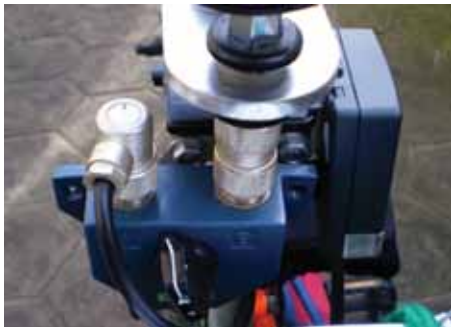
PHOTO 3: Aerial switch located immediately underneath the main aerial mount.
