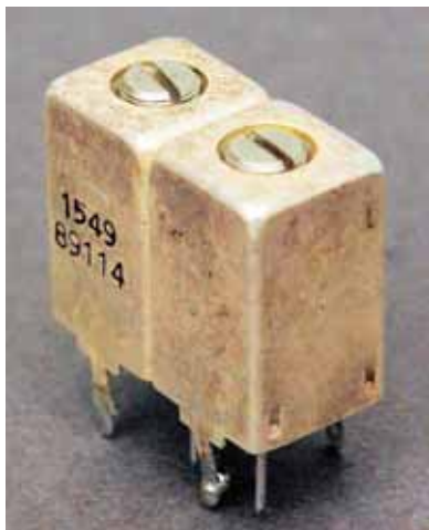
PHOTO 2: 5HW two-chamber helical resonator suitable for VCO use.
