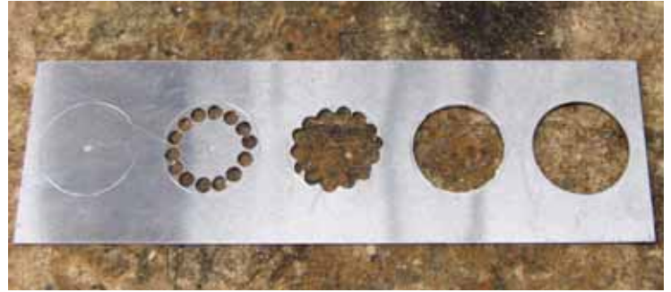
Cutting a round hole by using a series of drilled holes.
