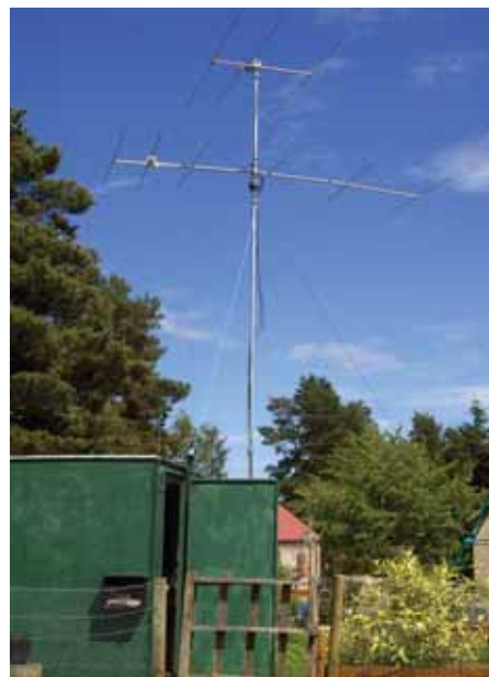
PHOTO 2: The 6m and 4m antennas at the QTH of Cris Henderson, GM4FAM.
