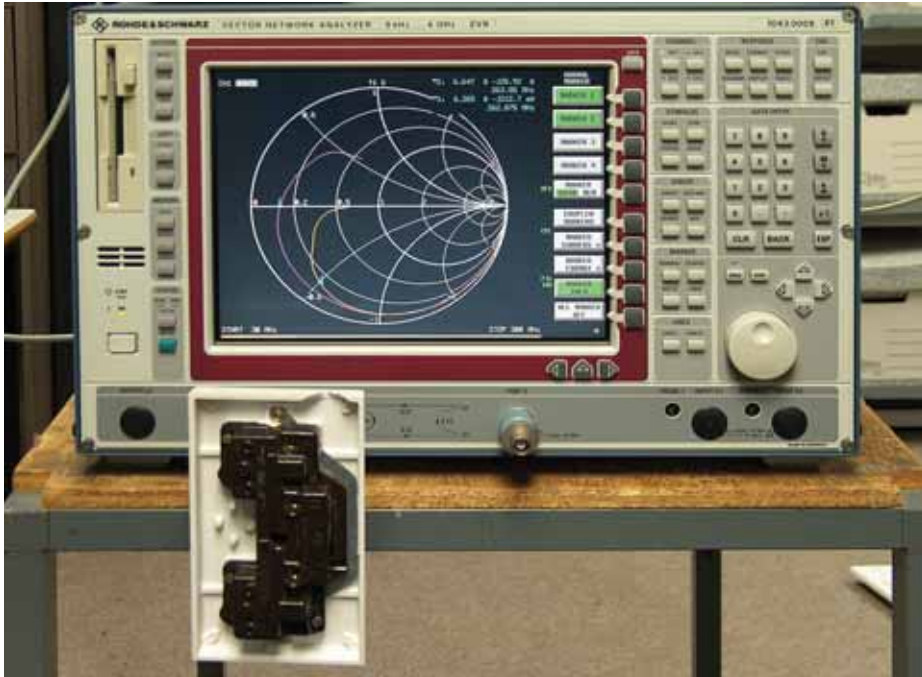
PHOTO 1: RF testing of a UK 13 amp double mains socket on a network analyser.
