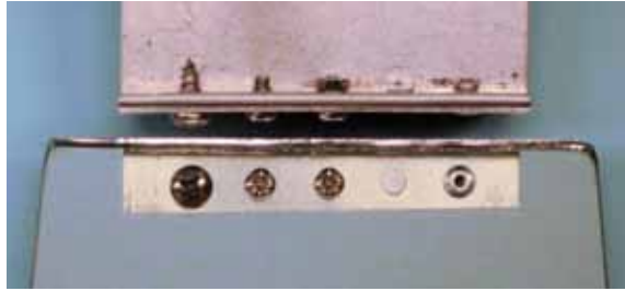
Different types of fastening. From left to right, self-tapping screw, screw for threaded hole, nut and bolt, flush rivet and pop rivet.
