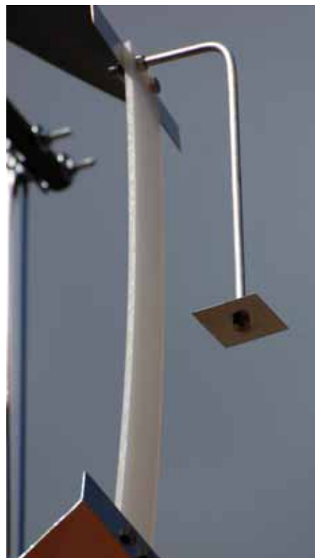
Close up of the tuning rod.
