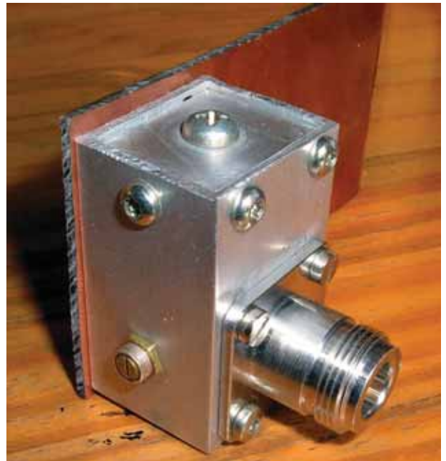
PHOTO 1: A homebrew 23cm GaAsFET preamp with a quarter wave cavity input circuit.
