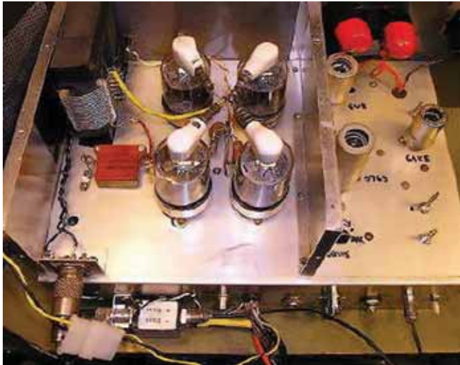
VE7BDQ's 136/500kHz transmitter using four 6146s. A good way to keep warm next winter!
