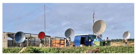
PHOTO 1: The French team set up in Portugal, showing the dishes for various microwave bands and the 14MHz dipole for liaison. Photo: Andre, F1PYR.
