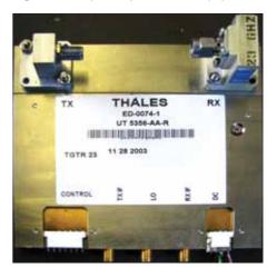
PHOTO 2: Thales 24GHz 'transverter' fitted with waveguide to coaxial adapters on the RF input and output.
