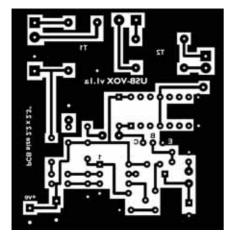
FIGURE 2: PCB foil pattern of the USB sound card interface, reproduced at 1:1.
