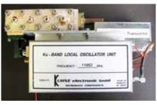
PHOTO 3: DB6NT transverter and local oscillator with 4 pole filter from a retuned surplus Telettra 23GHz system. This forms a basic 24GHz transverter system.
