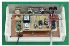
PHOTO 3: Prototype built on stripboard.
