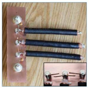
PHOTO 6: 70cm coaxial filter cable filter and (inset) how the coupling capacitors Ck were made from pieces of wire. The capacitance between the wires is all that's needed.
