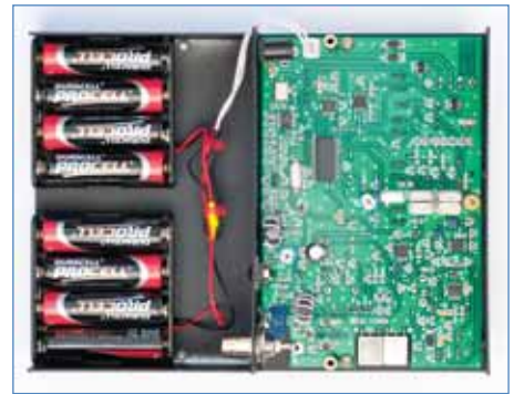
PHOTO 2: Inside the QRP transceiver.
