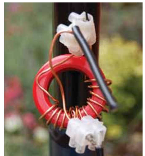
PHOTO 1: The transformer is wound on a T200 (red) toroid. The coax capacitor is connected to the upper terminal block.
