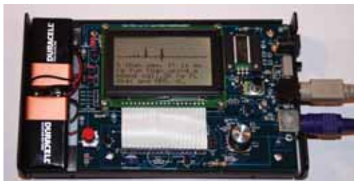
A self-contained PSK31 terminal – P79
