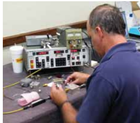
PHOTO 5: Tommy, WD5AGO, in front of his Eaton 2075 noise figure and gain analyser, making one of the many noise figure and gain measurements.
