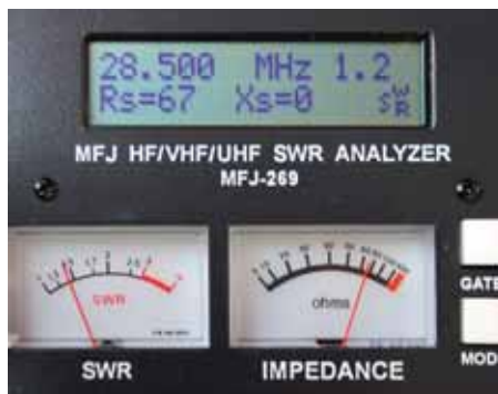
PHOTO 2: At resonance the aerial is quite well-behaved.
