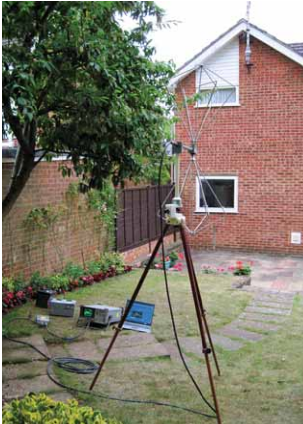
PHOTO 1: VHF radiated emission testing of PLA devices from 30-300MHz.
