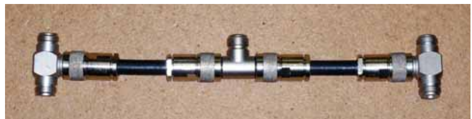
PHOTO 3: The 4-way power splitter.
