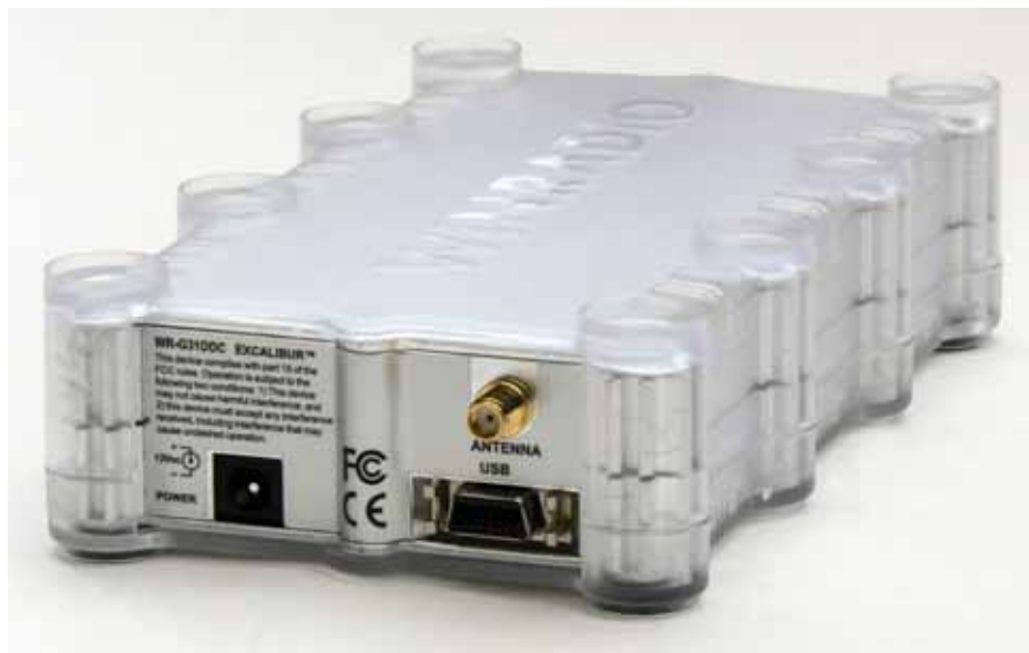
PHOTO 1: The Excalibur receiver hardware is contained in a small shielded box inside a clear plastic case.
