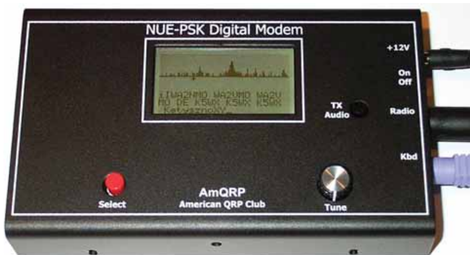
The NUE-PSK Modem provides standalone PSK31 and RTTY operation without a PC.
