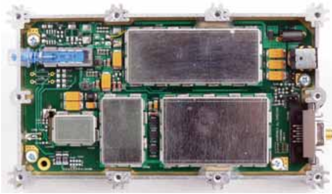
PHOTO 2: The receiver main printed circuit board.
