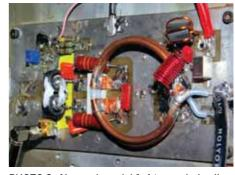
PHOTO 3: Air cored coaxial 1:4 transmission line transformer used for the output matching of a 250W VHF linear amplifier.
