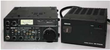
Icom IC720A all band AM/SSB/CW HF transceiver with general coverage receiver, no microphone. ICPS15 matching PSU.
