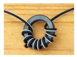
PHOTO 4: Wrapping my keyboard USB cable round a choke stopped it generating spurious characters.
