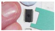
PHOTO 5: An IC upside down in a slot in a card, ready for tinning, and the piece of plastic cut to grip it for soldering to the PCB
