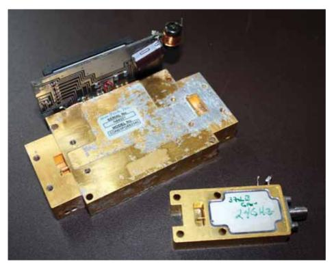
PHOTO 1: Millitech 2.5W amplifier together with a smaller 500mW Milliwave power amplifier.
