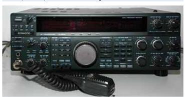
TS-950S HF transceiver, SSB, CW, AM, FM and FSK on all HF amateur bands including the WARC bands with 150 watts input.
