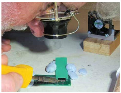
PHOTO 1: Good magnification is essential, as is close working. The small fan is to disperse smoke from the flux.
