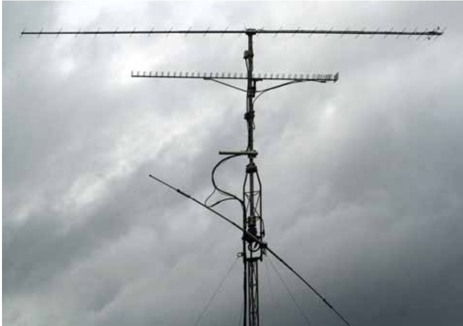
PHOTO 1: 39-element Quad Loop Yagi for 1.3GHz, 28-element Yagi for 432MHz and 10/15/20m trap dipole belonging to Martin, GM8IEM. (Photo: GM8IEM).
