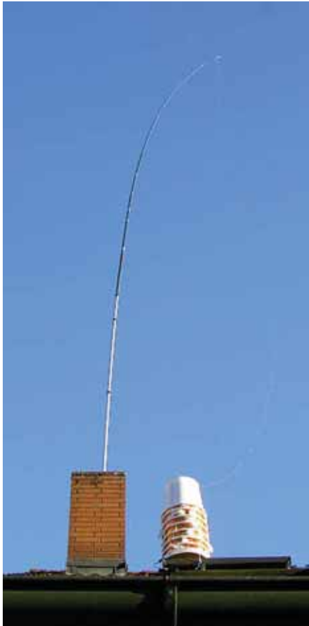
DF6NM's chimney-borne telescopic support pole and roof-mounted VLF coil.
