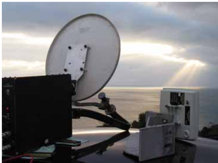
PHOTO 2: 10GHz dish (left) and 3.4GHz patch antenna on the roof of GJ4ISM/P car on Jersey, during the October opening. (Photo: GM4ISM).
