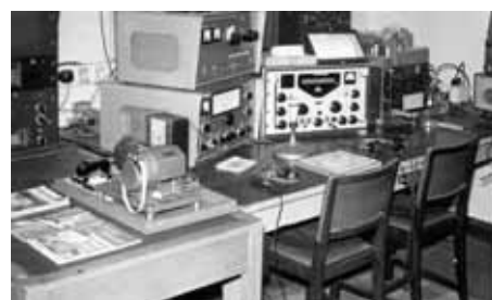
Creed and GNT Morse tape readers for the QRQ runs in the old HQ station at HMS Mercury .
