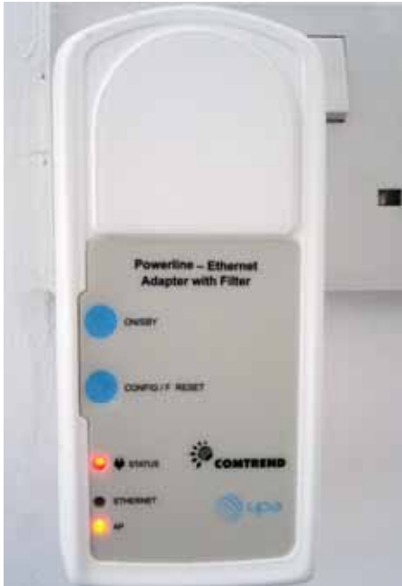
PHOTO 1: A Comtrend DH10P similar to the ones that are being replaced by BT Vision. (Photo: G3JWI).
