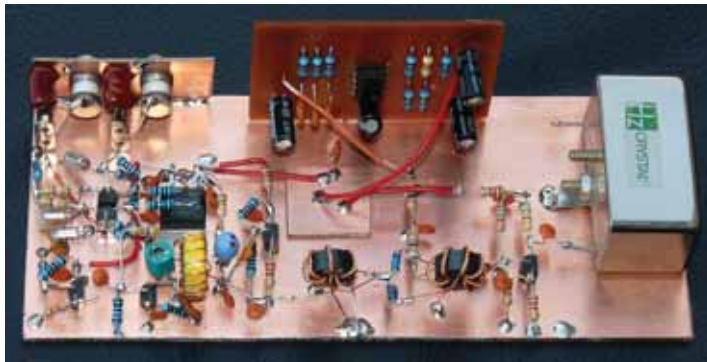
PHOTO 1: The SSB exciter that we build this month. The oscillator section is on the left, balanced modulator bottom-centre and the crystal filter on the right. The PCB at the top is the mic amplifier.
