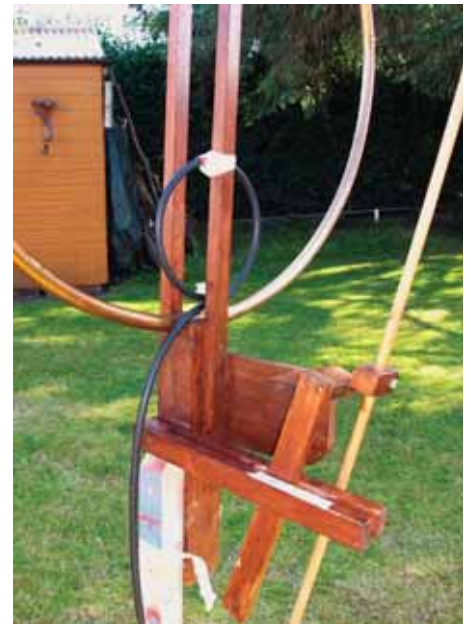
PHOTO 4: The Faraday coupling coil and the fine-tuning lever in more detail.
