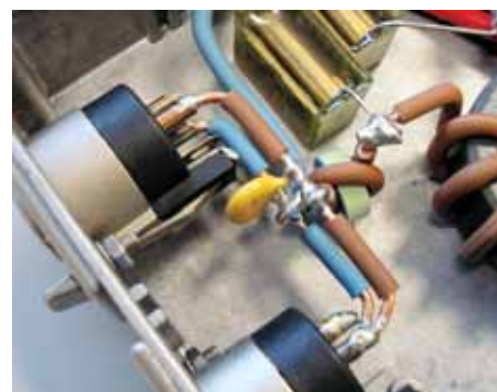
PHOTO 2: Position of C3 within the filter. Note L2 to the right of C3.
