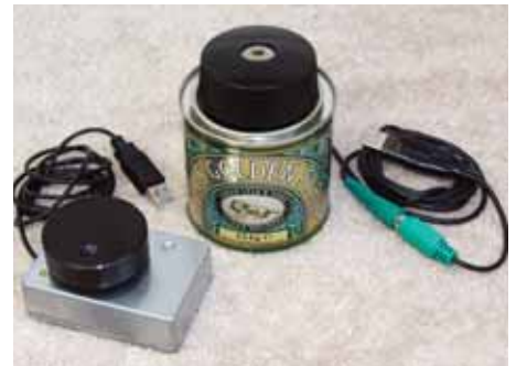
PHOTO 3: The final two SDR tuning wheels made from scrapped scroll-wheel mice with different types of rotary encoder.
