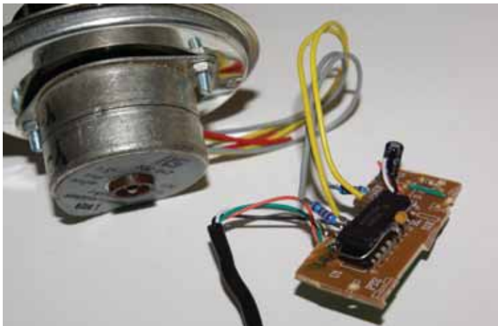
PHOTO 2: Modified PCB, with stepper motor and line receiver chip sitting on top of the mouse controller IC.
