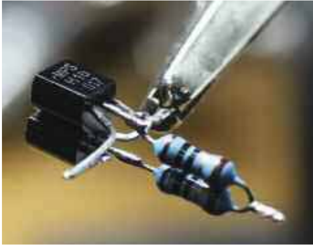
PHOTO 2: The double-decker arrangement of the post mixer amplifier transistors.
