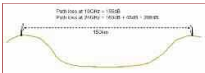
FIGURE 2: The additional (water vapour) loss on a 24GHz path compared to the loss at 10GHz where water vapour is not a problem. Reference RSGB Microwave Handbook , volume 1, System analysis and Propagation, page 3.6, fig 3.6.
