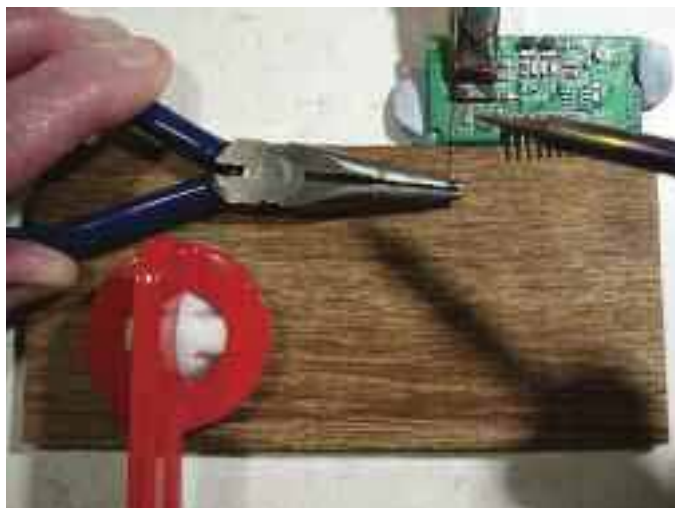
PHOTO 7: The PCB and IC securely fixed before the second side is started, to prevent a repeat of the situation in Photo 5.
