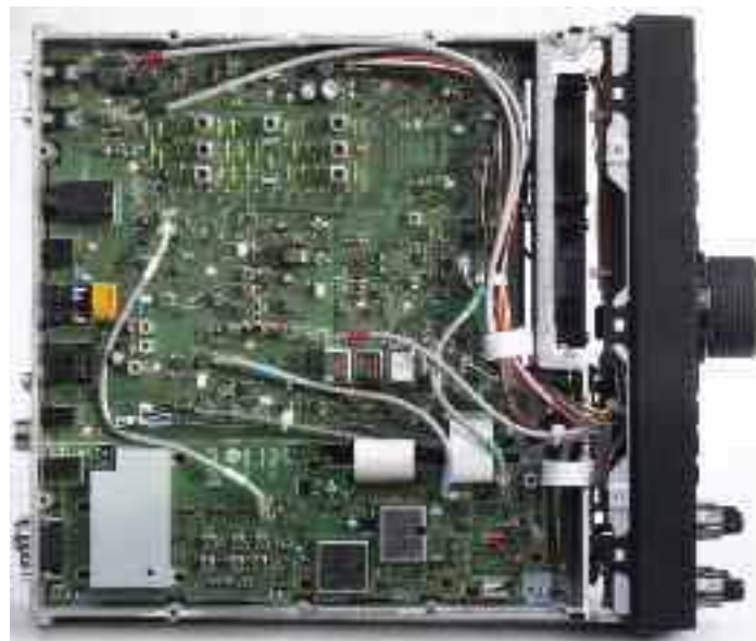
PHOTO 3: Underneath view showing signal processing boards.
