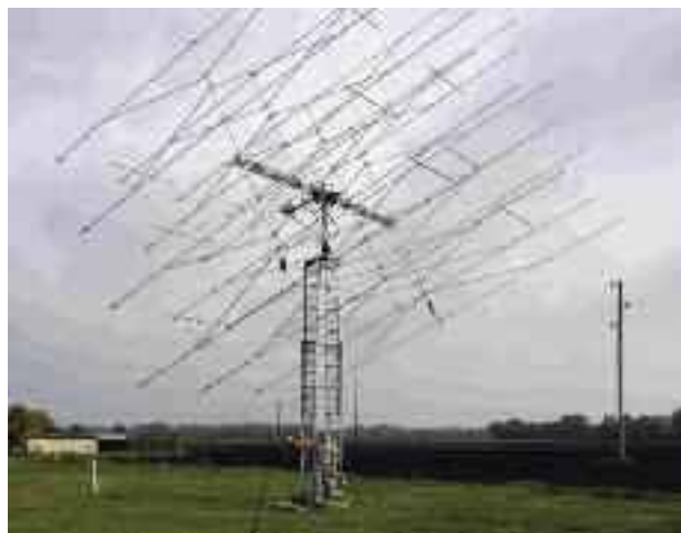
PHOTO 1: The 432MHz antenna system at the QTH of Bernd Wilde, DL7APV.
