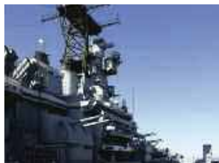
Aft view of the superstructure starboard side: antennas, missile launchers, CIWS, chaff launchers and 5" guns.
