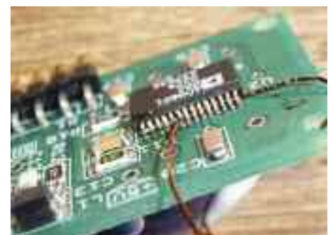
PHOTO 3: Part way through the removal process with five pins free.
