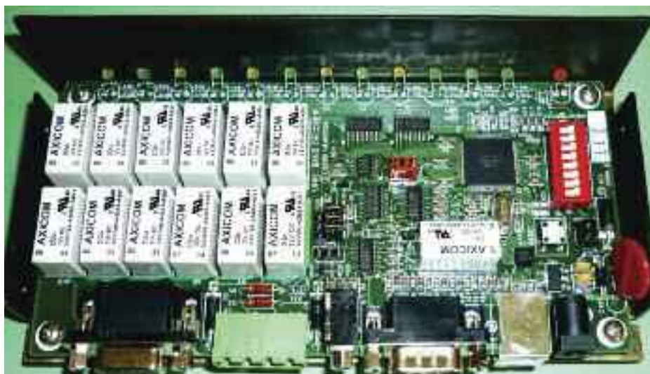
Photo 3: Inside the unit you can see the relays and switches.
