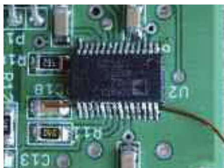
PHOTO 2: Passing a fine enamelled wire behind the pins.
