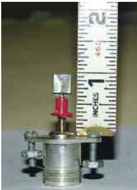
PHOTO 4: The completed feed assembly.
