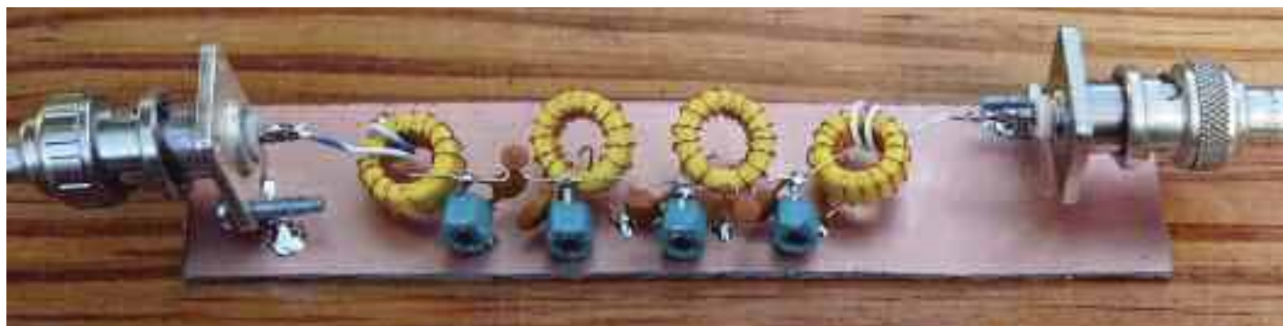
PHOTO 4: The finished 17m filter.
