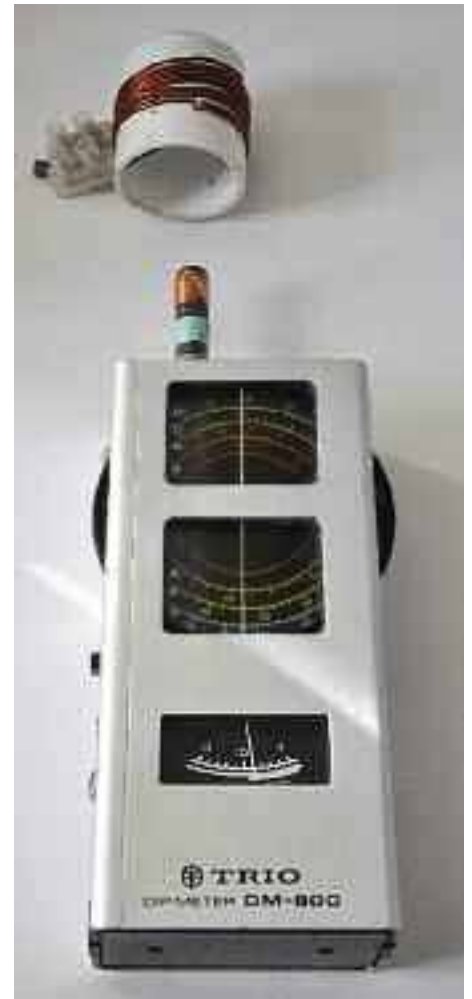
PHOTO 3: Testing the Trio DM-800 dip meter.
