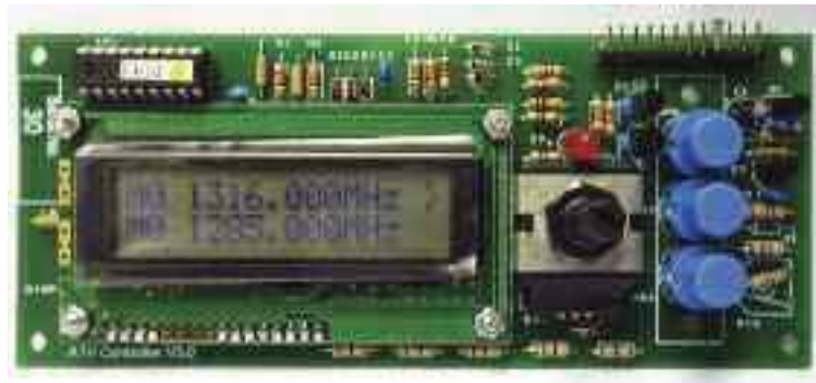
PHOTO 1: The G6ALU Comtech ATV controller.
