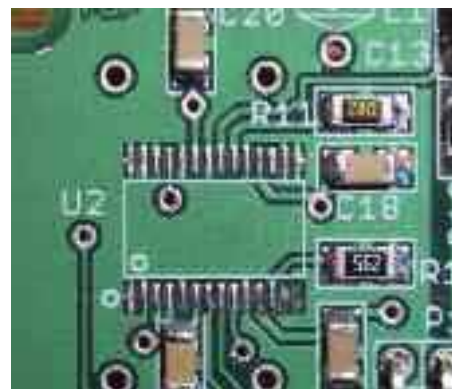
PHOTO 6: Cleaned up nicely and ready for the replacement.
