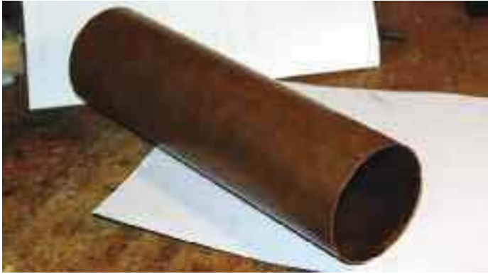
PHOTO 2: Raw 76mm copper tube cut to length.
