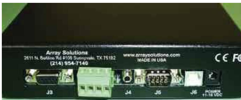
PHOTO 2: The rear panel connectors.
