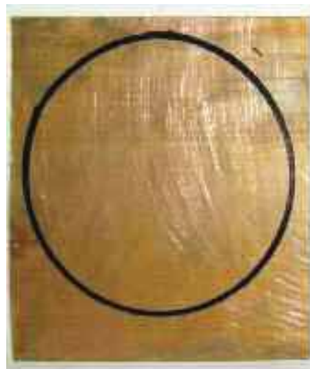
PHOTO 5: The end plate can be any shape as long as it's larger than the outside diameter of the tube.
