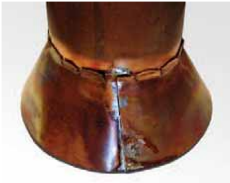
PHOTO 3: Soldering the conical hood to the tube.
