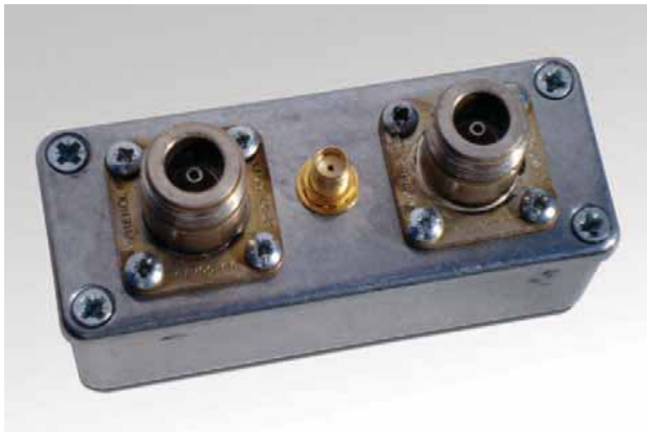
PHOTO 1: Completed sniffer. The sniffed output is available at the SMA socket.
