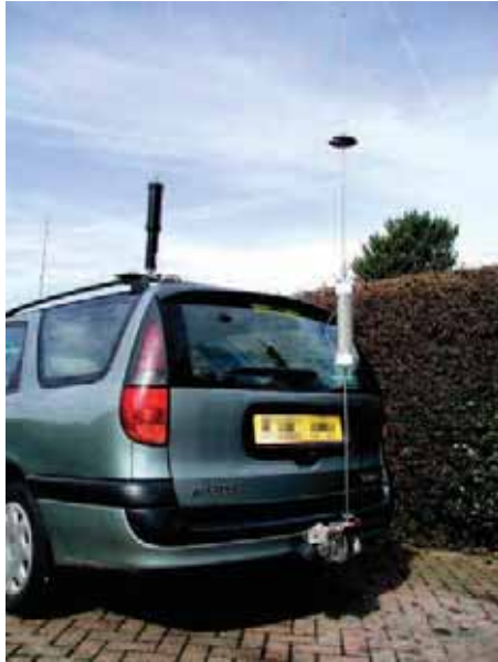
PHOTO 1: A Texas Bugcatcher antenna mounted on the tow bar on the rear of a vehicle. It uses a single large inductance with tapping points and a wander lead to short out the unused sections of the coil.
