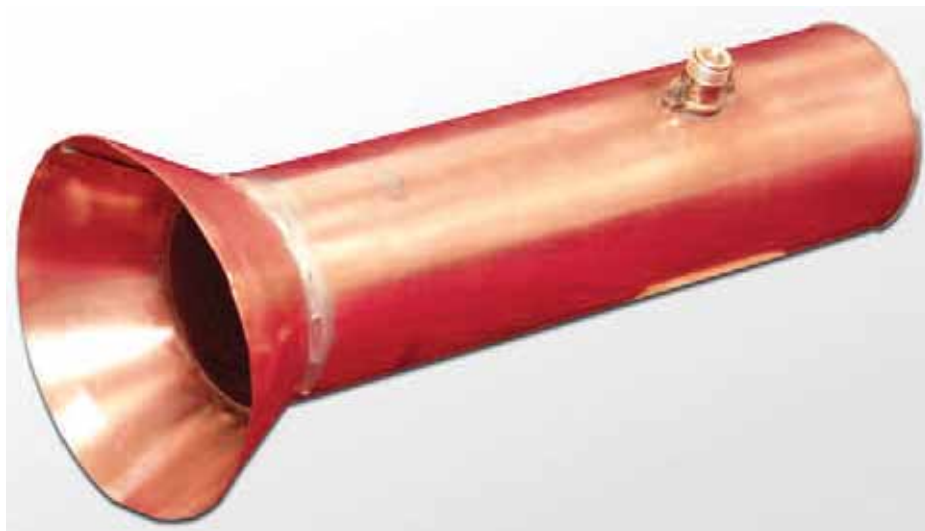
PHOTO 1: The completed antenna with the add-on hood that gives an extra 3dB of gain.
