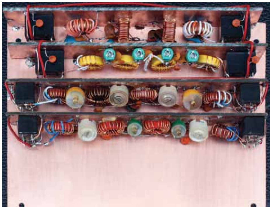
PHOTO 2: Part way through constructing the filter bank, with four sets completed.
