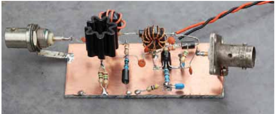
PHOTO 3: The completed low level transmit amplifier.
