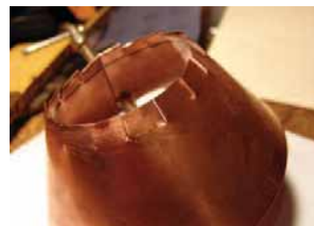
PHOTO 2: The copper sheet rolled into a cone, with strip cuts into the solder flange section.
