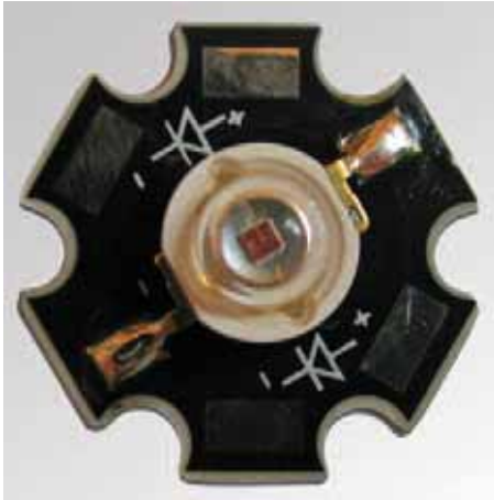
PHOTO 1: Edixeon 'Truopto' high intensity LED. These are available from Rapid Electronics, Colchester. Similar LEDs are available from Farnell and RS Components. Even higher power LEDs have recently become available. When ordering your LED make sure it has 'Lambertian' radiation characteristics.
