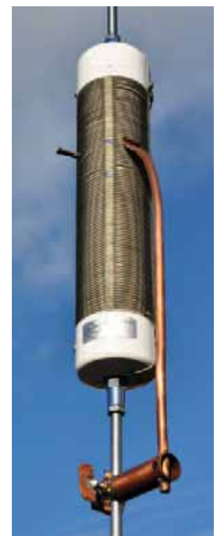
PHOTO 3: Modified Bugcatcher coil with sliding contact.
