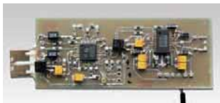
PHOTO 1: PCM2900 stereo USB codec (28 pin device, right) with a 3-port USB hub chip (quad package, left).
