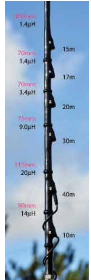
PHOTO 2: The centre section of an Outbacker Outreach antenna, with measured inductances for the bands 10, 15, 17 20 and 40m. The wander lead is shown with the 40m band selected.
