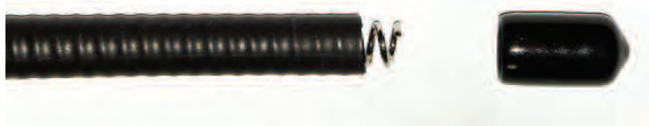
PHOTO 2: End cap removed from the antenna and a short section of the helical exposed.
