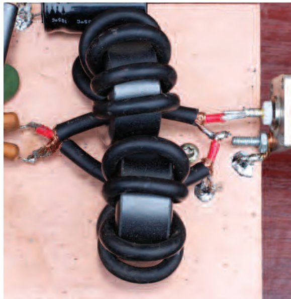
PHOTO 3: Close-up of the practical output transformer.
