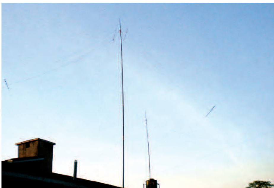
PHOTO 2: Two of the antennas at 5X1NH. In the foreground, nested dipoles for the HF bands, and in the background a dipole with removable links that can be set for any band.
