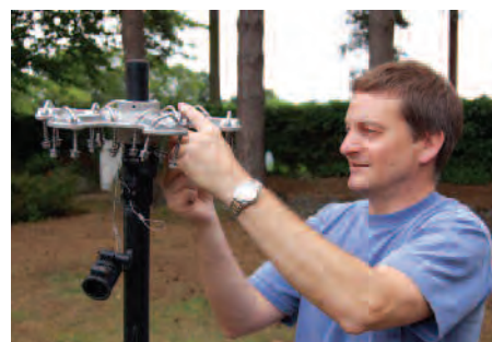
The first step is to fit the supplied fibreglass mounting centre post into the aluminium mast section and bolt this into place on the cast alloy HEXX plate.
