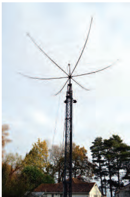
The five-band two-element Hexx Beam works quite well despite its unconventional looks.
