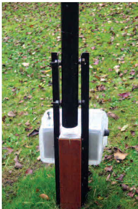
PHOTO 3: General mechanical arrangement of the support pole, angle iron and fibreglass pole.
