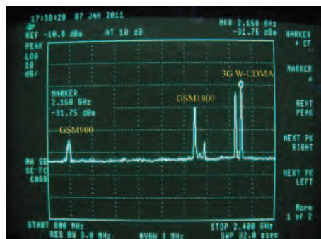
PHOTO 1: Frequency spectrum at the base of my 13cm band antenna feeder. The signals from left to right are GSM900, GSM1800 and 3G.
