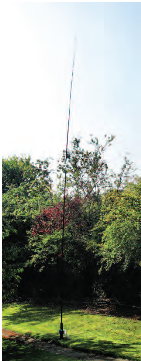
PHOTO 1: General view of the extended 40m vertical. Note the tilt-over base and box containing the matching components.
