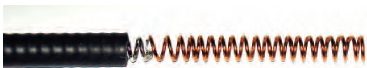
PHOTO 3: Additional wire soldered to end of helical and wound round a former.
