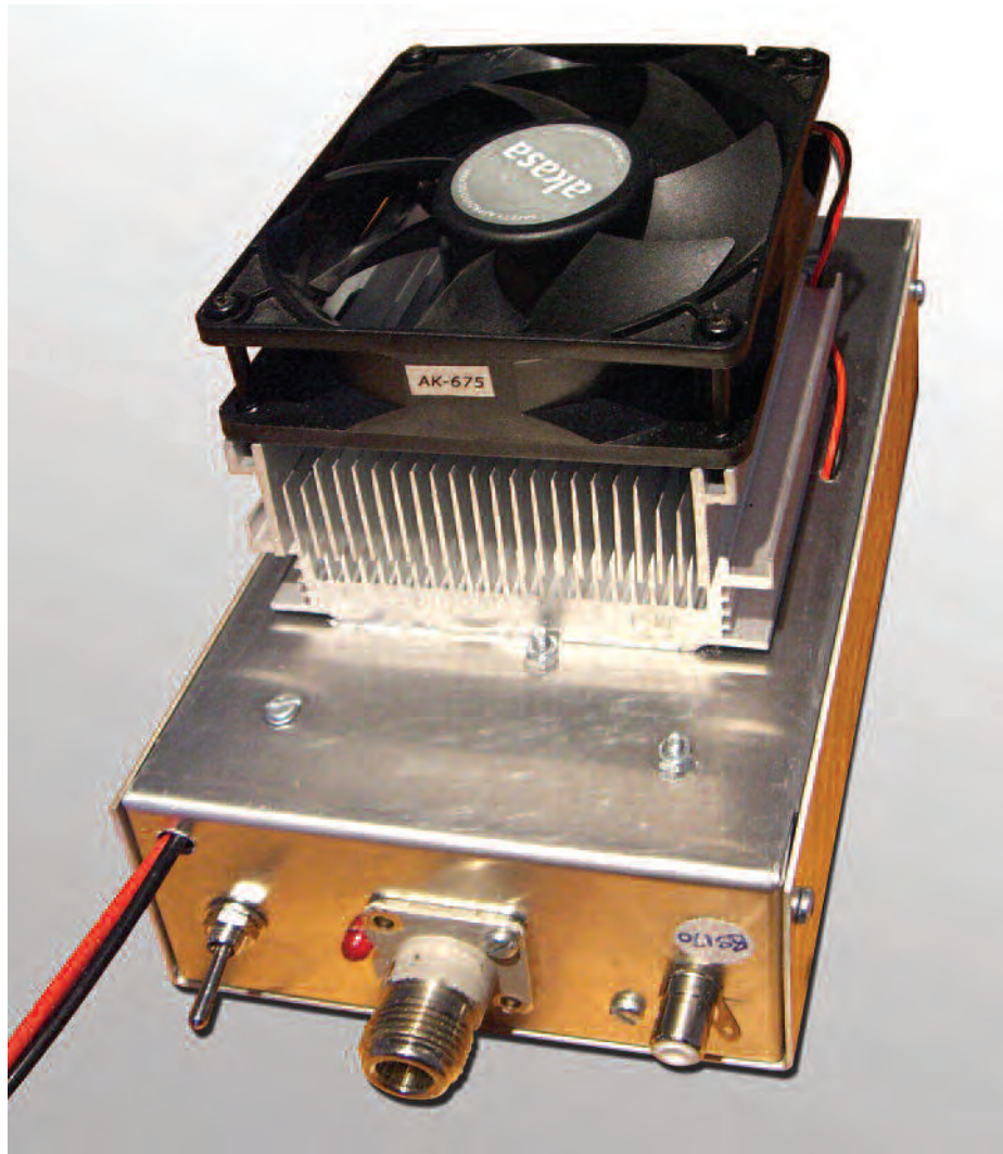
PHOTO 1: General view of the 50W 4m amplifier. The heatsink and fan were originally intended for a CPU (see text).
