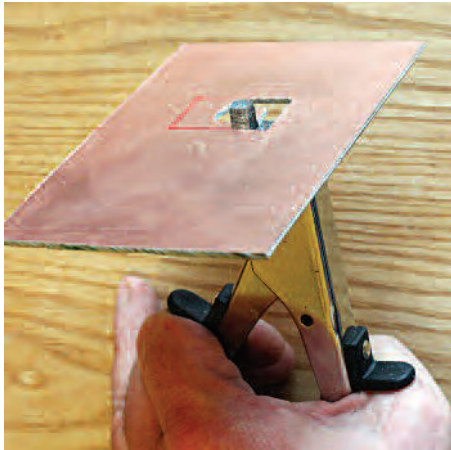
PHOTO 2: How I used the new nibbler to cut a rectangular hole in the PCB so that the MOSFETS can be screwed to the heatsink.
