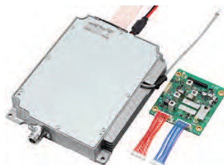
The optional UX-100 band unit gives 10W on 23cm.
