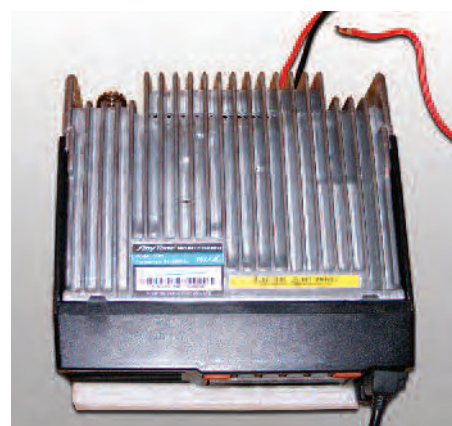
The image of the underside of the AT-5189 shows clearly the heat sink as it extends near to the whole underside of the AT-5189 with no stand or feet.
