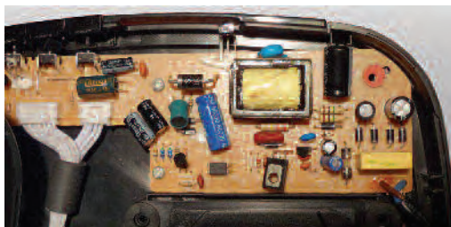
More PSU examples with no filtering? – p72
