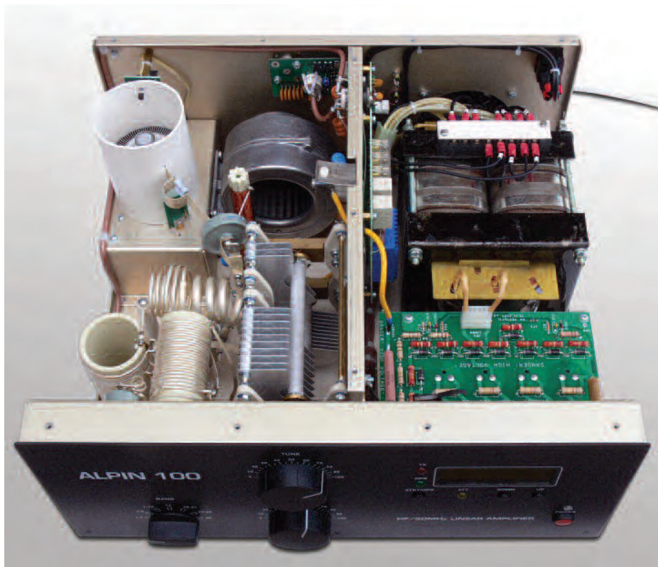
Amplifier with case removed showing RF deck (left) and PSU (right).
