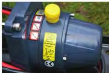
PHOTO 2: The winches are fitted with series-wound reversible motors.
