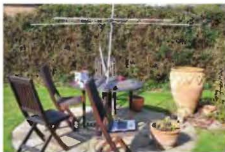
PHOTO 2: Test arrangement showing the antenna under test, the AIM4170 and the laptop computer.
