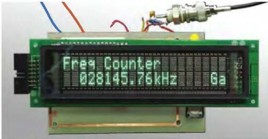
PHOTO 2: Frequency counter display with a vacuum fluorescent display installed. (The PIC code was written for a 4 line display, so part of the text showing the gating interval is missing).
