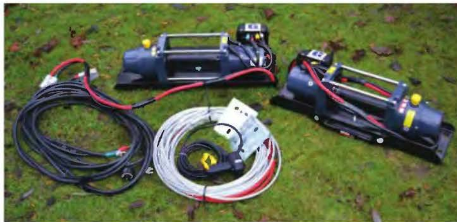
PHOTO 1: The contents of the winch boxes - everything you need, bar the battery.
