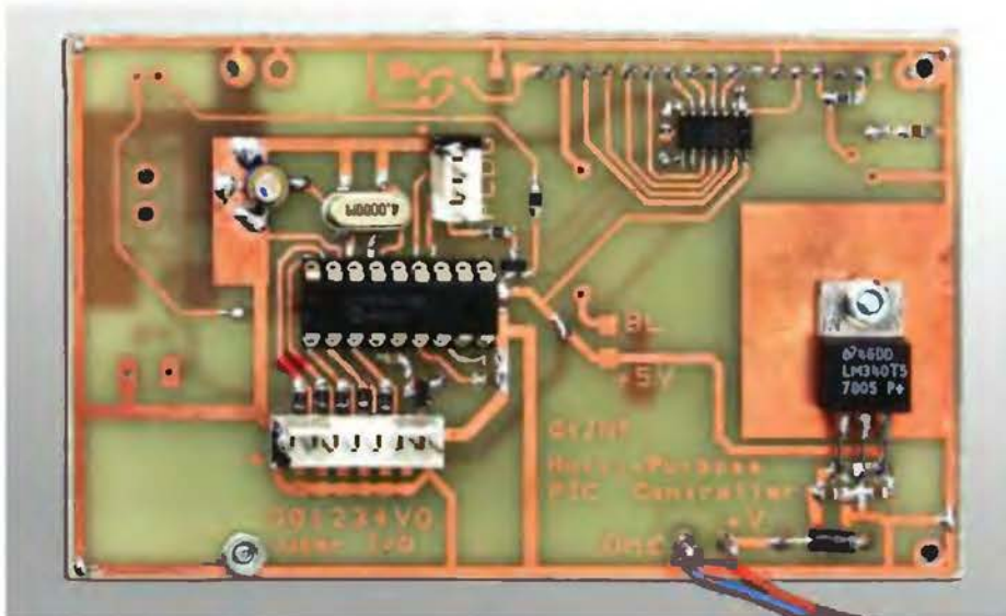
PHOTO 3: The original breadboard PCB from the rear showing components and input/output connections.
