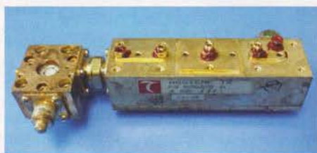
PHOTO 1: Circulator (left) attached to a commercial 13cm interdigital filter.
