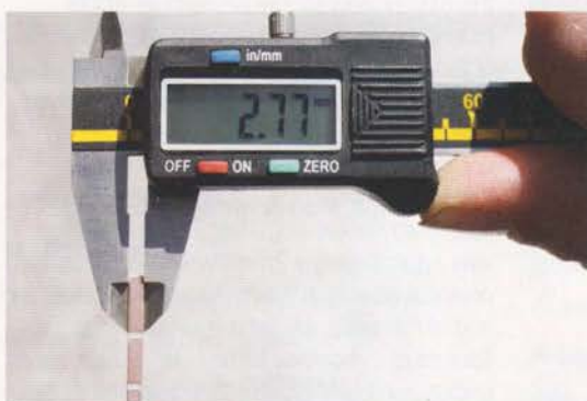
PHOTO 2: Homebrew 50Ω stripline made from a carefully filed offcut of fibreglass PCB (see text).
