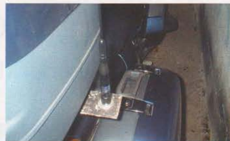
PHOTO 4: The antenna is mounted on a flat bar that's secured to the top box mounting frame.
