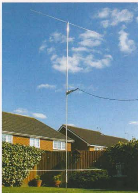
The coax must come away at an angle.
