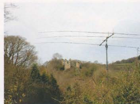
PHOTO 3: PICaYAGI at full element extension showing modest element droop.
