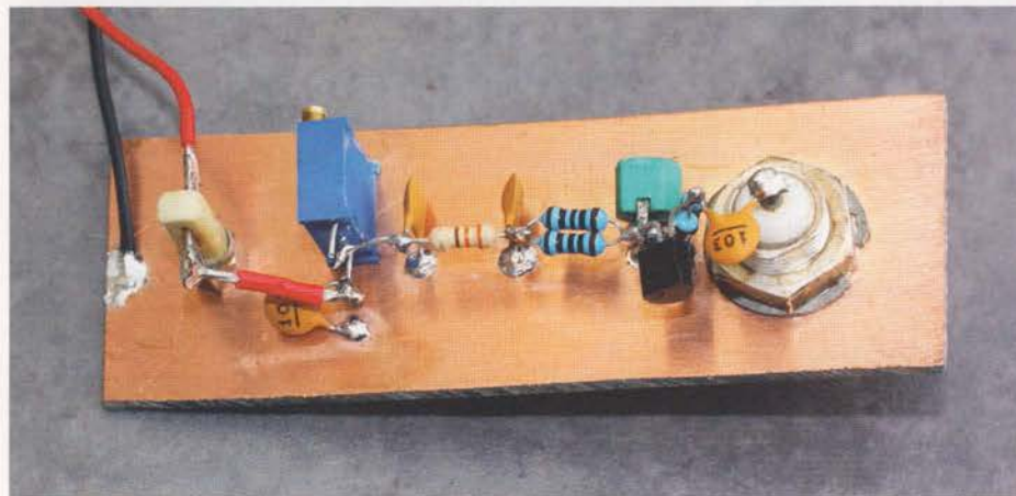
PHOTO 1: A homebrew noise source based on the circuit of Figure 2. An MPSH10 transistor base-emitter junction is used in place of the Zener diode (see text).
