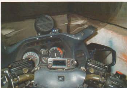
PHOTO 3: The control head and external loudspeaker mount neatly around the dashboard area.
