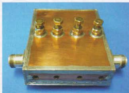
PHOTO 2: Homebrew 4 pole \lambda/2 line lookthrough filter made from PCB material.
