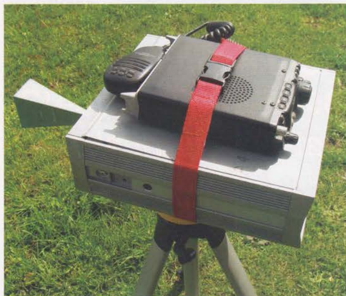
PHOTO 1: The new 24GHz transverter. The 20dB gain horn seen here is used for short range tests whilst a 30cm Cassegrain dish is available for long distance contacts. The FT-817 IF radio mounts on the top of the transverter with a simple webbing strap.
