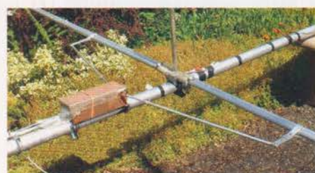
PHOTO 7: Controller in PCB box with GRP shrouding mounted on the boom.
