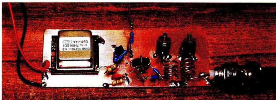
PHOTO 2: 200MHz reference clock consisting of a 100MHz OCXO module (left) and doubler circuit.
