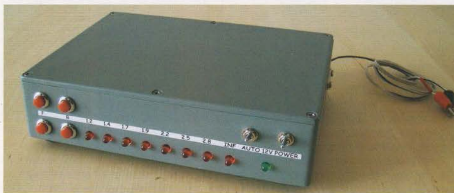
PHOTO 1: The complete BRATS project magnetic loop auto tuner control unit.
