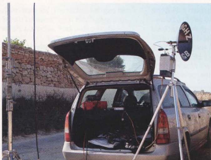
PHOTO 3: Mansueto, 9H1GB's portable 10GHz system set up in the back of his vehicle.
