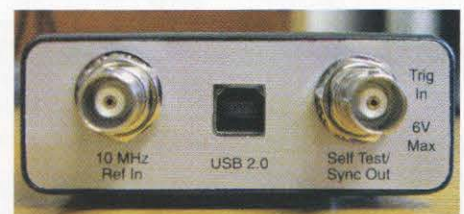
PHOTO 3: SA44B rear panel. The TG44 is similar.
