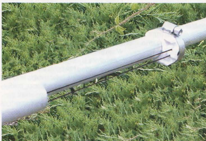
PHOTO 11: Braid tensioner made from a PVC pipe clip.
