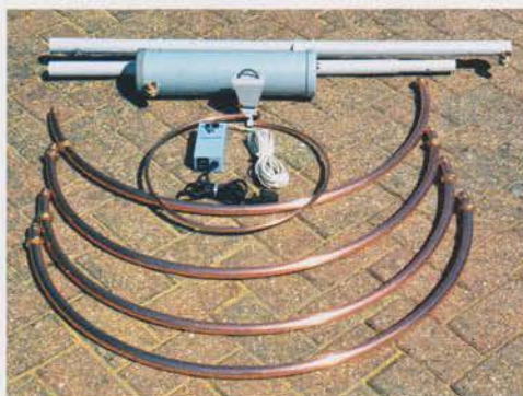
PHOTO 3: The kit of parts for the GMOSDV antenna.
