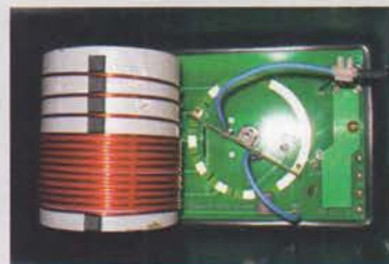
80m coil interior view
