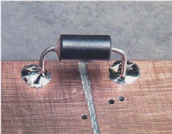
PHOTO 1: A ferrite bead on a wire link provides a DC link but AC isolation between the analogue and digital grounds.
