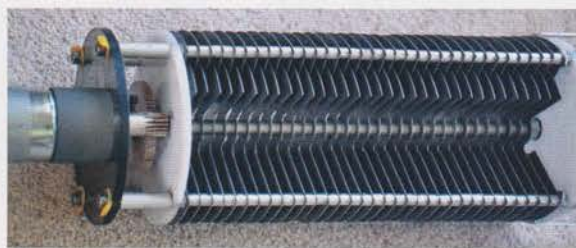
PHOTO 4: The loop tuning capacitor.
