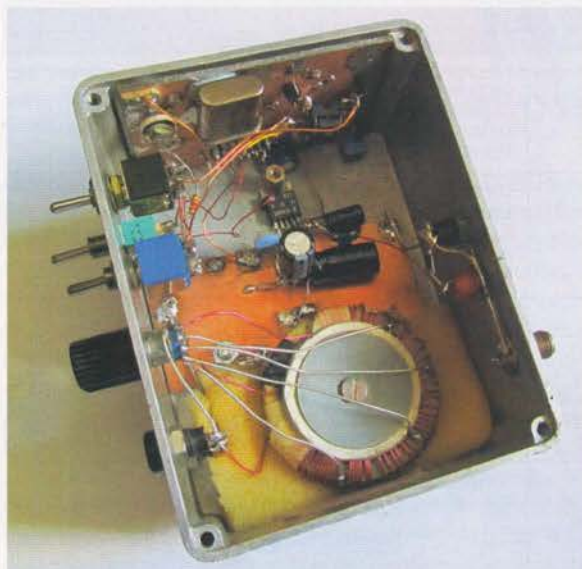
PHOTO 1: The completed VLF beacon test transmitter, capable of about 5W output.
