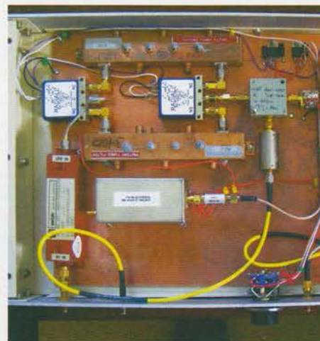
PHOTO 2: Inside view of the 13/9cm dual band converter.
