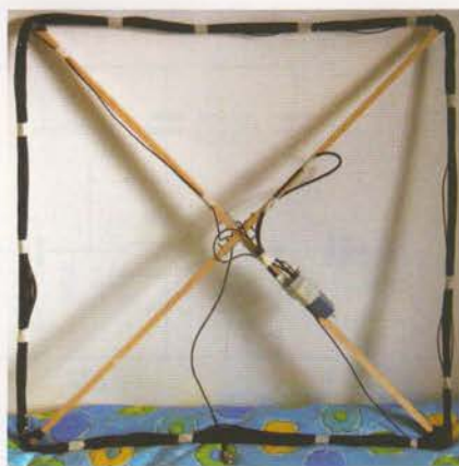
PHOTO 2: 30 turn loop receiving antenna with attached preamplifier.
