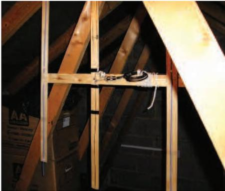
PHOTO 1: The G8PJC 145MHz three-element Yagi located in the loft. The elements are not hard drawn copper so need to be supported on wood battens.
