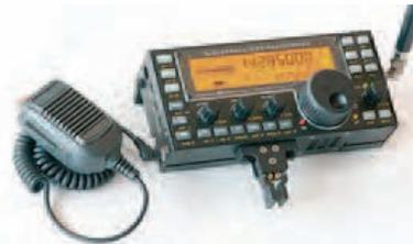
The revolutionary Elecraft KX3 puts the world in the palm of your hand! Despite its small size, it covers all amateur bands from 160-6 meters, operates in all modes, and has DSP-based features usually found only on larger radios.
