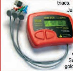
Just connect any way round and let the unit identify the type of component (Triac or Thyristor), the full pinout, the gate sensitivity and the gate voltage drop. The load test voltage is regulated to 12V, regardless of battery condition!
