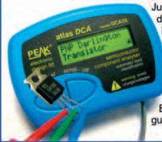
Just connect any way round to automatically detect MOSFETs, Bipolar Transistors, Darlingtons, Diodes, LEDs and more.
