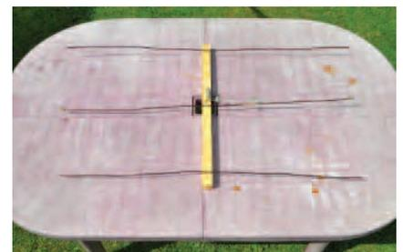
PHOTO 2: The latest edition of my 145MHz three-element Yagi with the elements made from 10SWG (3.2mm) enamelled wire.
