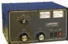
This Ameritron design gives a sensible power gain for a very reasonable price. It has a hunky built-in power supply with full monitoring of operation conditions. It uses three low cost 811A tubes to achieve 600W power output running from a 1500volt HT line. This desktop design can easily be accommodated. 350 x 210mm Weight: 14.51kg **£899.95 D**
