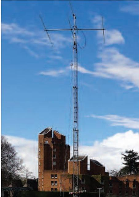
The 20m monobander + WARC dipole used for GR100MGY operations.
