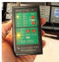
This compact device is a calibrated signal source that runs on an internal PP3 battery or an external 12v PSU. It is individually calibrated on the bands 160m to 2m and can be switched to generate either 1uV or 50uV. In addition it can generate a massive 0dBm signal. It is highly stable and locked to a programmed frequency on each band. This can be changed using the supplied data lead and a PC. It is great for receiver checking and S-meter calibration.
