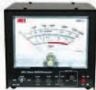
**MFJ-868** If you struggle to read your VSWR & output power, then help is at hand. This meter has a massive 6.5" instrument meter. It features "True PEP and Average" readings (which requires internal 9V cell or external 12v). The power saver circuit also only turns on when the meter is passing RF. Frequency coverage is 1.8 - 30MHz. Range 20/200/2kW. **£159.95 C**
