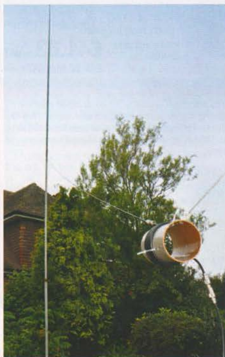
PHOTO 1: A vertical Controlled Feeder Radiation dipole for 14MHz, constructed by taping multi strand insulated copper wire and RG58 coax to a fibreglass support. The coax coil current choke can be seen in the foreground.
