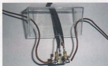
PHOTO 6: How the end of the feed and balun coax join the driven element. See also Figure 3.
