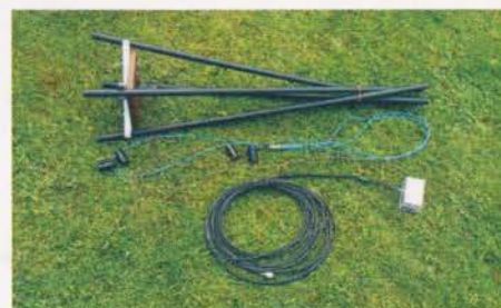
PHOTO 2: The antenna folds down to a compact size and shape for transport and storage.
