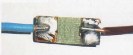
PHOTO 5: Insulating spacers made from PCB material allow an accurate 5mm gap to be maintained.
