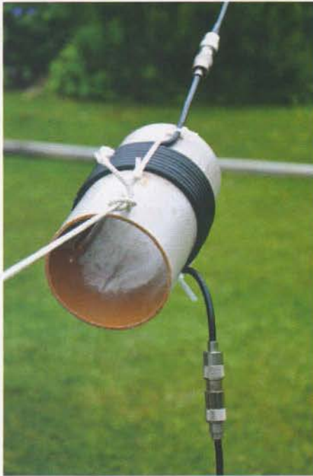
PHOTO 2: A coax current choke constructed from of 9 turns of RG super 8 coax wound on a 4.25in (110mm) plastic pipe.
