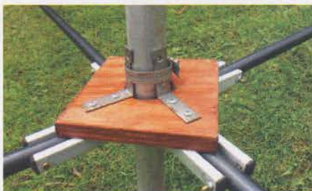
PHOTO 4: Attaching the antenna to a pole using a hose clamp.
