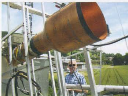
PHOTO 4: Close up view of the HB9Q 23cm circular polarisation feed horn. This is a W2IMU dual mode horn feed with screw polariser.
