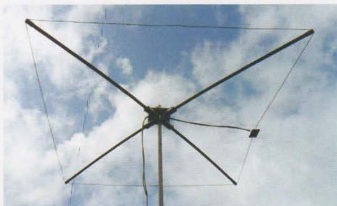
PHOTO 1: The 6m 2-ele collapsible antenna in operational configuration.
