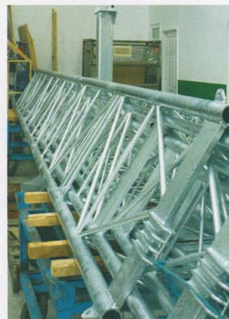
A partly completed tower, back from being galvanised.
