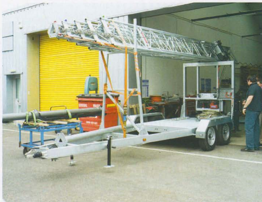
The new 31.5m trailer tower.
