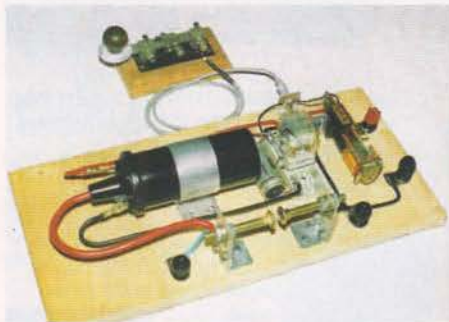
PHOTO 1: My experimental spark transmitter.
