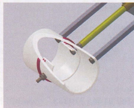
FIGURE 10: Cutaway view of the variometer showing the construction.
