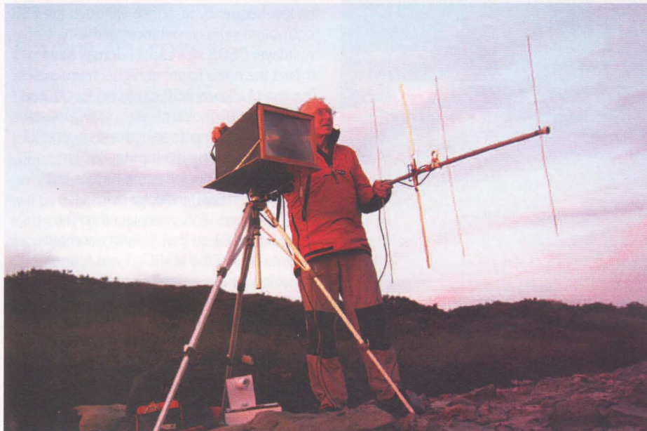
PHOTO 1: GOEWN with his compact 'TNG' optical transceiver (plus 144MHz Yagi for the talkback link).
