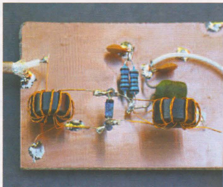
PHOTO 2: Double balanced mixer.
