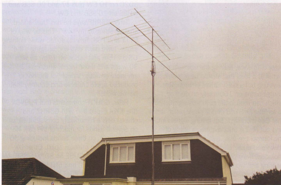
PHOTO 1: MOBKL's fine antenna array, consisting of (bottom) an M 2 6m 7-element Yagi on a 30ft boom. The middle antenna is an Eagle 4m 6-element Yagi and at the top is the M 2 2m 12 element Yagi. Photo MOBKL.
