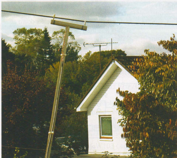
PHOTO 2: A short RF sampling loop in use on an overhead telephone line (NOT for use on power lines).
