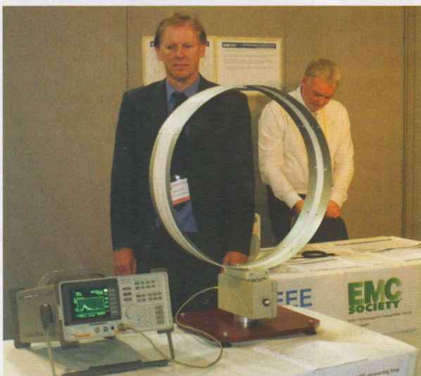
PHOTO 4: A prototype tuned loop HF measuring antenna being demonstrated by GOSNO at EMC UK 2012.
