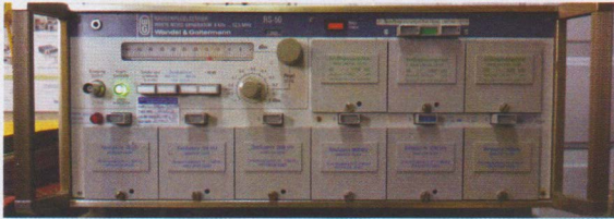
PHOTO 1: A typical white noise generator with filters suitable for NPR testing.
