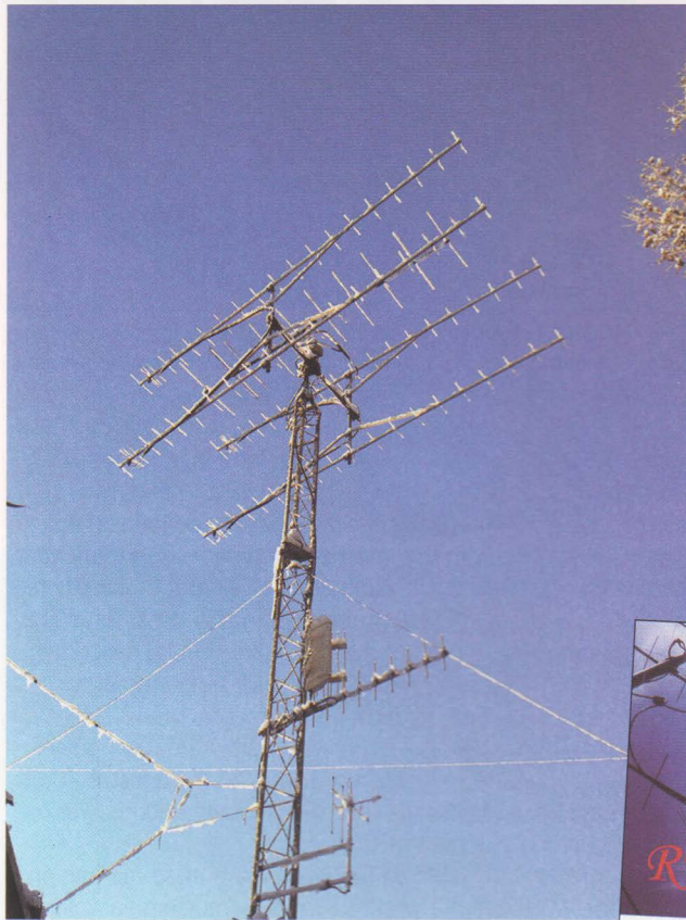
PHOTO 1: Ice covered F9FT 70cm Yagi array belonging to WA1ZMS in Virginia. Photo: WA1ZMS.
