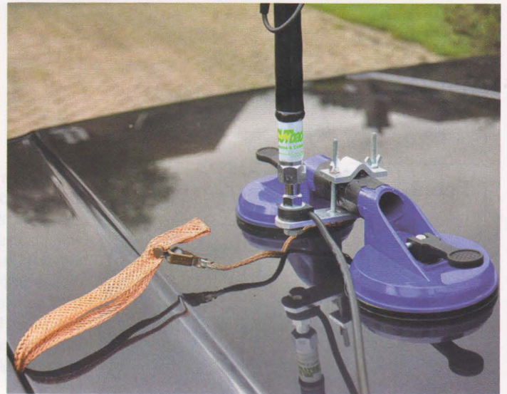
PHOTO 3: The G4UDU suction cup antenna mount. The copper braid earth strap was essential.
