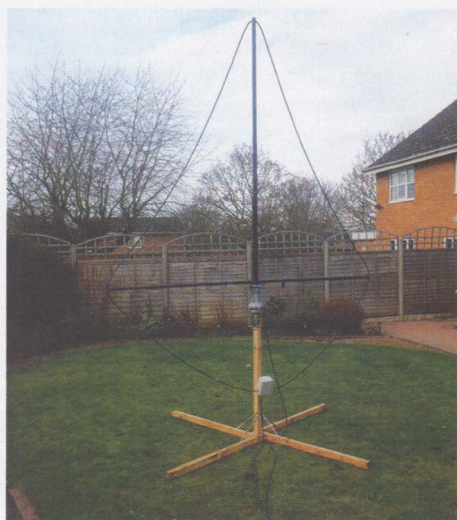
PHOTO 3: G4MKP's 160m receive loop, which "works great on 80m too".
