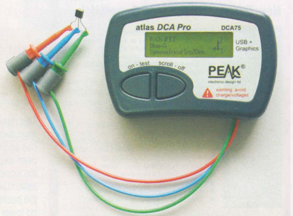
PHOTO 1: The DCA Pro correctly identified this randomly-chosen component as a P channel FET, and even identified the gate lead (see text).
