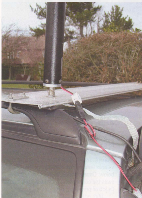
PHOTO 1: A metal plate fixed to a roof rack, which makes a reasonable base for a HF antenna mount. Note the earth braiding strap connected to a point by the tailgate hinge.
