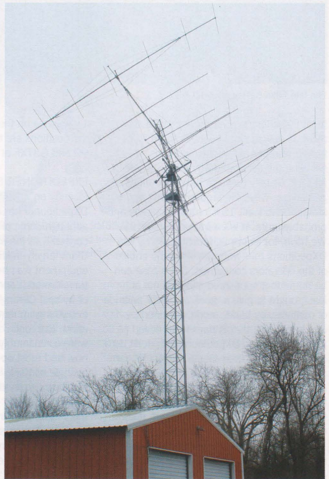
PHOTO 1: The 4 x 8 element Yagi array for 6m and 8 x 18 element Yagi array for 222MHz belonging to Gerald, K5GW. Photo: K5GW.
