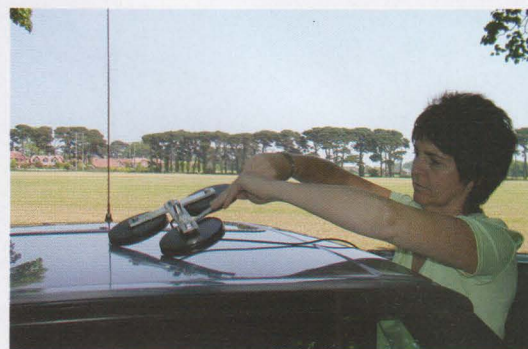
PHOTO 2: A three-magnet antenna mount being removed from the roof of a vehicle using a spanner as a lever.
