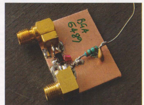
PHOTO 2: BGA6489 test rig.
