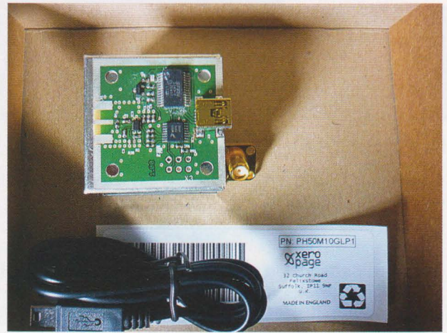
PHOTO 1: The G7OCD USB power sensor from Xeropage (photo: G4BAO).
