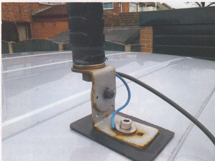
PHOTO 5: G4HJU Mobile antenna mount on the roof of a VW Caddy.
