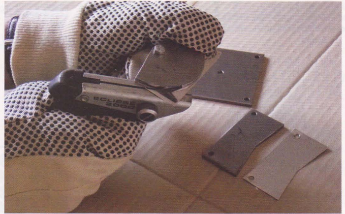
PHOTO 4: Using a pattern to cut out a rotor vane.
