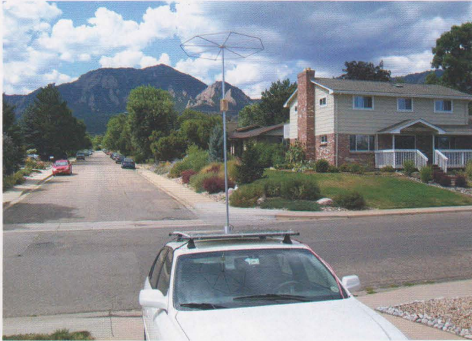
PHOTO 3: The WOIVJ mobile antenna with separate ground plane
