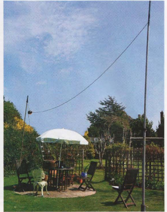
PHOTO 1: An inverted L CFR dipole setup. The feedpoint is located in the top right hand corner where the coax is fixed to the vertical section.
