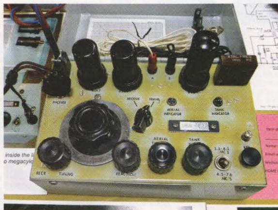
A fine replica Paraset 'spy' transceiver built by Bob Kellogg, AE4IC.
