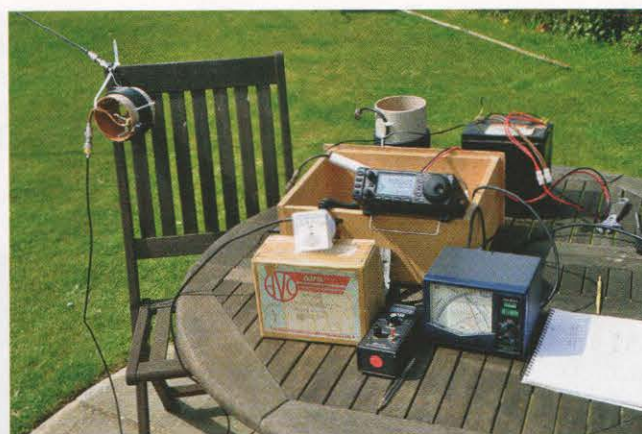
PHOTO 2: Test set up to compare the current variations relative to SWR on a CFR antenna.
