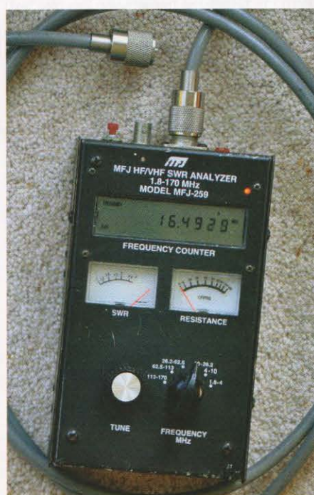
PHOTO 3: MFJ-259 being used to measuring the electrical quarter wavelength of a length of coax.
