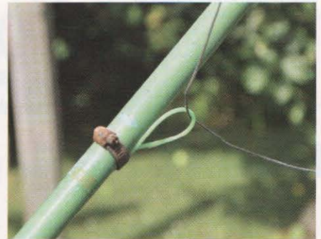
PHOTO 7: Improved method of fixing non-insulated wire elements to the element supports using jubilee clips (hose clamps) and strimmer cord.
