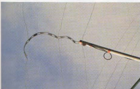
PHOTO 6: Improved method of connecting the coax to the multiband driven elements using 450Ω ladder line and soldering the connections.
