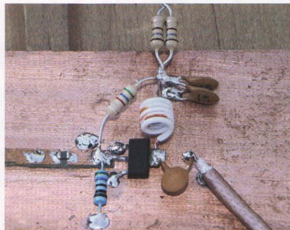
PHOTO 3: Prototype driver stage based on a BFG135.
