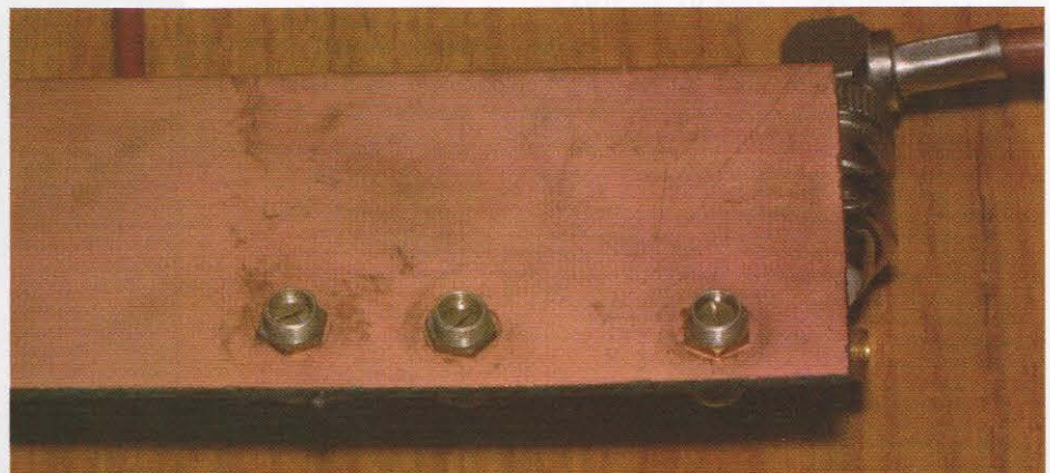
PHOTO 5: Back of the UHF receive converter showing the capacitor mounts and adjusting screws.
