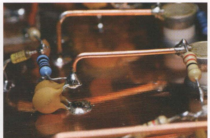
PHOTO 3: How L3 is cut short to allow room for the decoupling capacitors.
