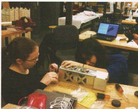
Students build a 3U CubeSat. Image courtesy NASA.
