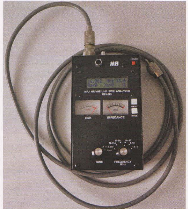
PHOTO 1: An MFJ-269 being used to measure the resonance of an open circuit length of coax. Originally an MFJ-259 was used, which can only measure the Rx component of impedance.
