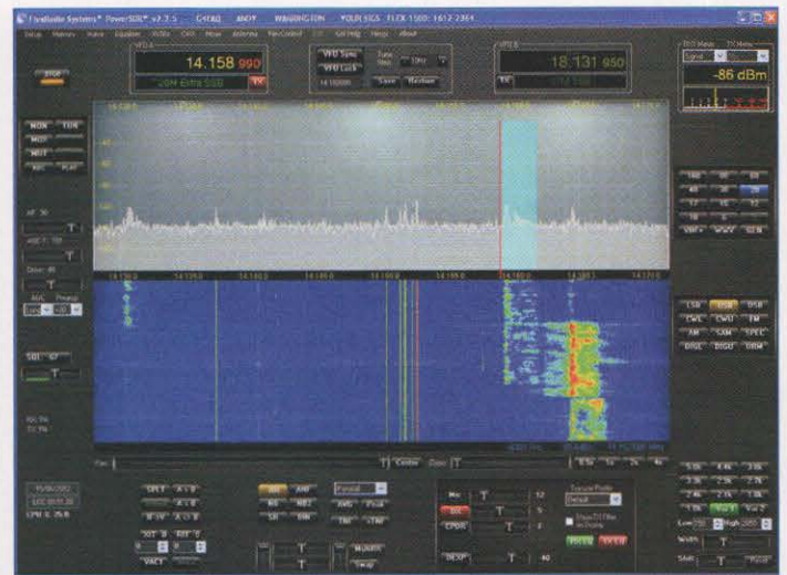
Figure 6: Splattering interferes with VK signals.
