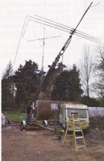
The DESpole manages to fit 14MHz into just 6.2m.
