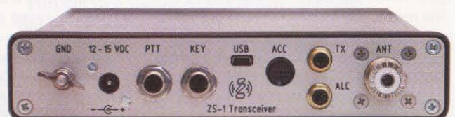
PHOTO 2: Zeus ZS-1 interconnections on the rear panel.
