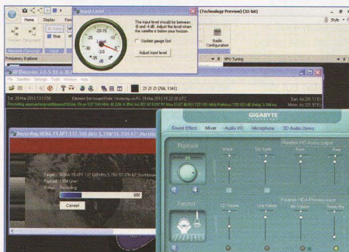
FIGURE 6: NOAA19 weather satellite received using SDR Console 2 and decoded using APTDecoder .
