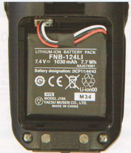
The lithium ion battery pack is different from many handhelds and connects via a flying lead and plug.
