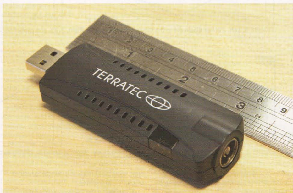
PHOTO 1: A common DVB-T USB dongle, usually available for about £10 on eBay.
