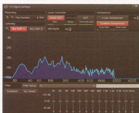
FIGURE 4: The ZS-1 transmit audio processing panel.
