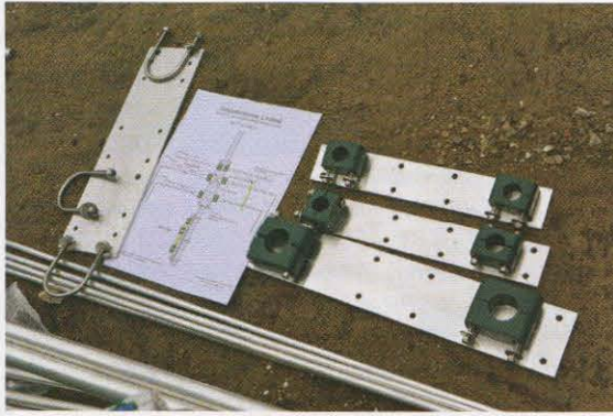
First job is to assemble the centre plates that hold the elements.
