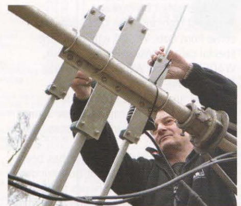
Fitting the coax choke balun.
