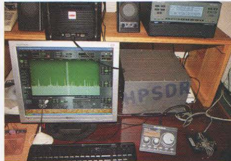
PHOTO 3: VK6VZ HPSDR-based station connected via USB to an old Pentium IV PC with PowerSDR OpenHPSDR software running under Windows XP. Just 8 – 10W from the HPSDR can drive an Expert 1K-FA linear to 400W PEP.
