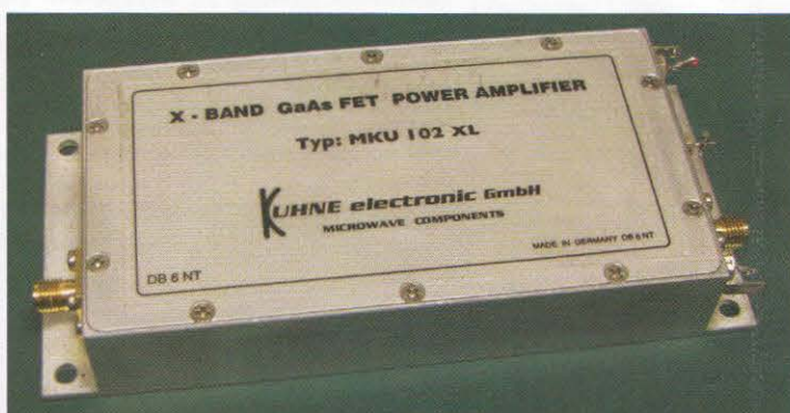
PHOTO 5: A DB6NT 8W RF output power amplifier for 10GHz. Courtesy G4DDK.
