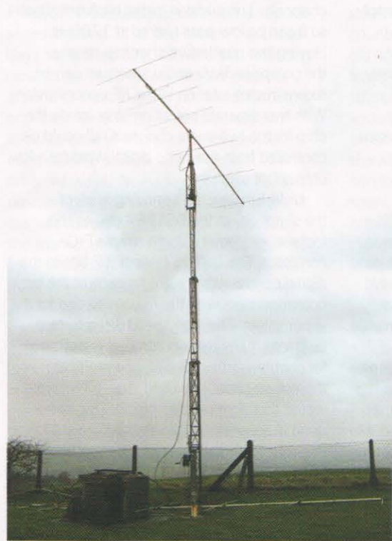
Tiverton SWARC only put up a single 7-ele Yagi for the February session of the 4m Cumulatives due to the weather.
