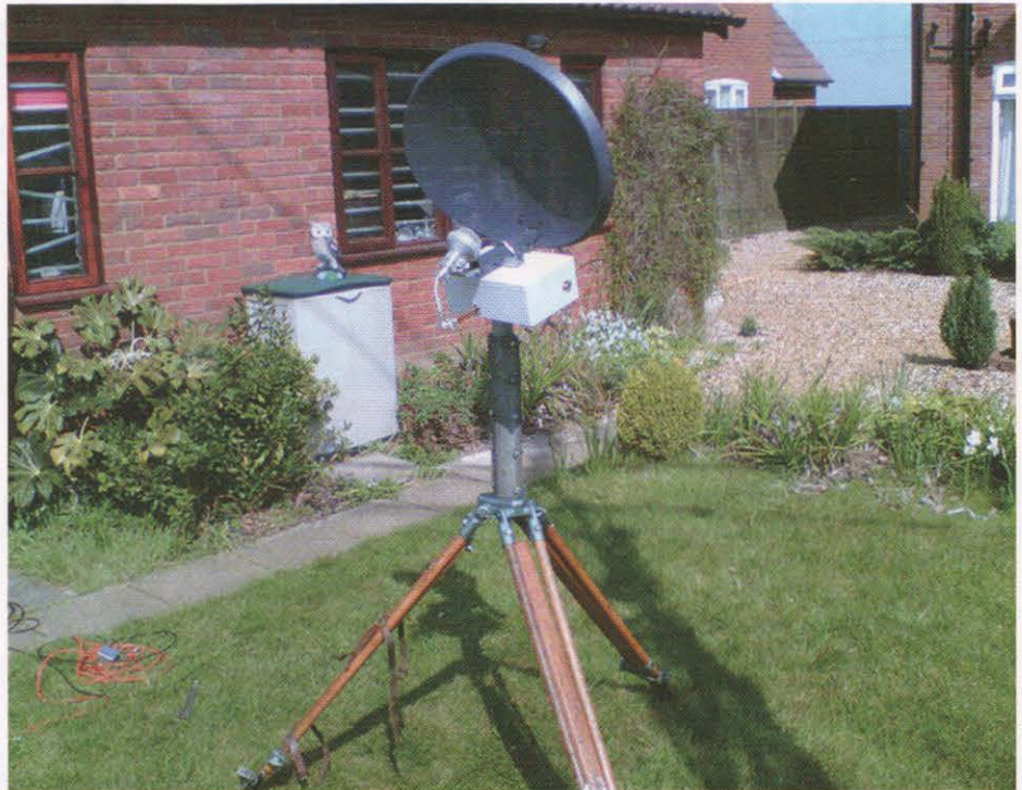
PHOTO 6: A neat microwave portable system using a Sky dish. Courtesy G4BAO.
