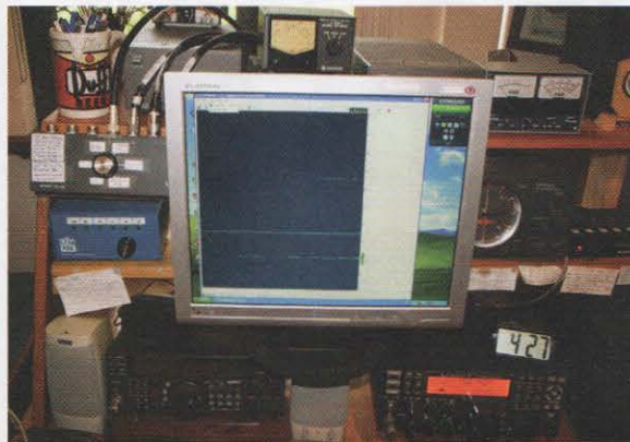
PHOTO 1: VK6VZ Elecraft K3-based station with Softrock SDR running from its 8.215MHz IF into M-Audio D44 pc-based soundcard, old Pentium IV PC and CW Skimmer software running under Windows XP. Note 'blind mode' is selected on CW Skimmer .
