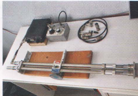
PHOTO 2: Test setup for checking the veracity of the measuring method. The receiver is an FT-817 and a homebrew noise bridge is used as a noise source. An adjustable constant-impedance line trombone is used as the coax under test.
