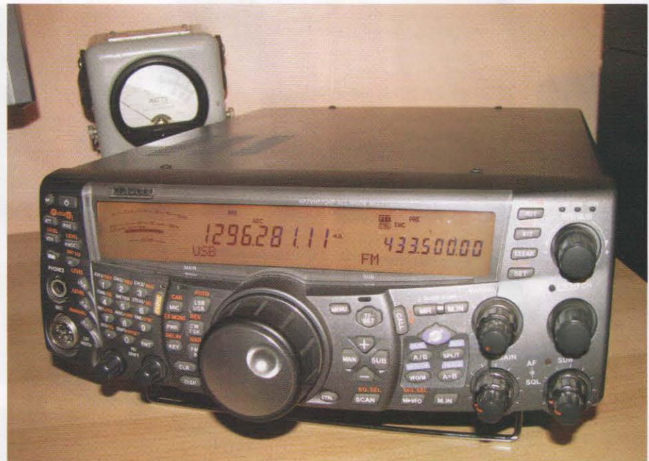
PHOTO 1: TS2000X transceiver that provides 1240MHz to 1300MHz all-mode coverage with 10W RF output. Courtesy G4DDK.
