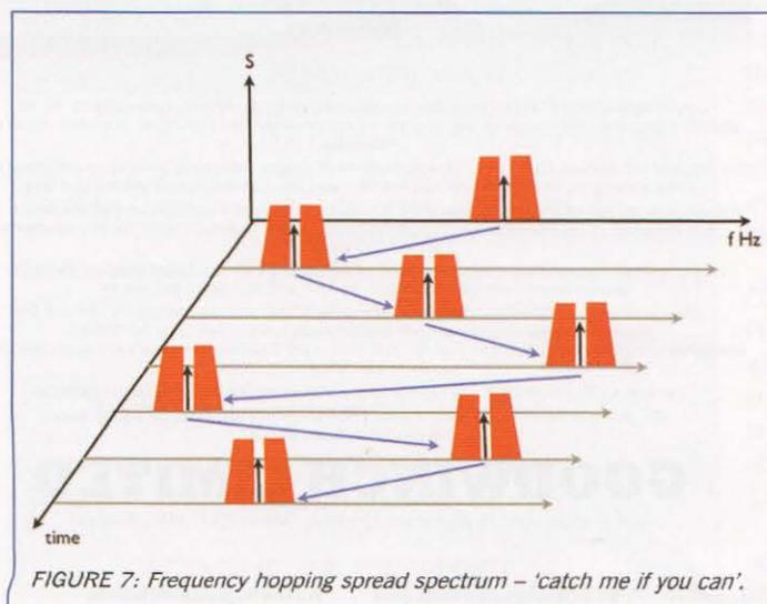
FIGURE 7: Frequency hopping spread spectrum – 'catch me if you can'.
