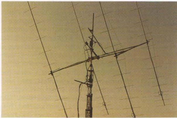
PHOTO 3: How a satellite dish actuator was used by G4SWX to elevate a 4 Yagi antenna system.
