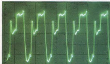
FIGURE 2: OCXO into a high impedance load through 3.2m of coax, showing the enhancement of harmonics due to the different impedances.
