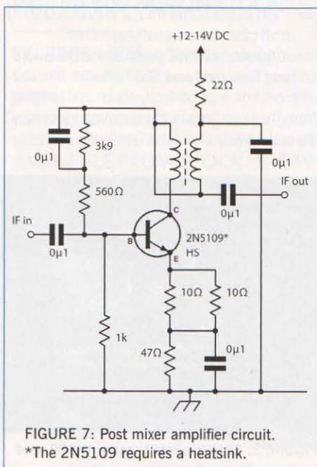
FIGURE 7: Post mixer amplifier circuit.
