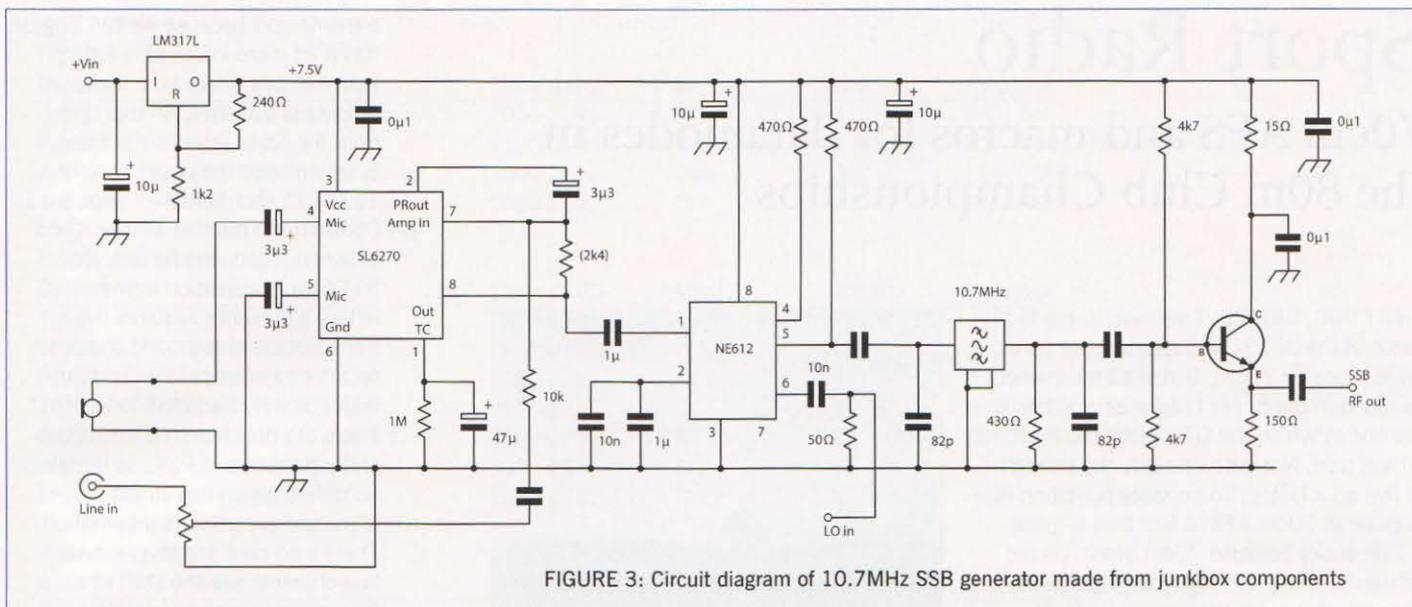
FIGURE 3: Circuit diagram of 10.7MHz SSB generator made from junkbox components
