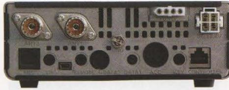
IC-7100 main unit connectors on the rear panel.
