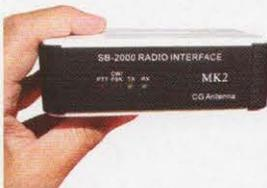
New from CG, the SB-2000Mk11 is an updated version of the original. The unit now supports 2 serial ports allowing you to have one reserved for CAT/CI-V rig control, the other for data operation. It also supports faster speed rate for CAT & CI-V, up to 19200bps.
