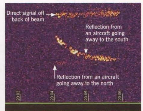
FIGURE 3: 50MHz aircraft scatter WSPR used on the north / south corridor.
