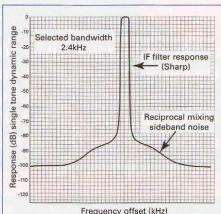
FIGURE 1: IC-7100 effective selectivity curve on USB.
