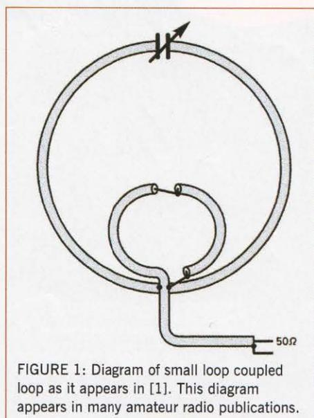
FIGURE 1: Diagram of small loop coupled loop as it appears in [1]. This diagram appears in many amateur radio publications.
