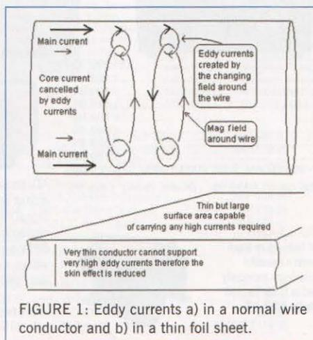
FIGURE 1: Eddy currents a) in a normal wire conductor and b) in a thin foil sheet.
