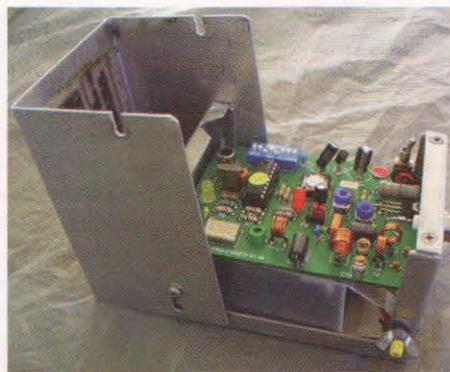
**PHOTO 1:** A typical 2m ARDF transmitter by G3ZOI, pictured with the cover open. The RF strip is along the side nearest the camera. A PIC microprocessor chip (back left) takes care of all the timing and synchronising of the transmitter.
