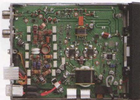
IC-7100 underneath the top cover showing transmitter PA and output filters.
