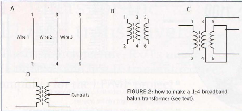
FIGURE 2: how to make a 1:4 broadband balun transformer (see text).
