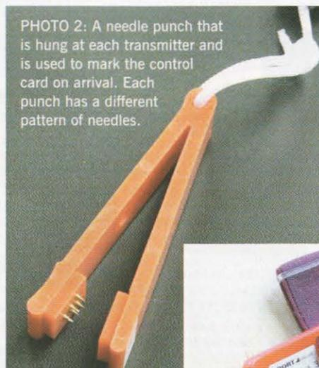
PHOTO 2: A needle punch that is hung at each transmitter and is used to mark the control card on arrival. Each punch has a different pattern of needles.
