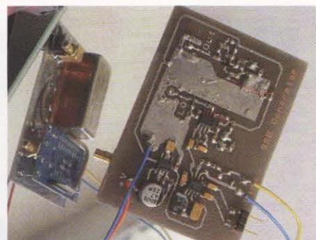
PHOTO 1: The finished SSB generator PCB with the blue eBay DDS module and metallic SSB filter mounted on the top side (seen in mirror) and all other components on the underside.
