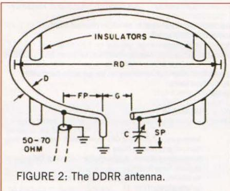
FIGURE 2: The DDDR antenna.
