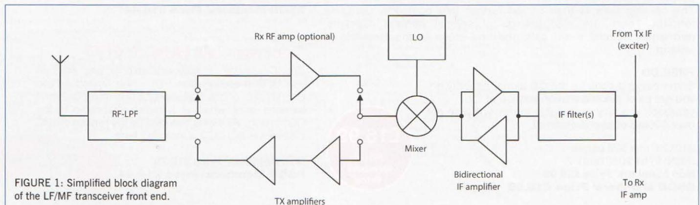
FIGURE 1: Simplified block diagram of the LF/MF transceiver front end.
