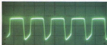
FIGURE 1: OCXO output into a 50Ω load.
