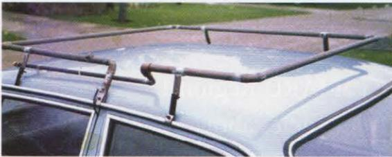
PHOTO 2: An experimental DDDR mobile roof rack antenna for 14MHz. Tuning is accomplished by altering the length of the element end near the vehicle roof.
