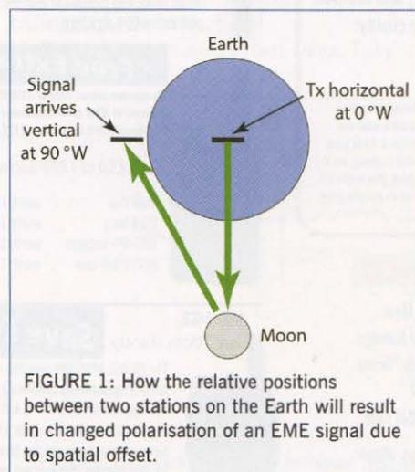
**FIGURE 1:** How the relative positions between two stations on the Earth will result in changed polarisation of an EME signal due to spatial offset.
