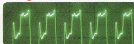
Random cable lengths can do odd things to clock signals
