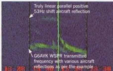
FIGURE 1: 50MHz aircraft reflections on the WSPR screen.
