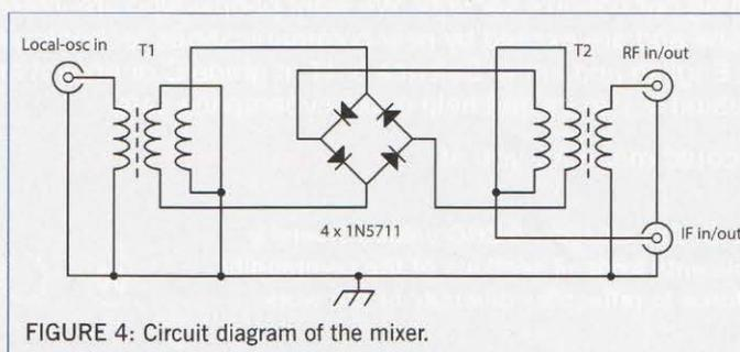
FIGURE 4: Circuit diagram of the mixer.
