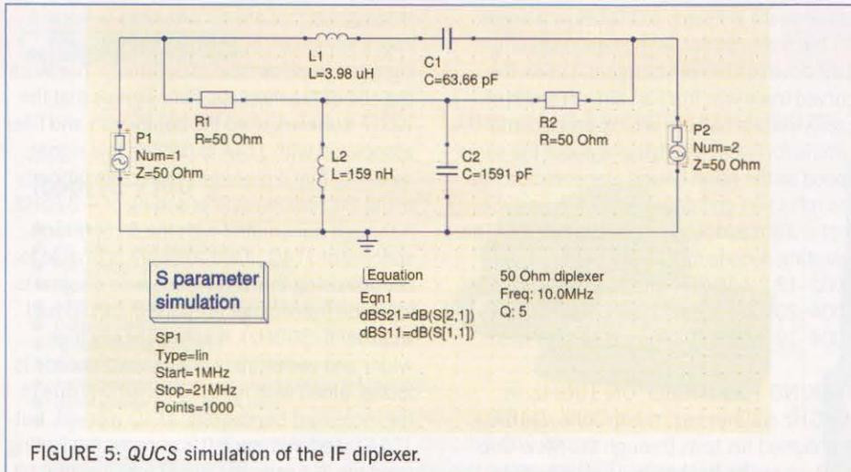
FIGURE 5: QUCS simulation of the IF diplexer.
