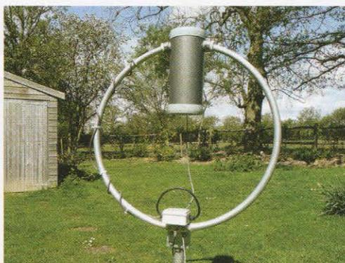
PHOTO 1: The AMA3 0.9m loop antenna used by G4LHZ for experimental measurements. The small loop and wrap wire gamma are under test
