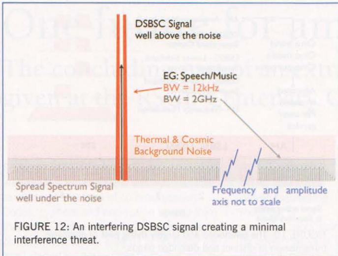
FIGURE 12: An interfering DSBSC signal creating a minimal interference threat.
