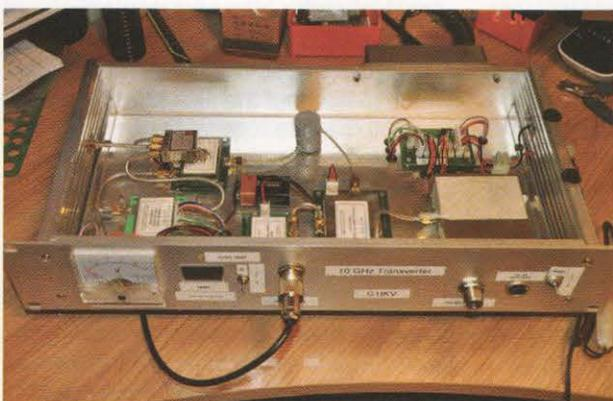
PHOTO 2: The G3VVB prizewinning 10GHz transverter built by G1IKV. Photo: G1IKV.
