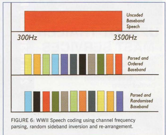
FIGURE 6: WWII Speech coding using channel frequency parsing, random sideband inversion and re-arrangement.
