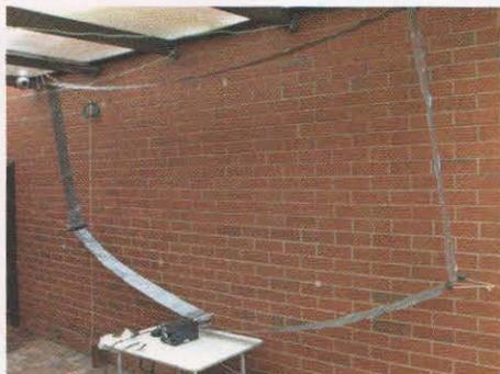
PHOTO 1: A prototype loop antenna fabricated from aluminium foil. Note how its suspension points are well isolated from their surroundings.
