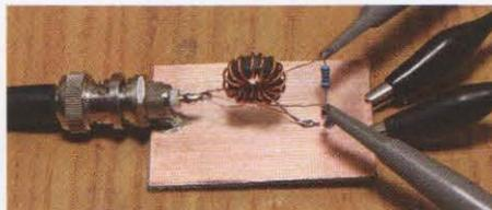
PHOTO 1: Testing the 1:4 broadband balun transformer.
