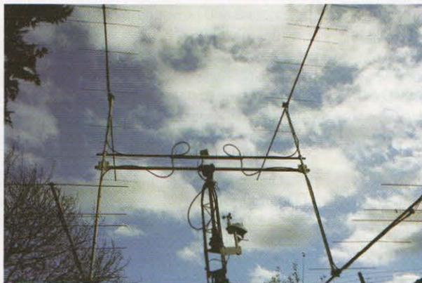
PHOTO 2: 'H frame' in use at G4ZTR supporting a four I0JXX Yagi array.
