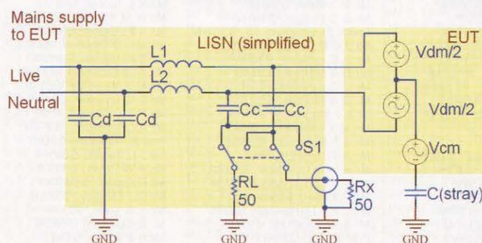
FIGURE 1: Mains conducted emission test using a LISN.
