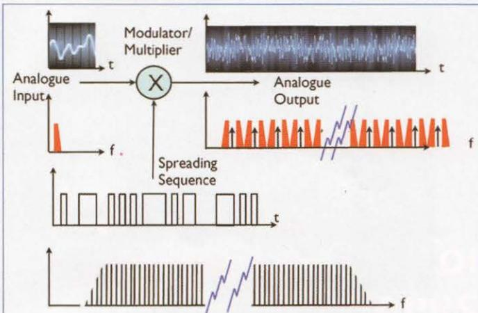
FIGURE 9: Frequency spreading analogue SSB.
