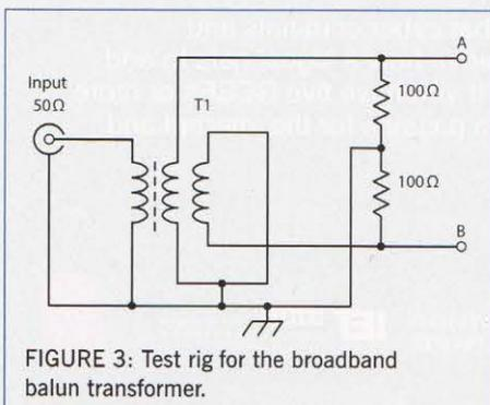
FIGURE 3: Test rig for the broadband balun transformer.
