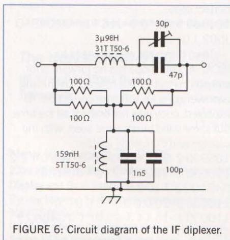
FIGURE 6: Circuit diagram of the IF diplexer.
