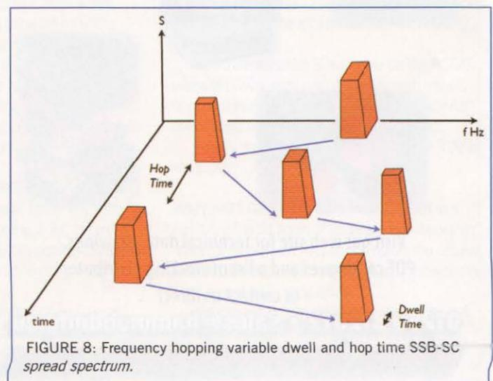
FIGURE 8: Frequency hopping variable dwell and hop time SSB-SC spread spectrum.
