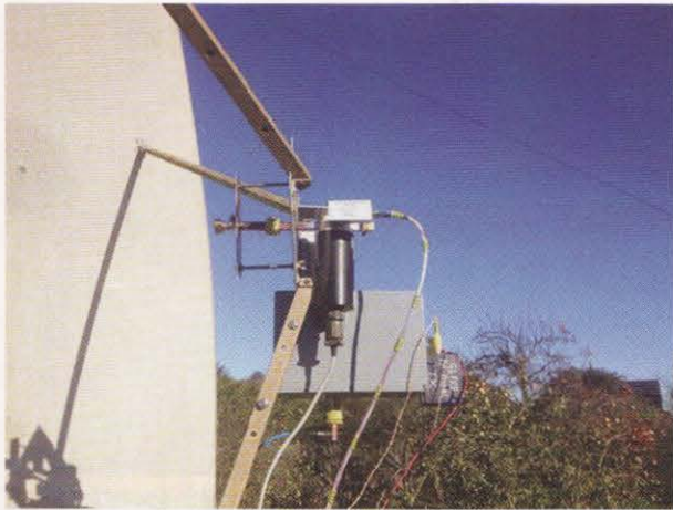
PHOTO 2: 24GHz Feed, preamp WG22 switch and 10W SSPA at G3WDG. Photo: G3WDG.
