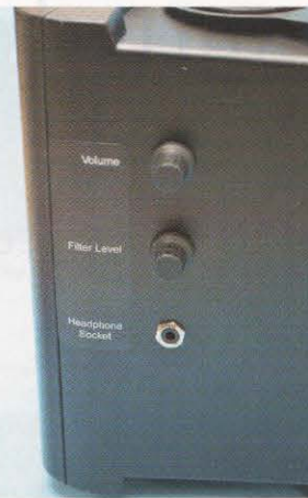
The rear connectors on the bhi DESKTOP speaker.
