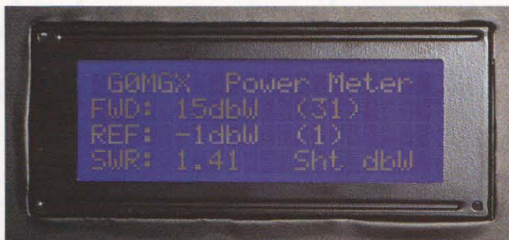
PHOTO 5: Close-up of the LCD showing a VSWR of 1.4:1.
