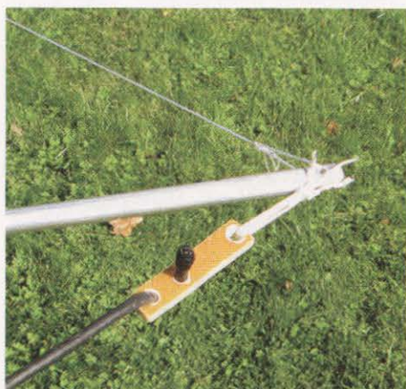
PHOTO 2: Close up of the RG59 element ends and supports.
