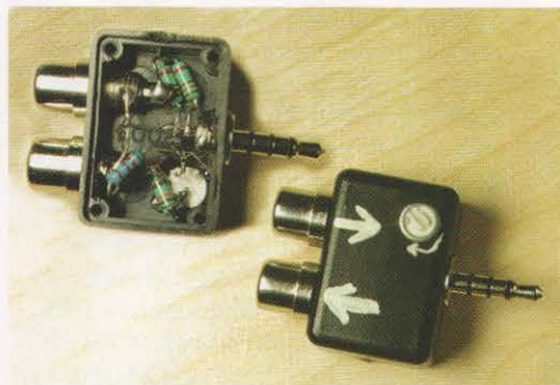
PHOTO 2: The notebook interface module of Figure 1 built into a self-contained plug-in module.
