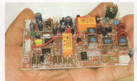
Indonesian SSB transceiver kit from Blekok QRP.
