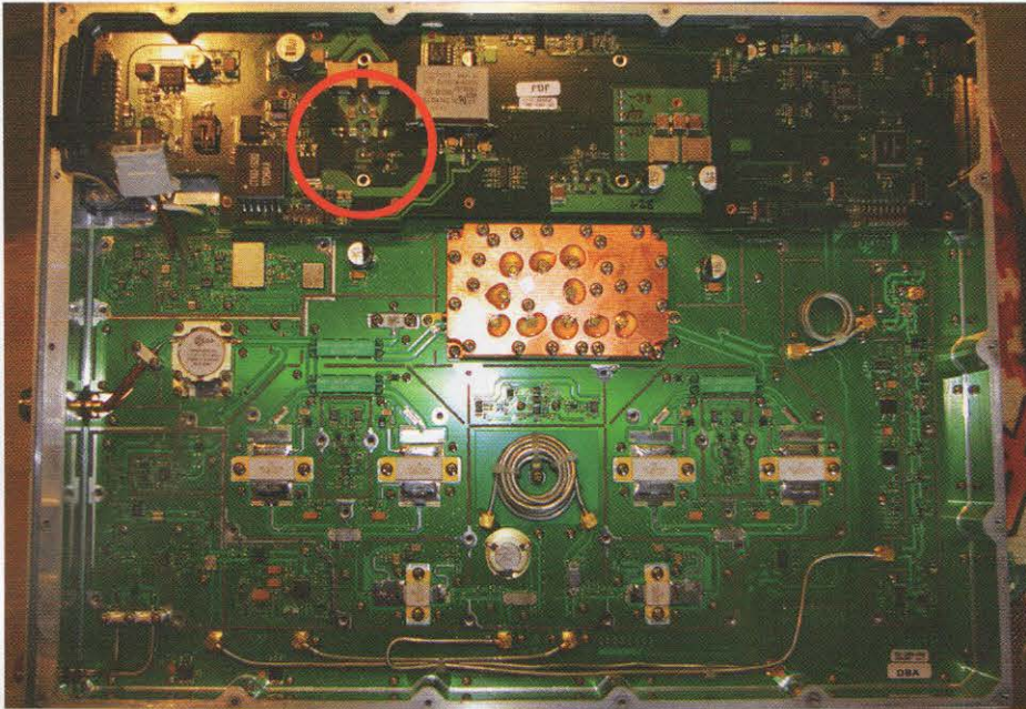
PHOTO 3: Interior of the REMEC amplifier once all the casing and shielding has been stripped. The red circle indicates the area shown in Photo 4.
