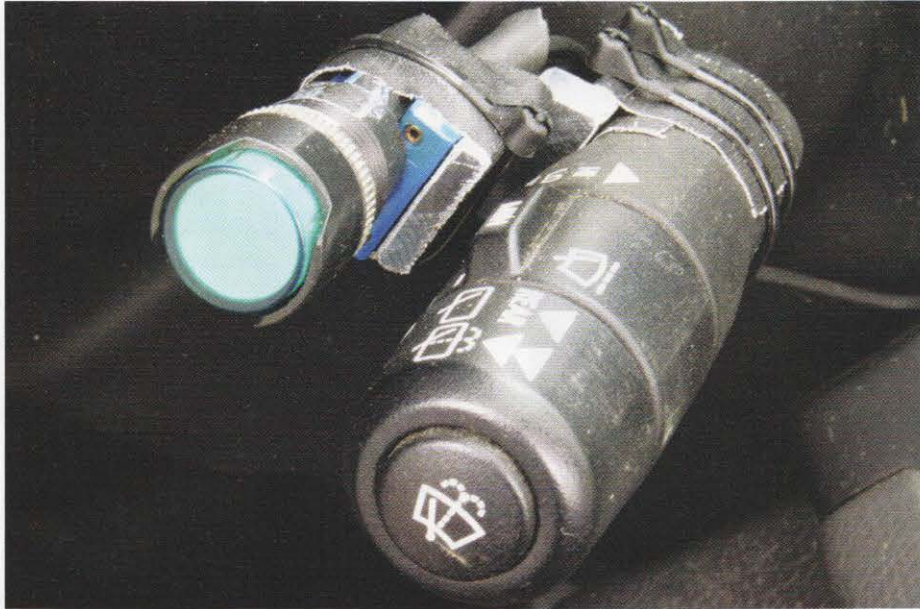
PHOTO 2: Momentary PTT switch attached to one of the steering column stalks.
