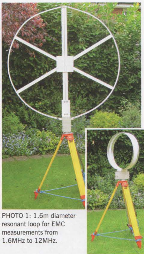
PHOTO 2: 0.6m diameter resonant loop for EMC measurements from 3.5MHz to 30MHz.
