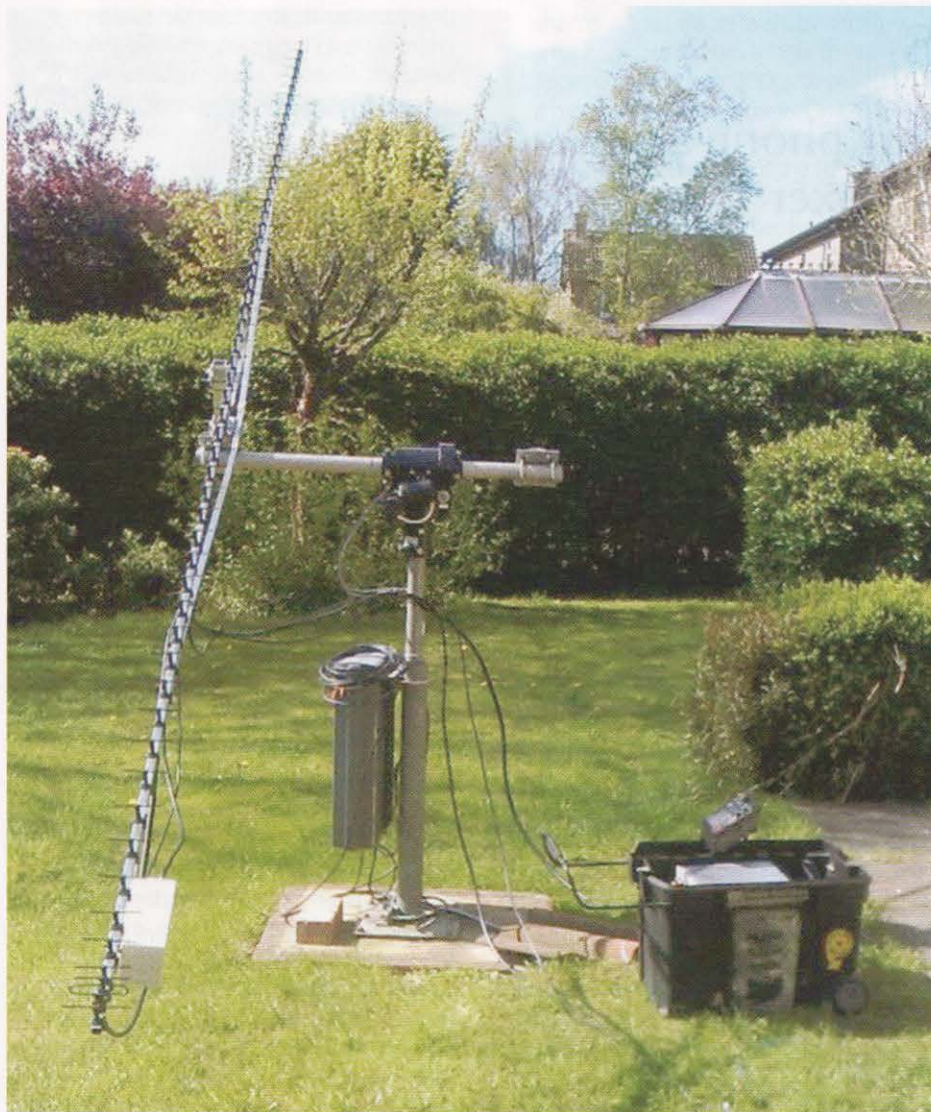
PHOTO 2: The 55-ele Yagi and 'EME in a toolbox' for GS3PYE/P.
