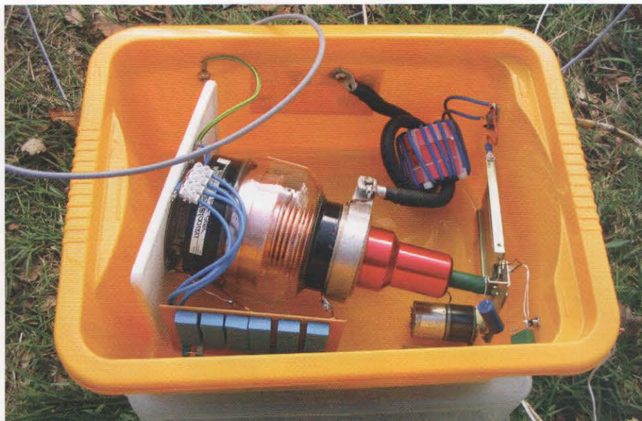
PHOTO 7: Transmitting loop tuning and coupling box.
