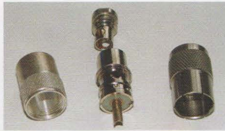
PHOTO 1: PL-259 coax plug components. Centre: plug body for RG213-type cable. Top: reducer for RG58-type cable. Left: screw coupler. On the right is a quick-fit (push-on) PL259 adapter, very useful when experimenting with antennas. Similar temporary push-on connectors are available for a variety of other plug types including SMA.
