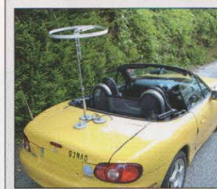
Cover image: The Lambda Loop horizontally polarised 2m mobile antenna by G3NAQ.
