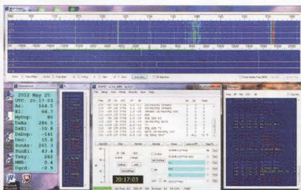
FIGURE 6: MAP65 software from K1JT in operation. This includes a 60+kHz wideband waterfall display at the top and a QSO dialogue box in the middle at the bottom. It displays decodes of other QSOs in progress in addition to the one being made by the operator.
