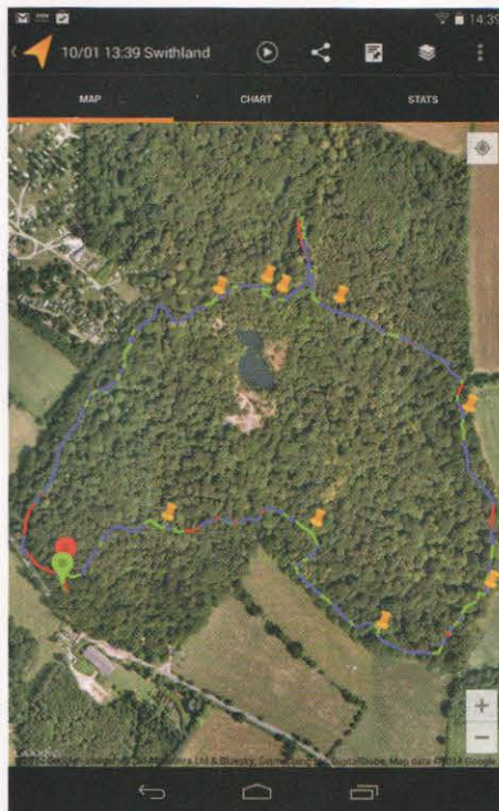
PHOTO 1: Screen grab from My Tracks (Android app). GPS track is coloured according to speed thresholds, which can be adjusted. Pin markers can be added manually or set to specific time (or distance) intervals. If the time interval is set to the normal Tx cycle of 5 minutes it will help to work out which Tx was transmitting.
