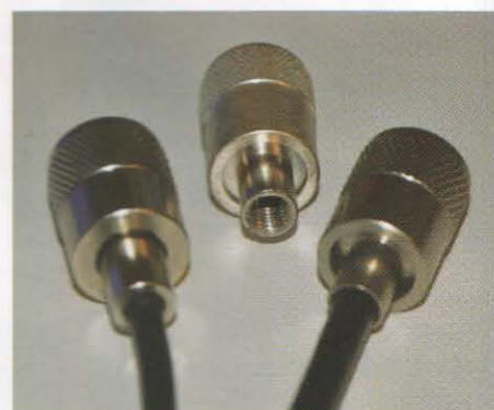
PHOTO 4: Centre, PL259 with built in reducer. Left, connected to RG58 with a 5mm built-in reducer. Right, connected to RG8 Super XX with a built-in 7mm reducer.
