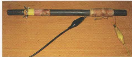
PHOTO 2: A ferrite rod coil can be used to tune a receive aerial.
