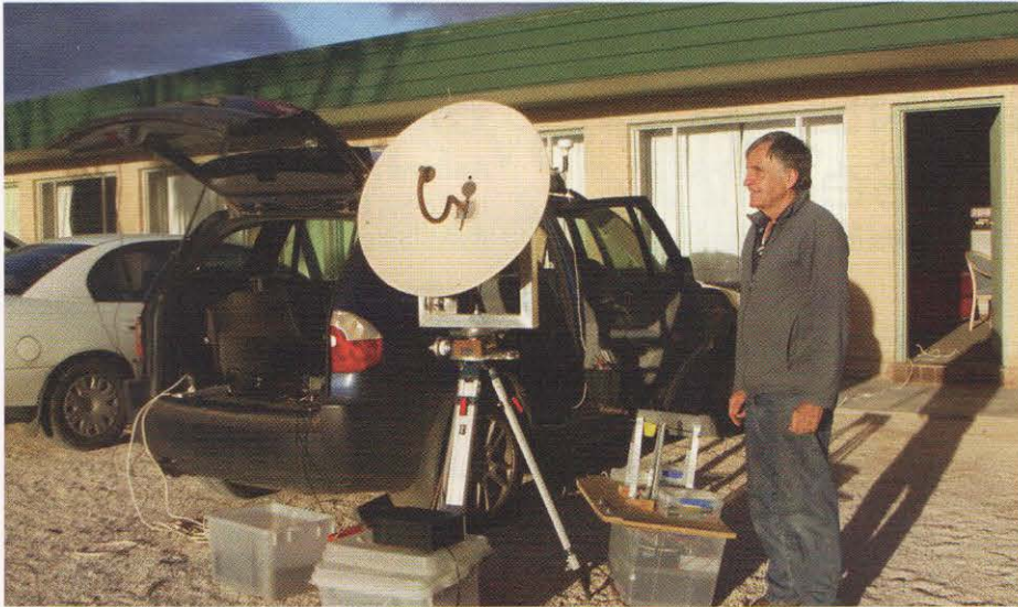
PHOTO 2: VK7MO's portable 10GHz EME system. Photo: VK7MO.
