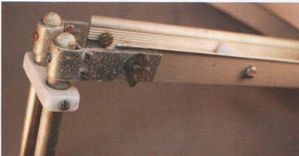
PHOTO 5: Detail of loop connected to bracket.
