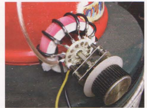
PHOTO 5: A switched matching transformer wound on a large toroid.
