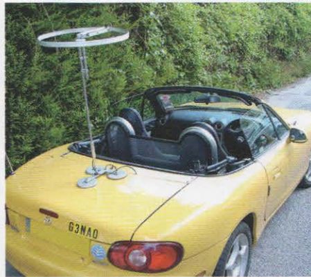
PHOTO 1: The Lambda Loop antenna mounted on my car.
