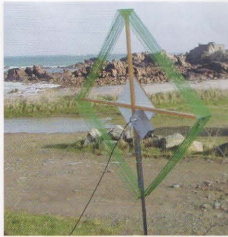
PHOTO 3: Tuned loop for 136kHz in action on a Guernsey beach.
