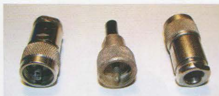
PHOTO 3: Assorted compression sleeve type PL-259s, all variations on the theme of Figure 3.
