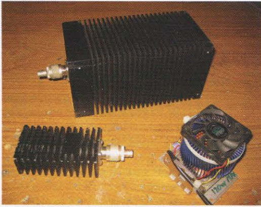
PHOTO 5: Two commercial dummy loads and one homebrewed on a CPU cooler.
