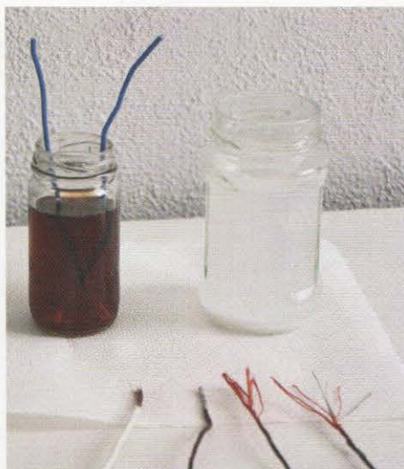
Photo 3: Kitchen cupboard chemistry set used for cleaning tarnished copper wire. Left: vinegar and salt solution, right: bicarbonate of soda (see text).
