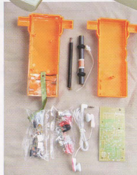
PHOTO 1: The kit as unpacked. Top – case halves, ready wound ferrite rod and telescopic 'sense' antenna. Bottom – bag of through hole components, hardware items, earphones and PCB.
