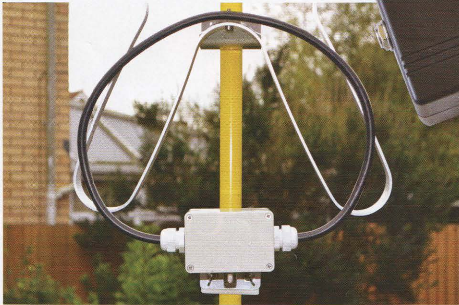
The antenna is fed with a single-turn Faraday loop.
