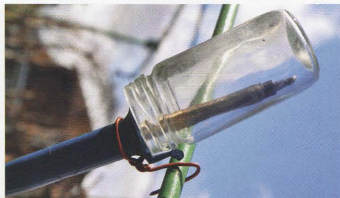
Photo 5: A 25W soldering iron provided with a microclimate to give greater heat.
