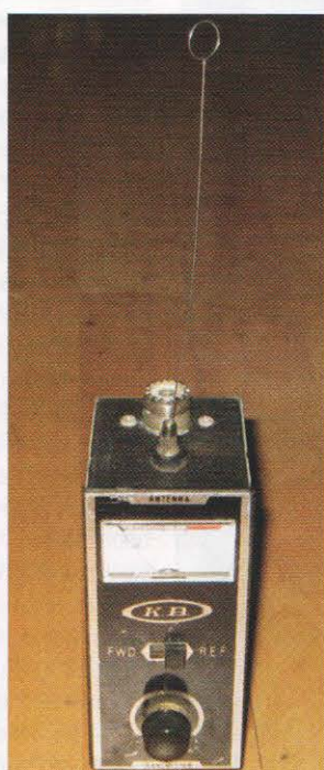
PHOTO 4: A simple field strength meter combined with an SWR bridge.
