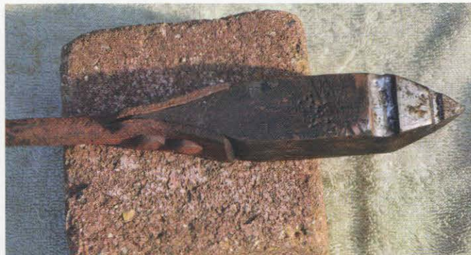
Photo 8: Large copper bit soldering iron. The two channels cut in the tip provide a reservoir for molten solder, making the job of soldering a wire joint easier.
