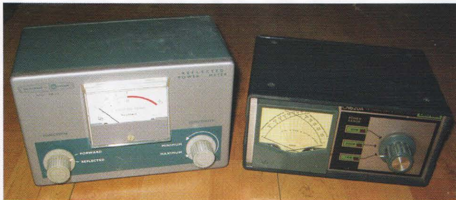
PHOTO 3: A simple forward or reverse meter (left) and a cross-needle power meter (right).
