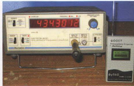
PHOTO 10: A desktop counter and a cheap hand-held counter both measuring the same signal!
