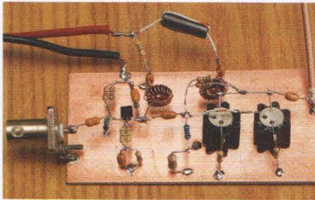
PHOTO 2: Completed driver amplifier. Note that the heatsinks must not touch the ground plane.
