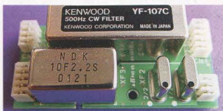
PHOTO 5: Completed filter installation.
