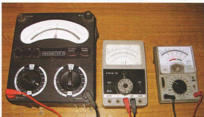
PHOTO 2: Analogue meters including a giant Avo 8, which used to be the 'industry standard' meter.
