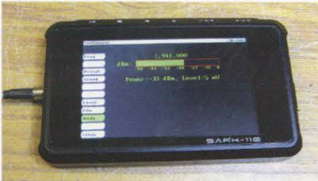
PHOTO 12: Using the Sark-110 analyser as a signal generator.
