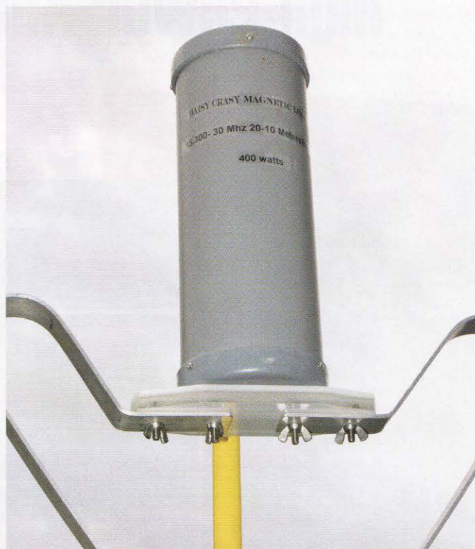
The loop is brought to resonance with a 'butterfly' split stator variable capacitor.
