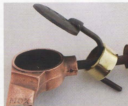
Photo 7: A magnesium oxide heated MOX soldering iron originally used for outdoor antenna work.
