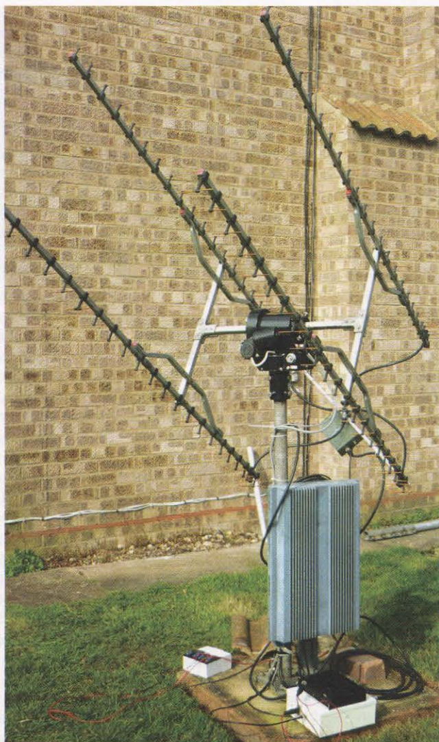
PHOTO 1: Sun noise tests on a 4x23-ele Tonna array at G4BAO.
