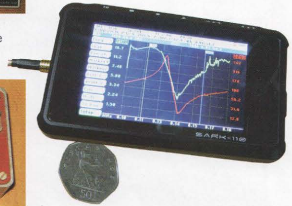
PHOTO 14: The new miniature Sark-110 aerial analyser in action.
