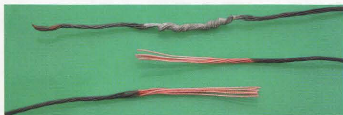
Photo 4: The effect of cleaning weather tarnished copper antenna wire using the chemistry described in the text. Also shown is a soldered joint I made earlier – 10 years earlier – showing how it has stood up to the weather.
