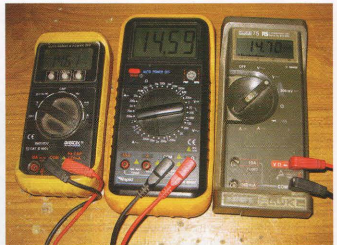
PHOTO 1: A selection of digital meters all measuring the same voltage!
