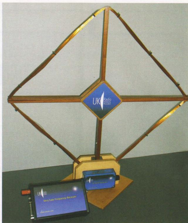
PHOTO 2: Loop antenna and tuneable 12-35kHz VLF receiver from UKRAA. Image courtesy of G4CSD.
