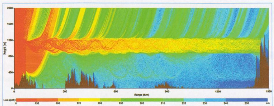
FIGURE 7: Predicted path loss for GMOUSI/P-F2CT/P link at 10GHz using modified refractivity profile from Brest radiosonde data at 1200UTC on 15 September 2012 assuming GMOUSI/P at altitude of 1000m.
