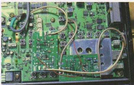
PHOTO 2: Two PATs installed in an FT-897.
