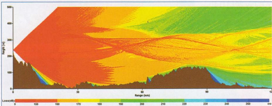
FIGURE 9: Predicted path loss for GB3SEE-G4BAO link at 24GHz using modified refractivity profile from Larkhill radiosonde data at 0600UTC on 10 July 2013
