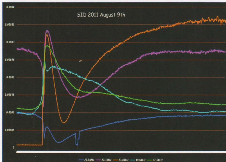
FIGURE 2: The effect of a very strong (X-class) flare on five VLF signals over about five hours. Image courtesy of Mark Edwards.
