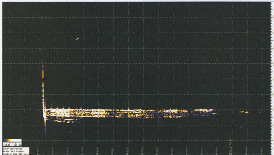
FIGURE 3: The high power signal from GRAVES allows you to watch meteor trails as they disperse with time. Note that the vertical axis shows the Doppler-shifted frequency of individual plasma tubes in the trail. Image courtesy of G4CSD.
