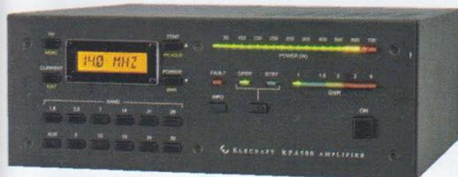
The KPA-500 covers the bands 160m to 6m and delivers 600W with a drive level of around 30W. It can be used with any transceiver and features auto band switching through RF sensing. It has a built in AC supply and is the same size as the K3 transceiver. This is a great solid state design with full protection. No warm up and capable of full QSK switching.
