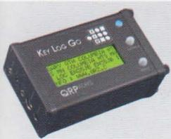
Designed for CW and data operation with the KX3. It can decode CW and data, store messages, and can also extract call signs for automatic logging and phrase insertion. Can also
