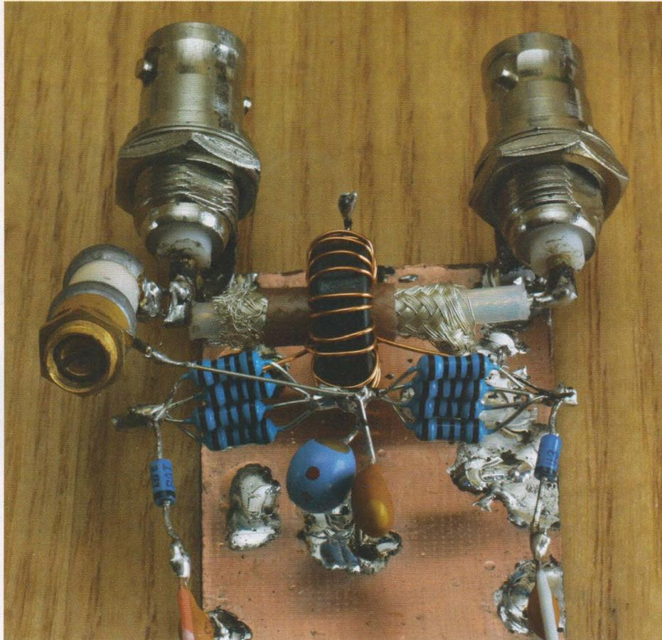
PHOTO 1: This directional coupler may look a bit cobbled-together but it has been tested and found satisfactory at powers of up to 250W from Top Band to 10m.
