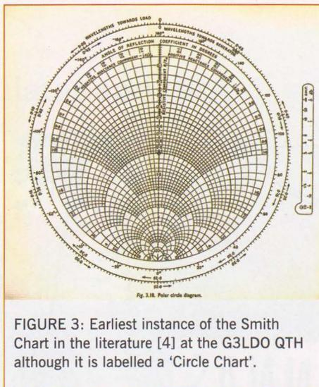
FIGURE 3: Earliest instance of the Smith Chart in the literature [4] at the G3LDO QTH although it is labelled a 'Circle Chart'.
