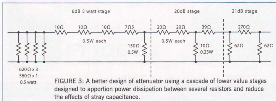
**FIGURE 3: A better design of attenuator using a cascade of lower value stages designed to apportion power dissipation between several resistors and reduce the effects of stray capacitance.**
