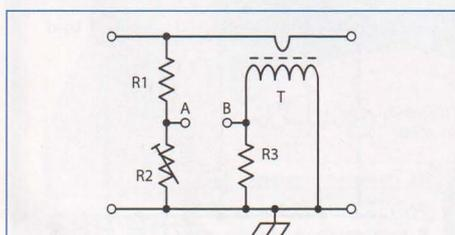
FIGURE 3: Directional coupler based on a current transformer and a resistive divider.
