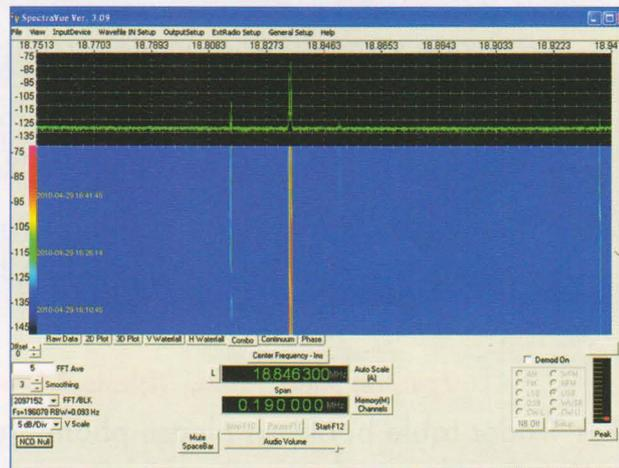
FIGURE 1: Reception of 10GHz beacons using SDR.
