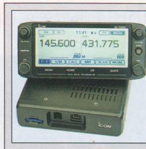
Cover image: The Icom ID-5100 dual band D-Star transceiver.
