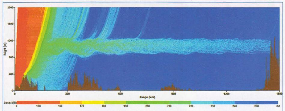
FIGURE 6: Predicted path loss for GMOUSI/P-F2CT/P link at 10GHz using modified refractivity profile from Brest radiosonde data at 1200UTC on 15 September 2012
