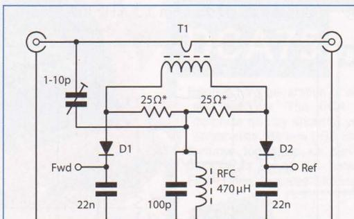
FIGURE 4: Directional coupler with diode detectors providing forward and reflected power outputs.
