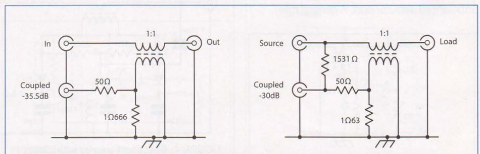
FIGURE 6: (left) RF current sampler based on a 1:1 transformer; (right) a -30dB directional coupler based on the same circuit (see text).
