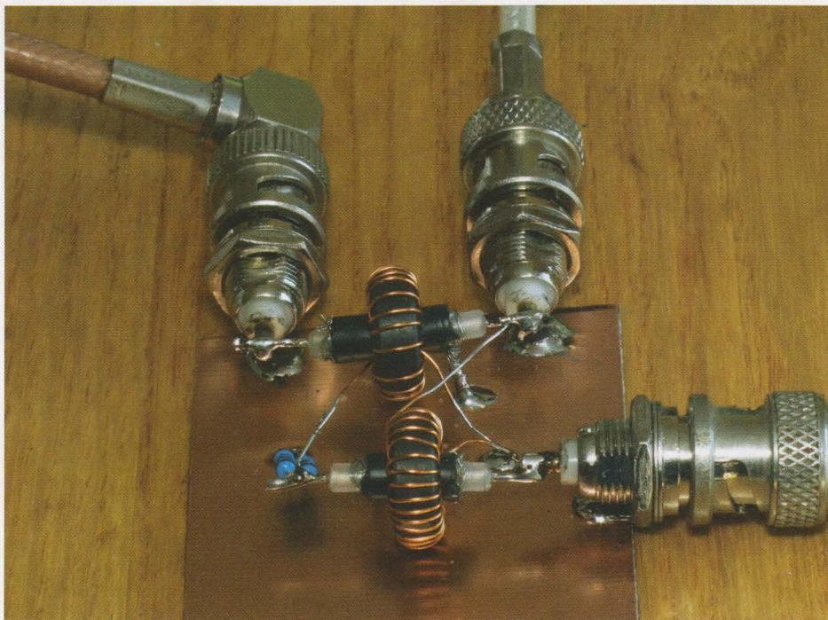
PHOTO 2: Prototype Tandem Match. Note that the coax braids are each earthed at only one end.
