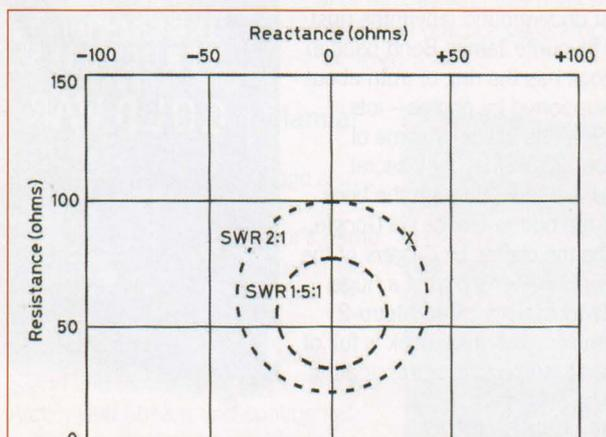
**FIGURE 1:** Cartesian plot of frequency where an impedance of  $R80 + j34$  is marked with an X. The outer dotted circle indicated an SWR of 2:1; the inner circle is 1.5:1.
