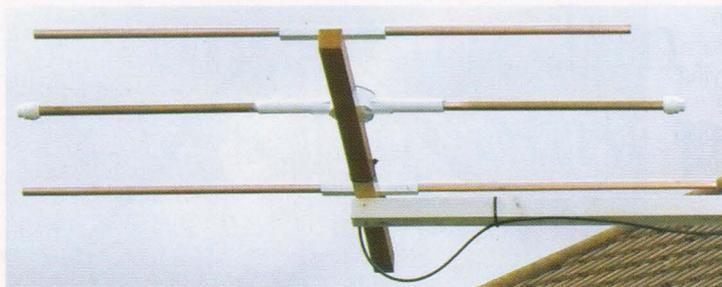
PHOTO 3: Simple 3-element Yagis like this are adequate for meteor scatter experiments.
