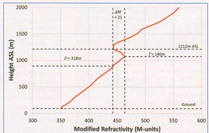
FIGURE 4: Modified refractivity profile for Camborne radiosonde measurements at 1200UTC on 15 September 2012.
