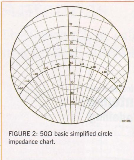
FIGURE 2: 50Ω basic simplified circle impedance chart.
