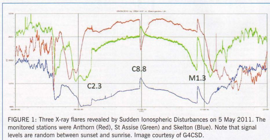
FIGURE 1: Three X-ray flares revealed by Sudden Ionospheric Disturbances on 5 May 2011. The monitored stations were Anthorn (Red), St Assise (Green) and Skelton (Blue). Note that signal levels are random between sunset and sunrise. Image courtesy of G4CSD.
