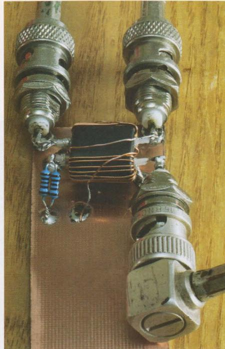
PHOTO 3: A -20dB directional coupler built around a binocular-style ferrite core.
