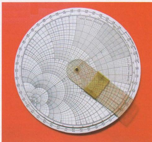
**PHOTO 1:** Smith Chart calculator with rotatable wavelength scale and a number of radially scaled parameters on a centre-pivoted cursor based on [7].
