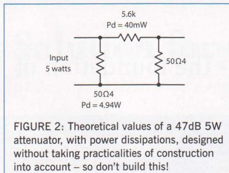
**FIGURE 2: Theoretical values of a 47dB 5W attenuator, with power dissipations, designed without taking practicalities of construction into account – so don't build this!**
