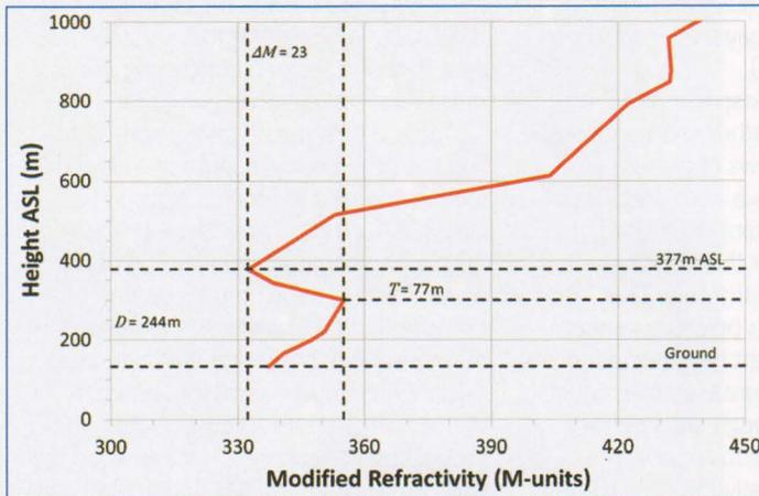
FIGURE 8: Modified refractivity profile for Larkhill radiosonde measurements at 0600UTC on 10 July 2013.
