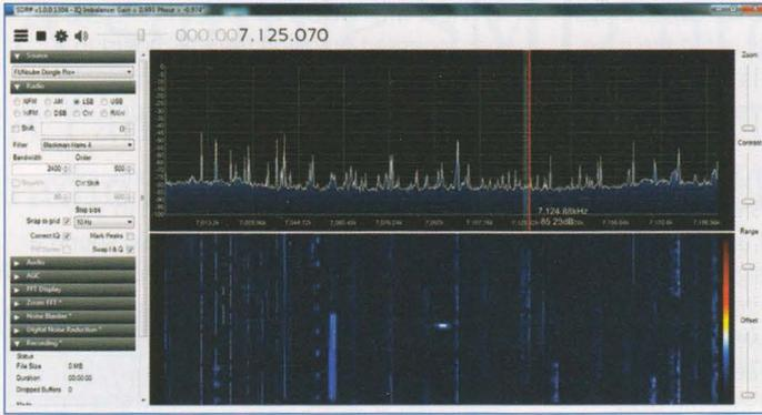
FIGURE 3: 40m band as 2nd Rx function, using a FUNcube Dongle Pro+ and SDR#.
