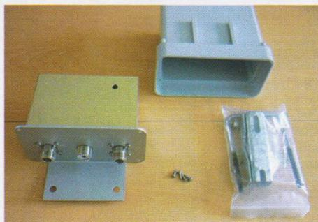
PHOTO 2: The preamp with its waterproof box removed
