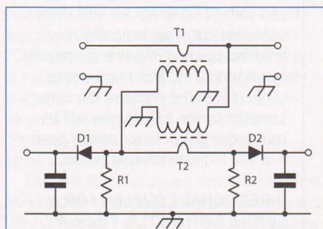
FIGURE 5: The basic Tandem Match circuit.
