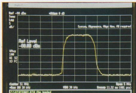
PHOTO 1: The spectrum of a DATV transmission on the 6m band using a symbol rate of 1.1333MS/sec.
