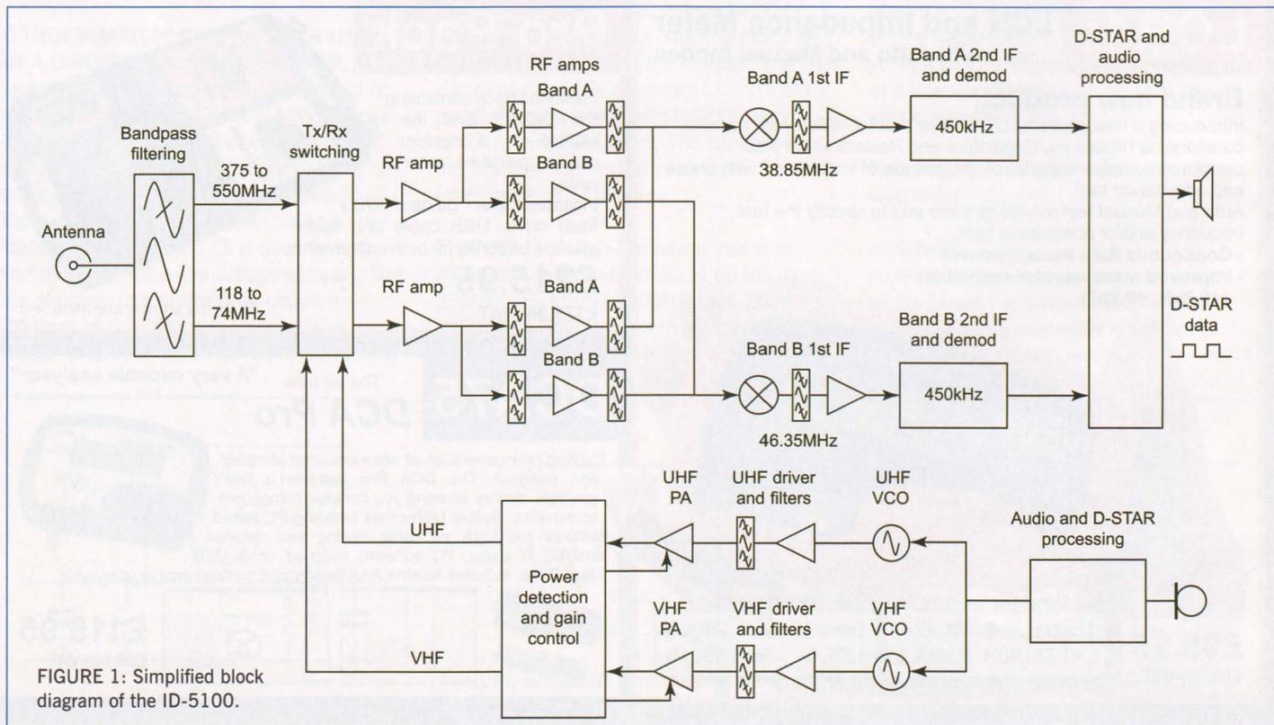
FIGURE 1: Simplified block diagram of the ID-5100.
