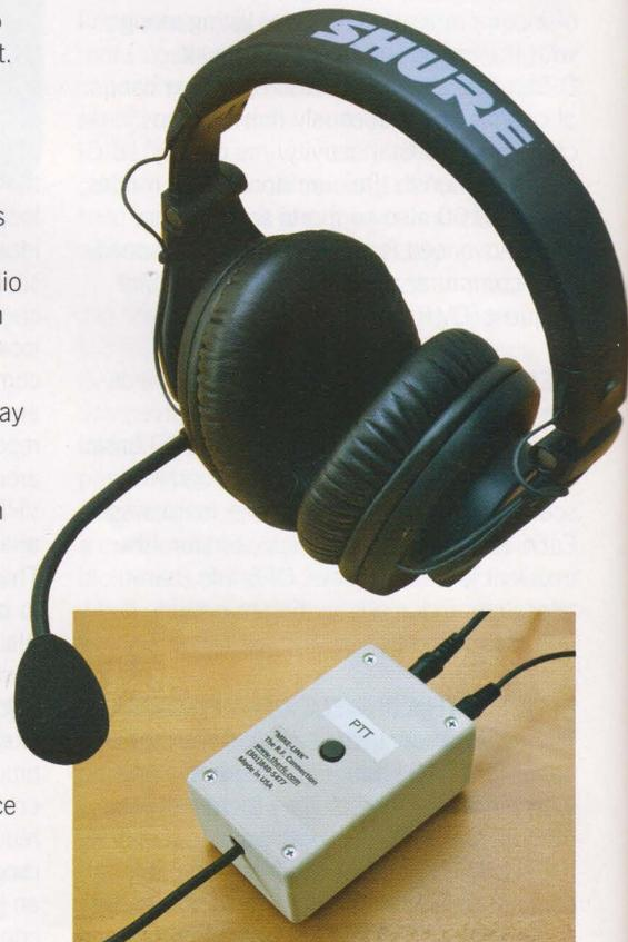
The Mike-Link interface box has a single PTT button in the middle, plus switches on the side.
