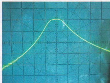
PHOTO 3: Plot of the frequency response on a 50MHz sweep width, vertical axis 10dB/division.
