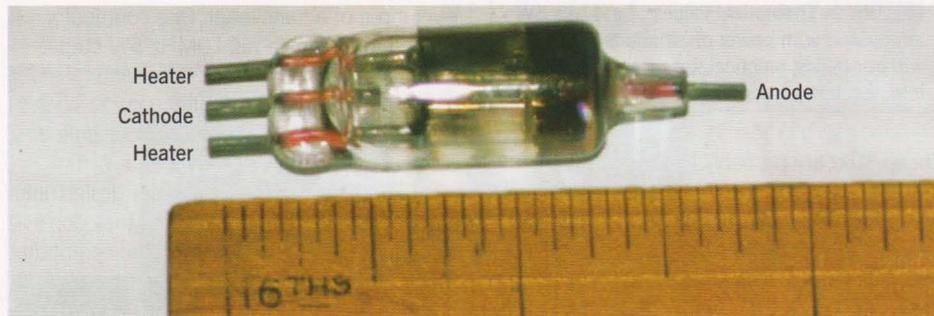
PHOTO 1: Miniature rectifier diode rated at 50V RMS input, 5mA, which uses a 6.3V 150mA heater.
