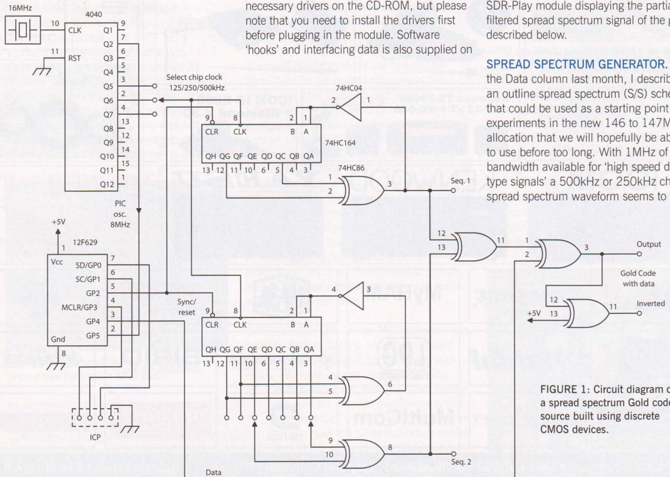
**FIGURE 1:** Circuit diagram of a spread spectrum Gold code source built using discrete CMOS devices.
