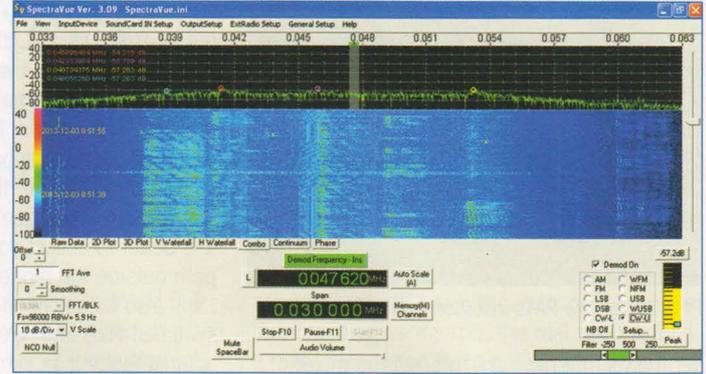
FIGURE 4: 40m band SSB segment as IF tap, with FUNcube Dongle Pro and Spectravue 3.09.
