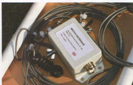
A 4:1 balun of MOCVO's design is added at the feed point.
