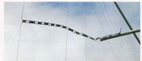
PHOTO 2: Detail of the long stub used to tune the quad on the 20m band. You can probably see where the length of the stub was altered during the tune up process.
