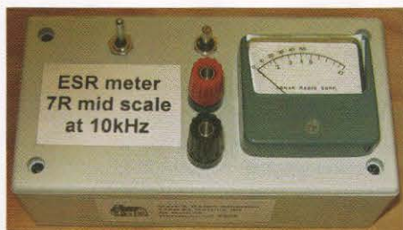
PHOTO 2: My home-made ESR meter, based on instructions found at [1].
