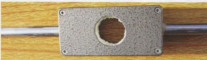
PHOTO 6: Diecast box for the anti windage horizontal rods.
