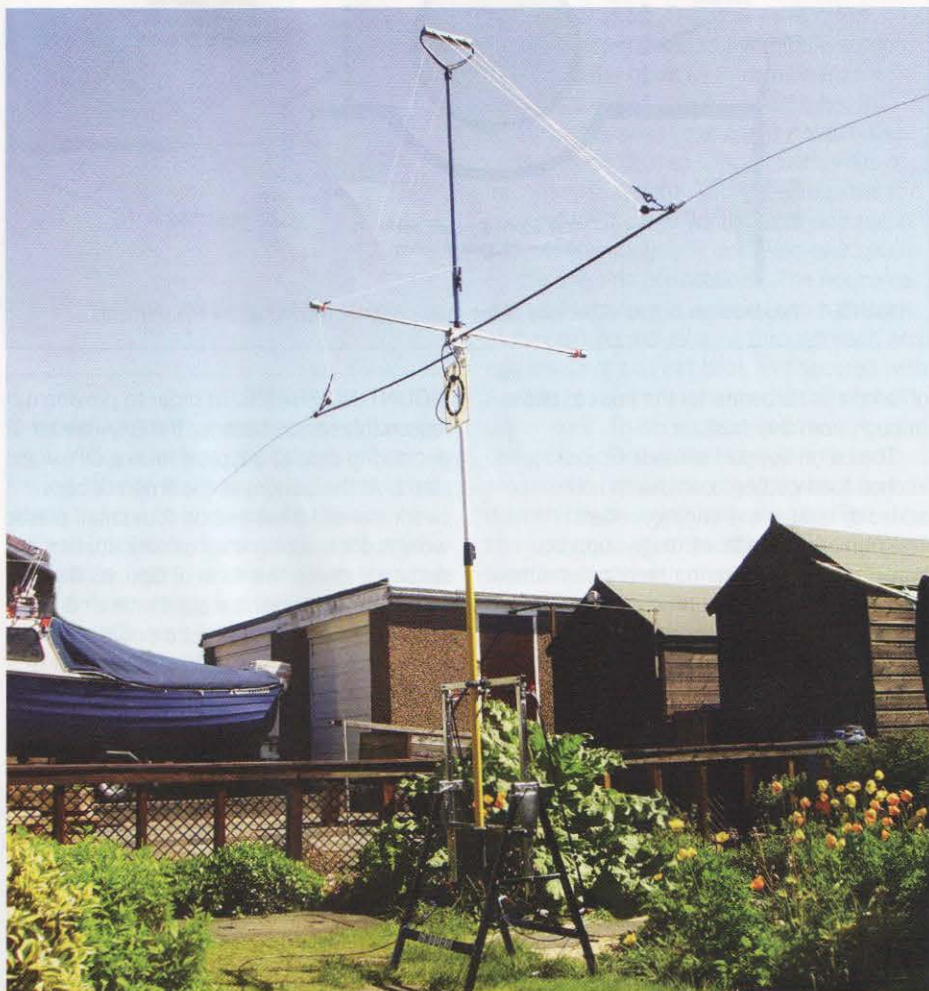
PHOTO 1: General view of the fully erected Sky-Painter portable 40m dipole antenna.
