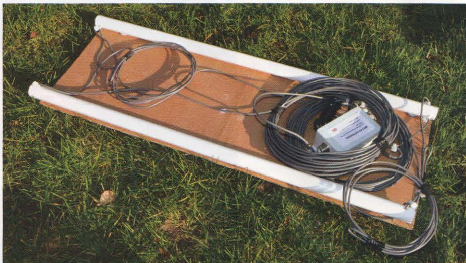
The starting point of the antenna is the classic off centre fed dipole.
