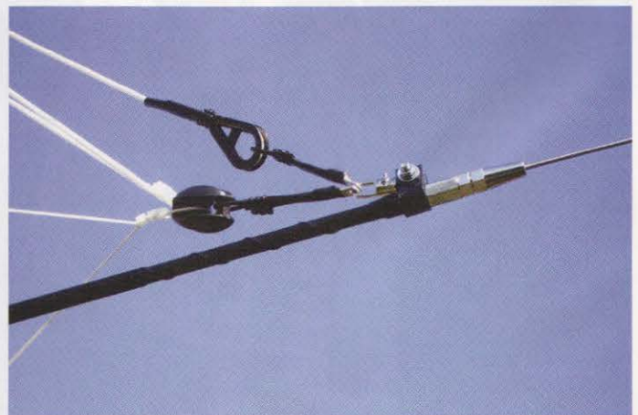
PHOTO 9: How the nylon cords attach to the antenna loading coils.
