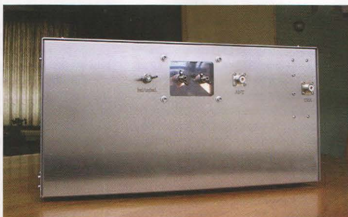
PHOTO 9: The most striking feature of the minimalist rear panel is the clear acrylic insulating sheet that carries the balanced output terminals.
