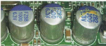
PHOTO 1: The electrolytic capacitor on the right has died and the one in the middle is extremely poorly.
