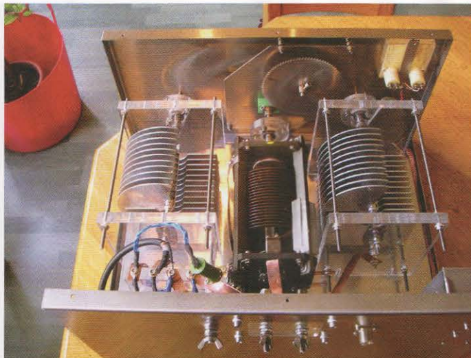
PHOTO 7: Looking towards the front panel. The 6mm thick semi-circular stainless steel counterbalance weights can be seen at the far end of the variable capacitors and the variable inductor is in the middle of the photo.
