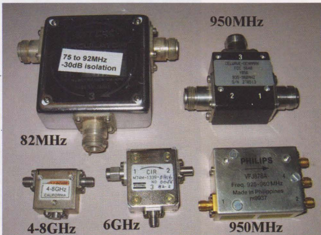
PHOTO 1: Circulators and isolators come in all shapes and sizes – and frequency ranges.
