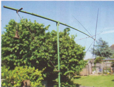
PHOTO 1: Fold-over pipe mast in current use. An additional counterweight is used to ease the raising and lowering of the antenna.
