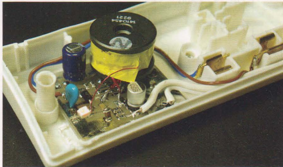
PHOTO 1: 230V DC supply built into low cost 13A two-way adapter block.
