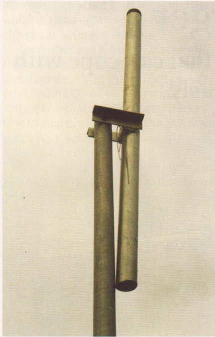
PHOTO 2: Fold-over/rotator mechanism comprising a 90mm (3½in) section of pipe on which two short lengths of angle iron have been welded to make the thrust bearing.
