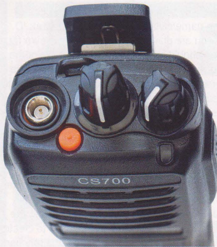
PHOTO 2: The top panel contains the antenna socket, a programmable button, channel & volume controls and a Tx LED. The belt clip is quite sturdy and just visible at the top of the panel is a moulding to take a lanyard.
