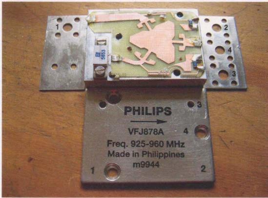
PHOTO 3: Inside the Philips VFJ878A isolator.
