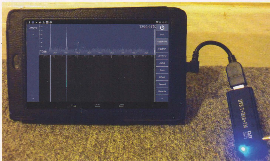
PHOTO 1: An RTL dongle plugged into a Google Nexus tablet computer running SDR Touch and showing some of the spurious signals mentioned in the text.
