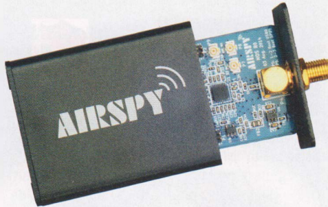
PHOTO 1: The Airspy 12-bit 10MHz bandwidth SDR, designed to complement SDR# and similar software. Image courtesy of www.SecQuest.co.uk
