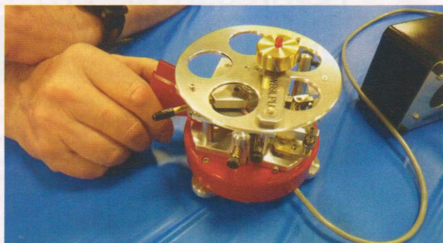
PHOTO 1: The RotoBug employs the rotation of a variable mass to provide the power for the string of automatic dots and the rotation of another variable mass to provide the power for a string of dashes.
