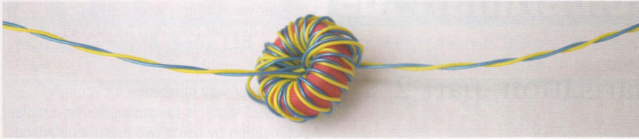
PHOTO 2: A twisted pair common-mode choke wound on a ferrite ring core
