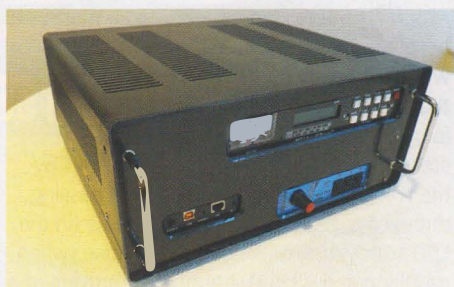
PHOTO 1: Integrated SDR transceiver showing cooling vents and chamfered front panel slots.
