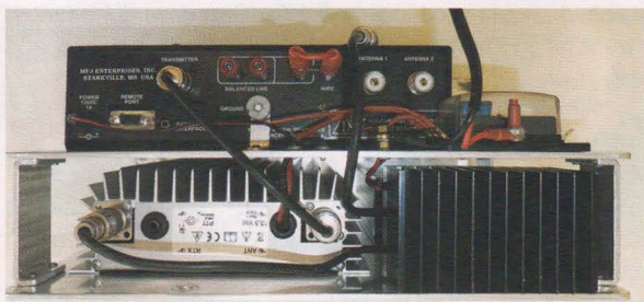
PHOTO 2: Double-decker chassis with ATU, fuse box, dummy load cooling fins and linear amplifier.
