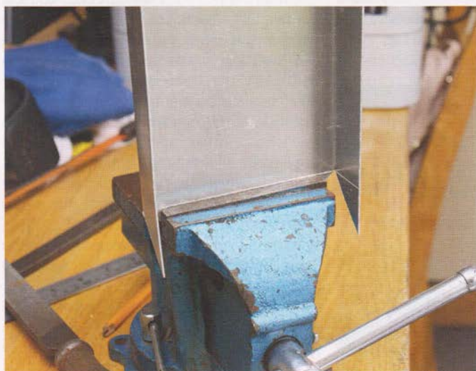
PHOTO 6: Bending sheet aluminium using a vice.
