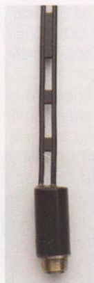
PHOTO 3: Ladder line SO259 termination.
