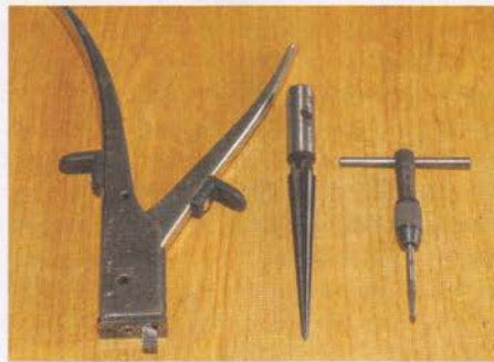
PHOTO 3: Some of my most useful metalworking tools: a nibbler, hand reamer and M3 tap.
