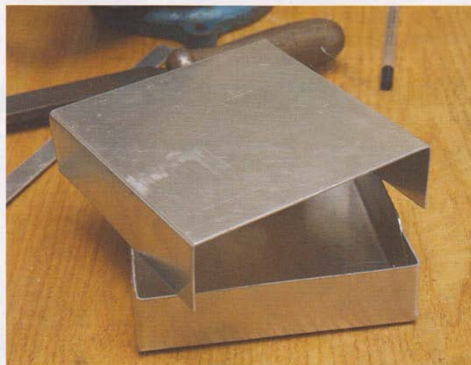
PHOTO 7: The completed box, ready for drilling and painting.
