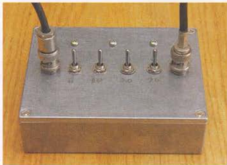
PHOTO 2: The completed attenuator in a diecast aluminium box.
