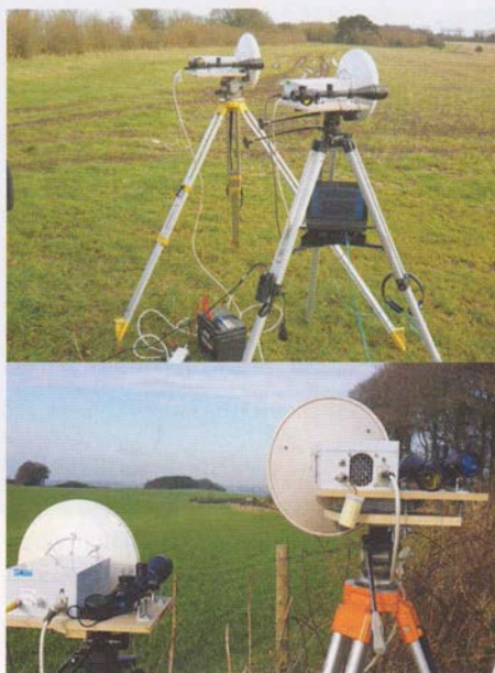
PHOTO 1: The equipment used at each end of the 134GHz record QSO. Photo: G8KQW.
