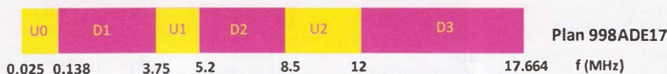
FIGURE 1: VDSL2 downstream and upstream bands alternate and the easiest way to detect VDSL is to look for level changes at the band transitions.
