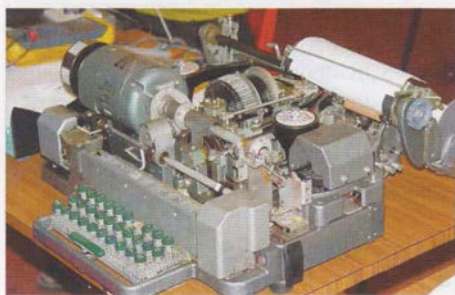
PHOTO 1: A Creed 7B teleprinter. Only a couple of hundred moving parts.
