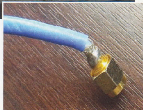
PHOTO 2: Coax braid parting company from an SMA plug.
