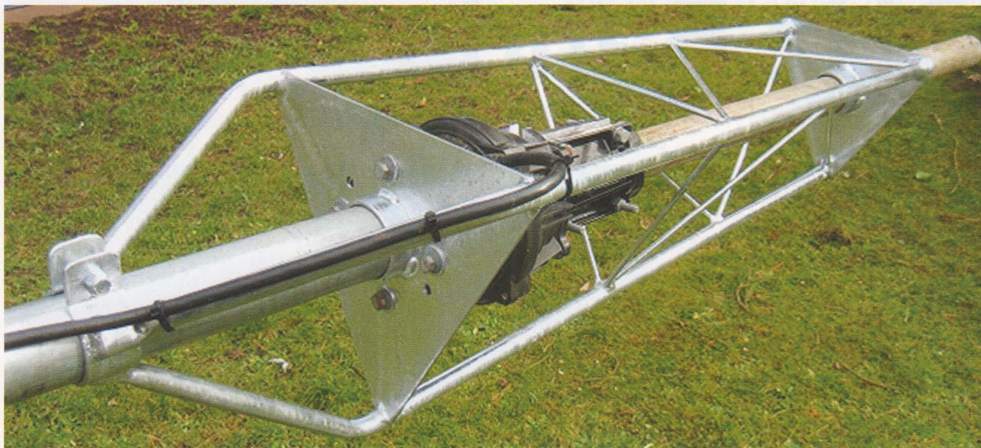
New rotator cage with dual pole entry. Picture courtesy of TennaMast.
