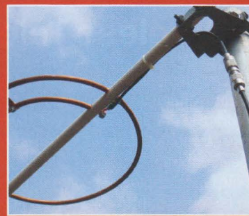
Cover image: A simple halo antenna for the 2m band. Photo: John Adams, G3ZSE.
