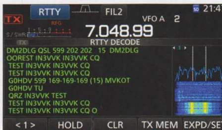
PHOTO 9: RTTY decoder display in expanded mode.
