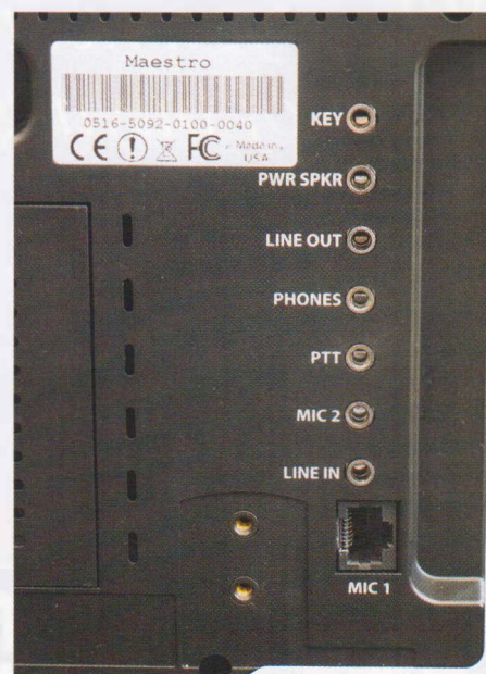
PHOTO 1: The well-connected rear panel of the Maestro.
