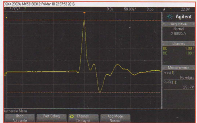
FIGURE 2: Switching spikes injected into the mains by a 50W LED floodlight. The actual spike amplitude is twice as large (see text).
