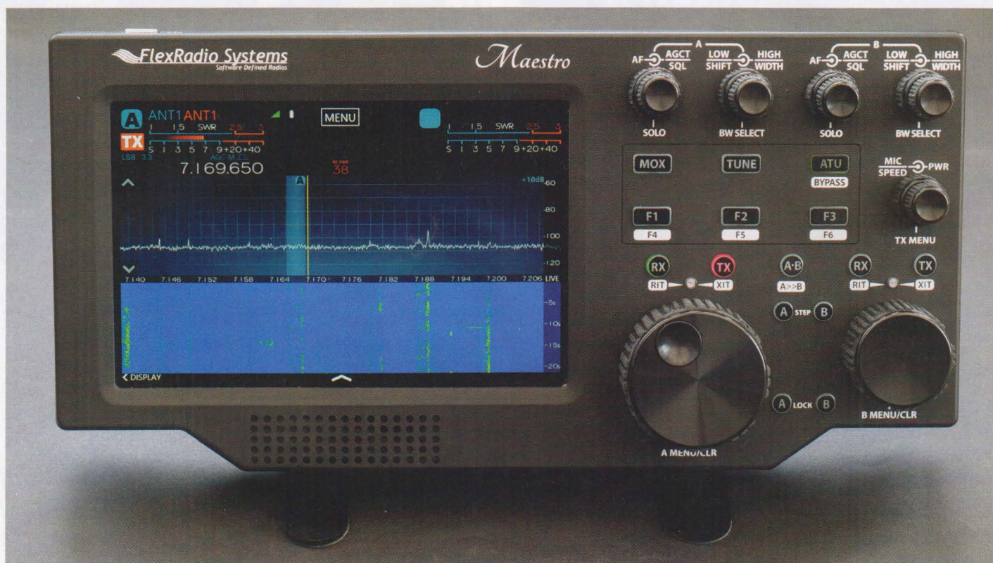
The Maestro is a standalone unit that enables full control of any FLEX-6000 series of transceivers.
