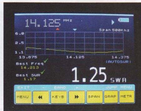
PHOTO 6: The AutoSWR screen for a 20m dipole.
