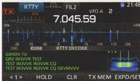
PHOTO 8: RTTY decoder with mini scope display.
