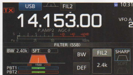
PHOTO 7: Filter bandwidth display.
