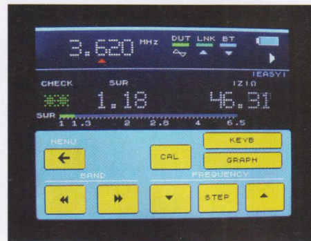
PHOTO 4: A good SWR at 3620kHz.
