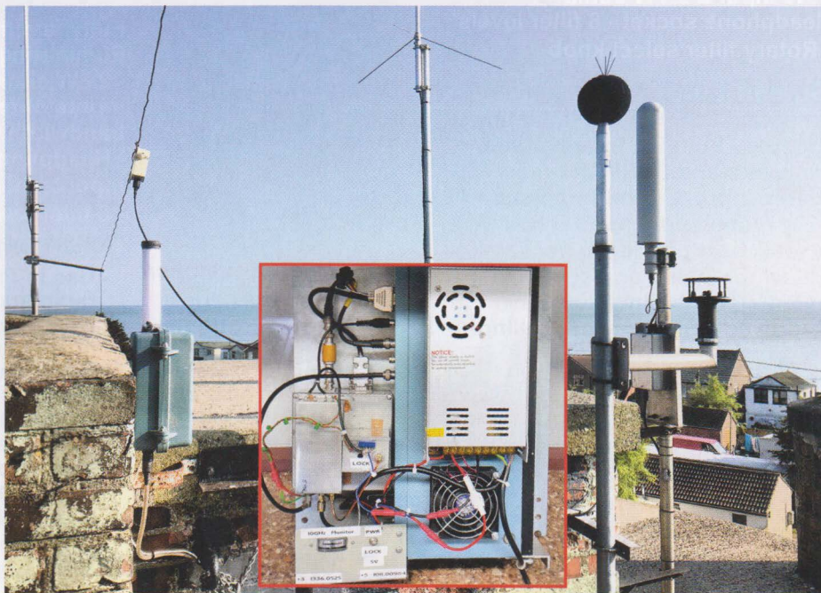
PHOTO 1: The 10 and 24GHz beacons at GB3PKT (blue box on left is 24GHz, long 'radome' on right is 10GHz). Inset: the GB3PKT 10 and 24GHz indoor unit. Photos: GOMBA and G4BAO.
