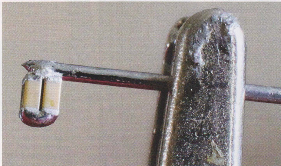
PHOTO 1: Surface mount capacitors paralleled and prepared for soldering to the PCB (see text).
