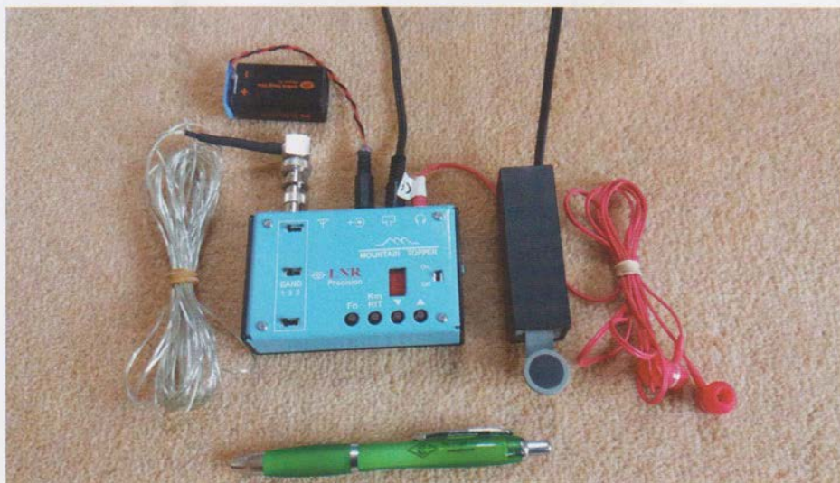
PHOTO 1: An entire station – aerial, power, rig, key and phones – that can easily be carried in your pocket.
