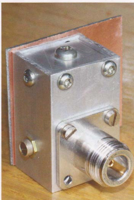
PHOTO 2: General view of the completed 23cm preamplifier. The adjustment screw for C2 is on the left side.
