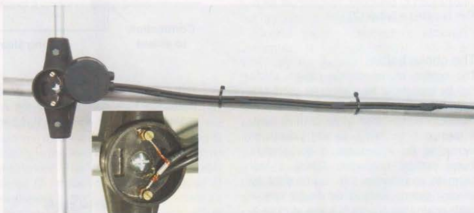
PHOTO 3: \lambda/4 or Pawsey balun used for a 2m antenna and (inset) detail of the connection to the driven element.
