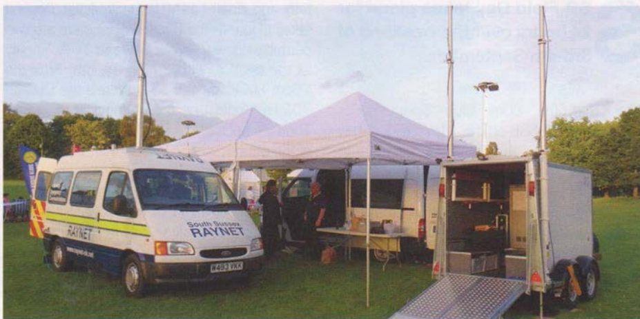
A one-of-a-kind mobile resilience trailer built to bring emergency comms to areas affected by major incidents.
