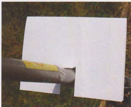
PHOTO 3: White card attached to the aerial to provide a target for the laser rangefinder.
