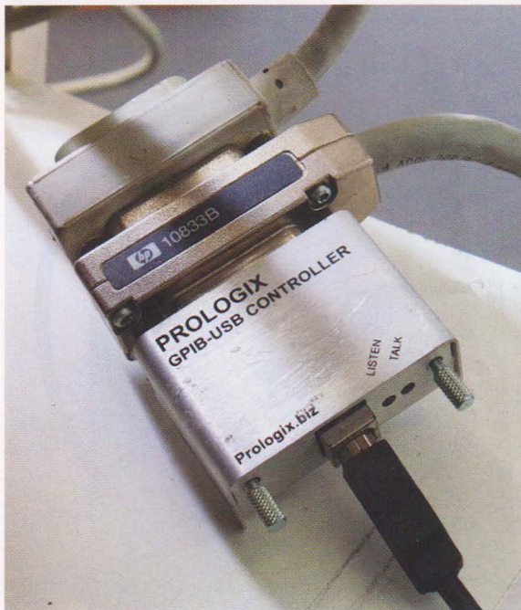
PHOTO 1: General Purpose Instrumentation Bus (GPIB) connectors and Prologix USB/GPIB interface controller.
