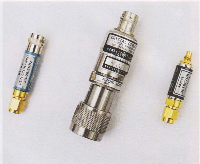
PHOTO 2: Three diode detector heads. The two smaller ones, in spite of different type numbers, are near enough identical internally.
